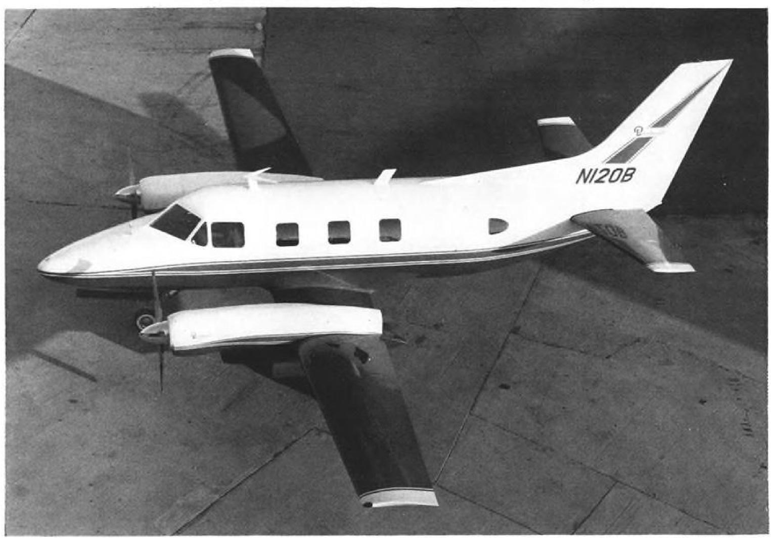
BEECH MODEL 120 turboprop executive transport will be powered by two Turbomeca Bastan 6 engines. Market potential of 500 is seen.
