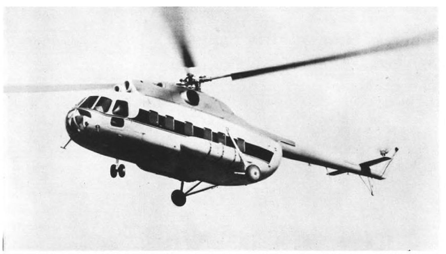
Russian V-8 24-place helicopter, credited to Mikhail Mil's design office, is now powered by paired turboprop engines instead of the single unit of the prototype (AW Feb. 12, p. 65). Wheel pants have been removed from this version.
