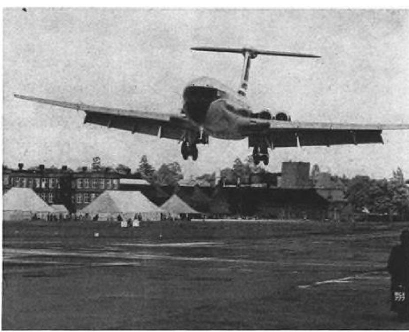
Vickers VC.10 transport makes final approach (right to left) after flight at Farnborough. Fowler-flap sections and leading edge slats
