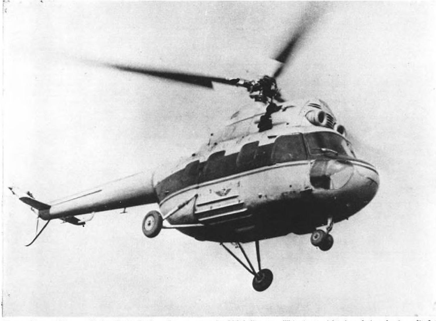
Two small gas turbines, credited to Soviet Designer Isotov, power the V-2 helicopter. This six- to eight-place design also is credited to Mil's office and apparently is a conversion of the piston-engined Mi-1 to turbine power.
