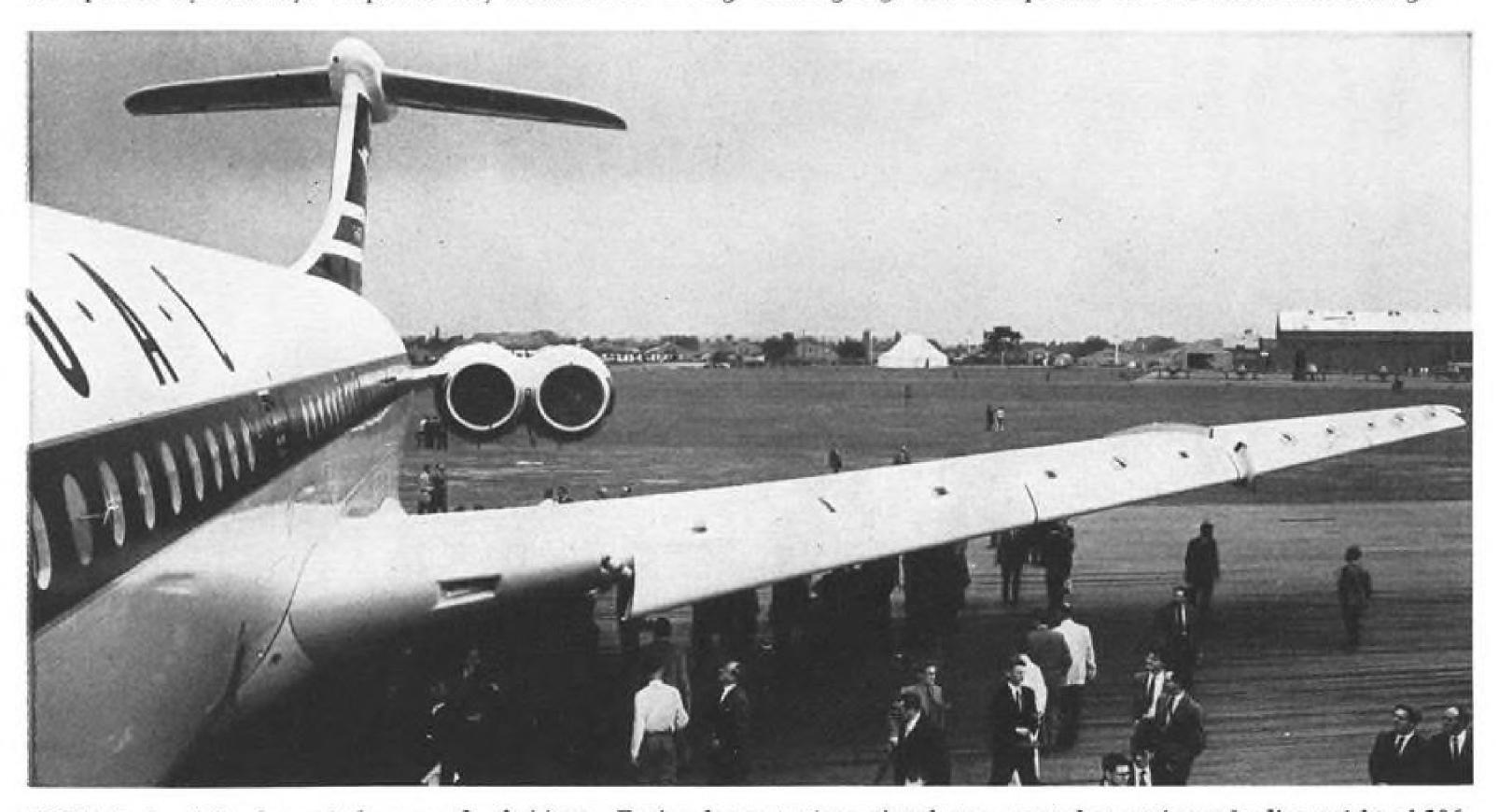
VC.10 display at Farnborough drew crowds of visitors. During demonstrations, aircraft was operated at maximum landing weight of 206,-000 lb. Maximum takeoff weight is 310,000 lb. Original VC.10 model and stretched version, Super VC.10, have 4,000-mi. ranges. Vickers also plans a third model with 6,000-mi. range. The company currently is attempting to determine the feasibility of the VC.10 transport for London-Los Angeles service.
