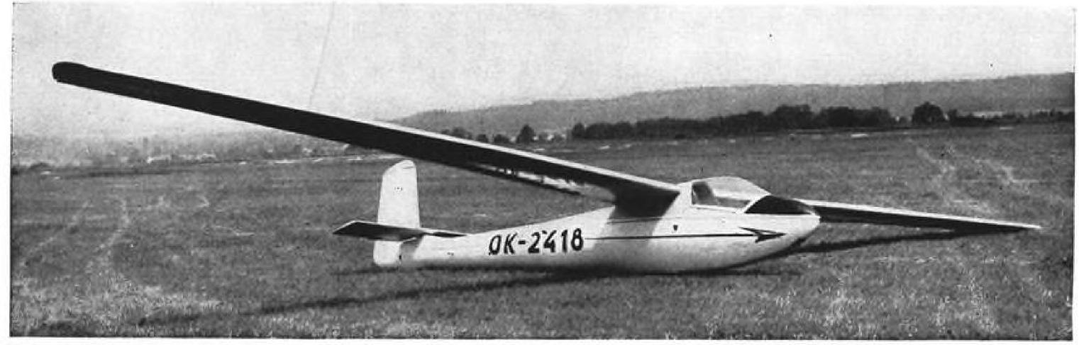
SPAN OF THE NEW ORLIK VT-16 sailplane is 52.5 ft.; length is 24.7 ft., height 5.2 ft., wing area of the sailplane is 138 sq. ft.
