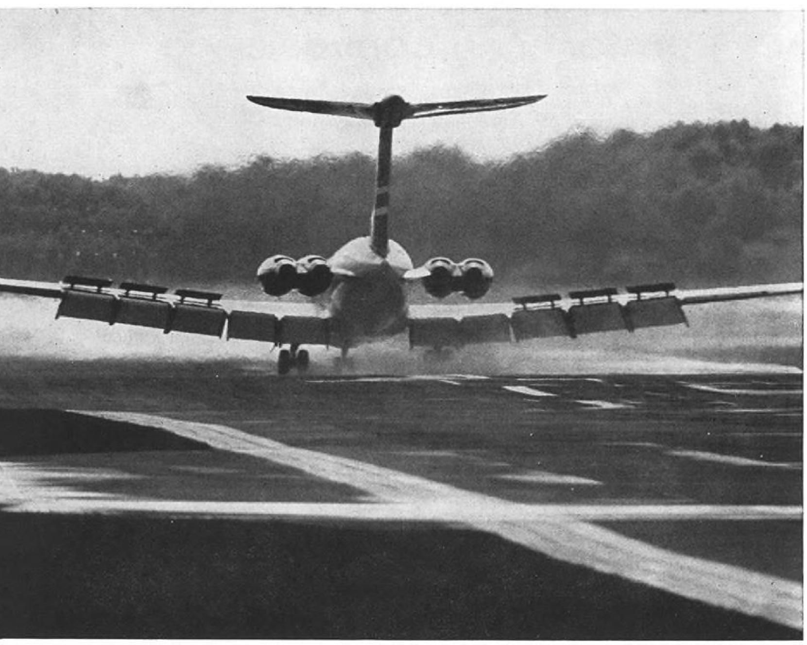
Three spoilers installed in each wing assist in braking the VC.10. During the Farnborough flights (AW Sept. 10, p. 26), made with the first production model, pilot actuated thrust reversers immediately prior to touchdown. VC.10 has completed 44 flights, totaling 56 hr. 50 min. Highest takeoff weight has been 250,000 lb.; top speed reached was Mach .84 at 35,000 ft.
