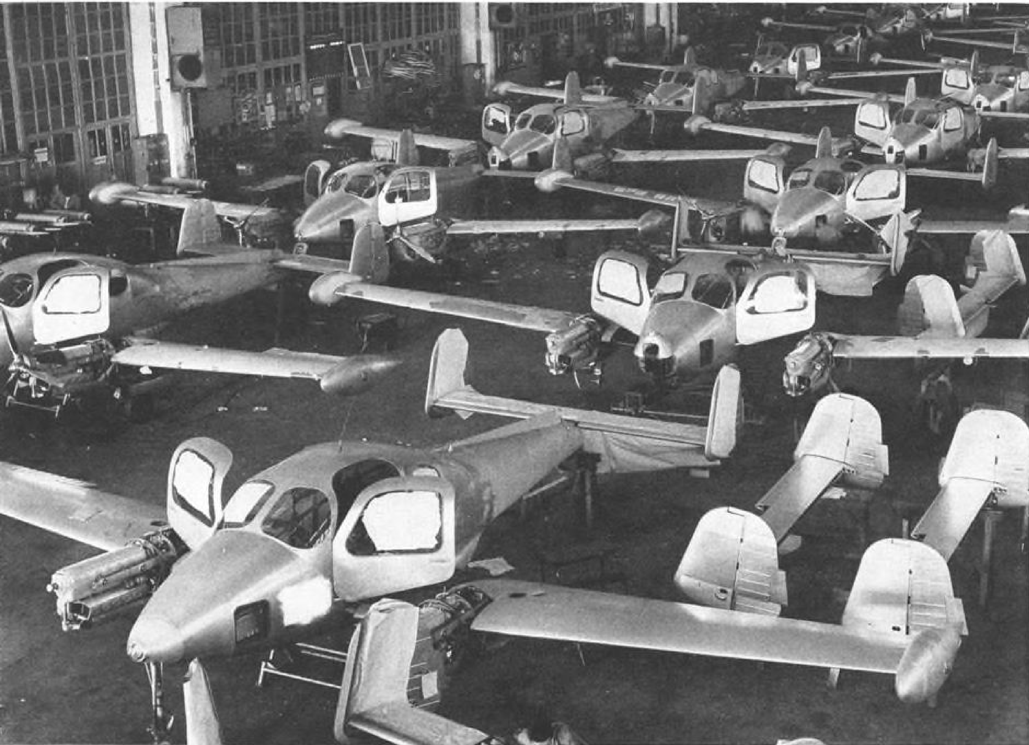
SIXTEEN CZECHOSLOVAKIAN MORAVA 200D executive twins move down the production line at the National Aircraft Works in Kunovice. Fuselage is all-metal semi-monocoque structure. Aircraft is certificated under CAR Part 3 (Category N).
