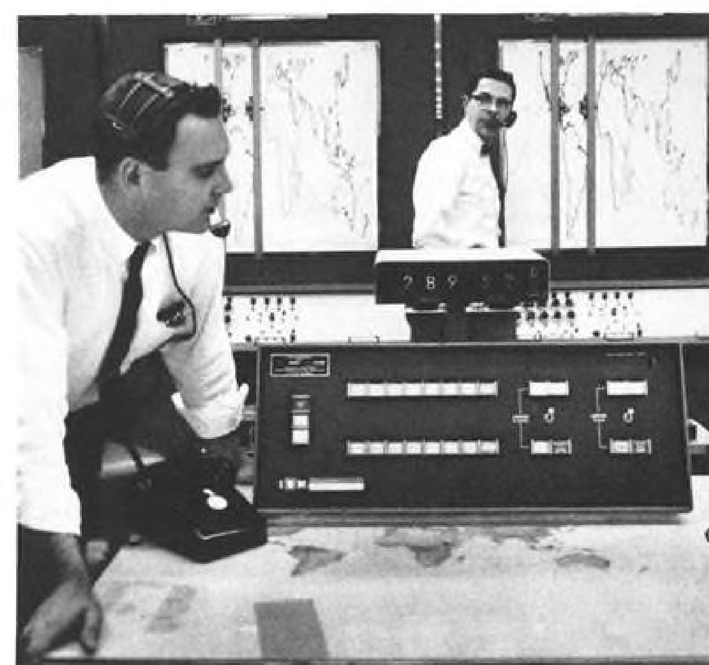
This plotting board, driven by an IBM computer, tells PROJECT MERCURY control personnel the exact location of the MERCURY spacecraft at any time in its orbit.
