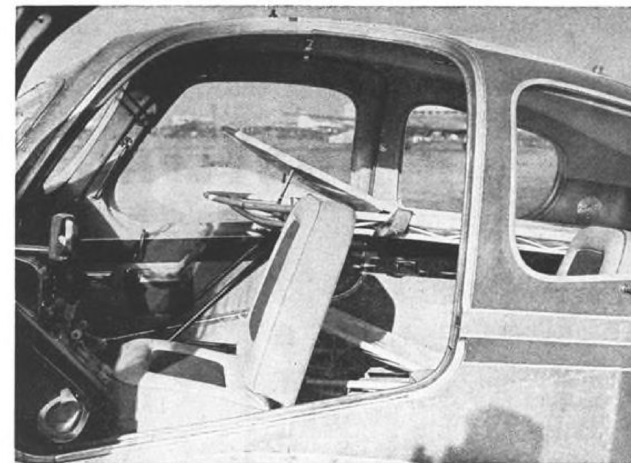
MORAVA 200D equipped for air ambulance service contains two stretchers and a seat for flight attendant. CSA, Czech airline, has a number of this type in operation. Baggage compartment is behind rear seat in passenger version.
