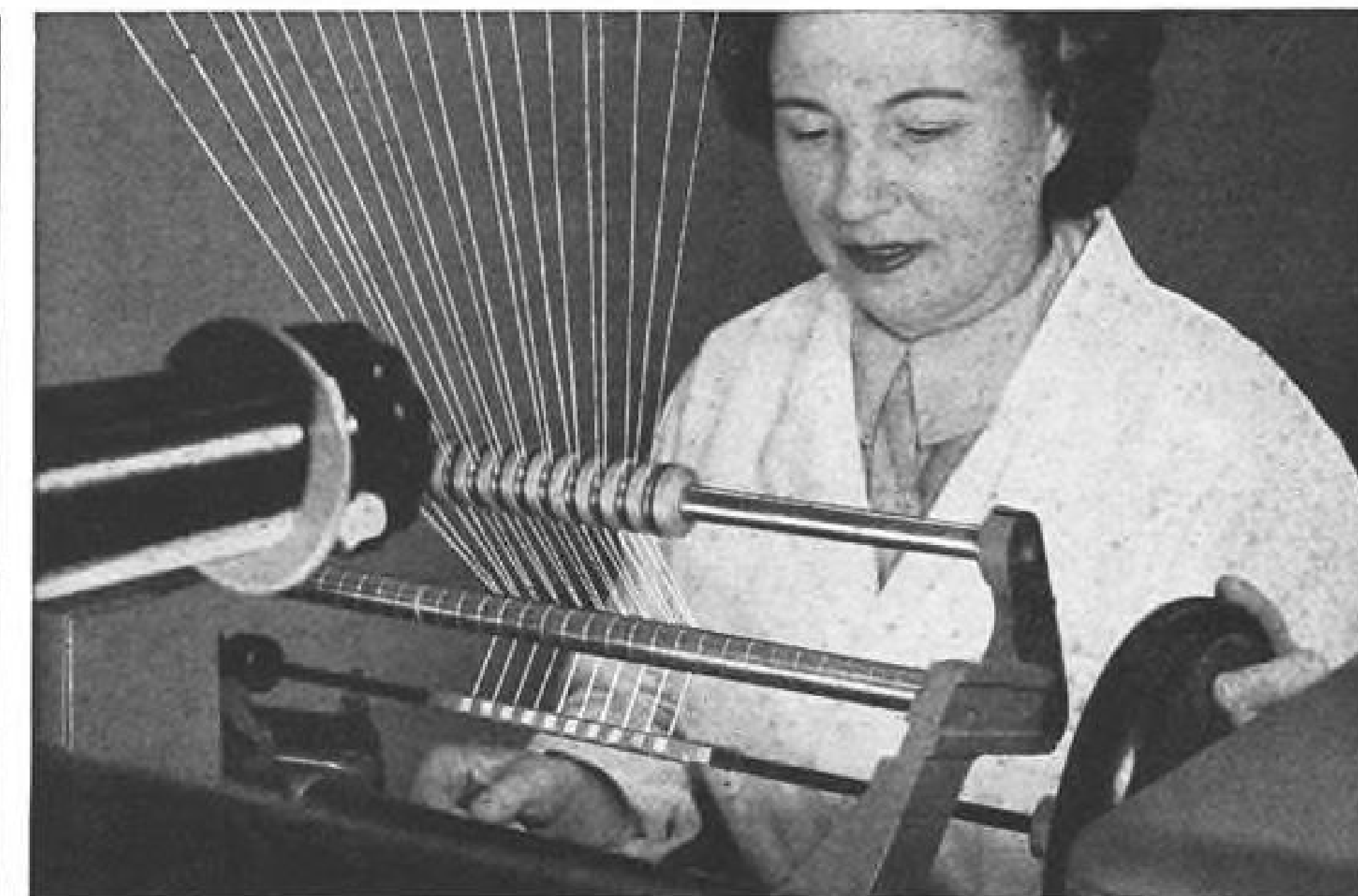
Multiple winding of coils is one of the procedures used by Wheeler in its unprecedented facility for the continuous production of high reliability transformers.
