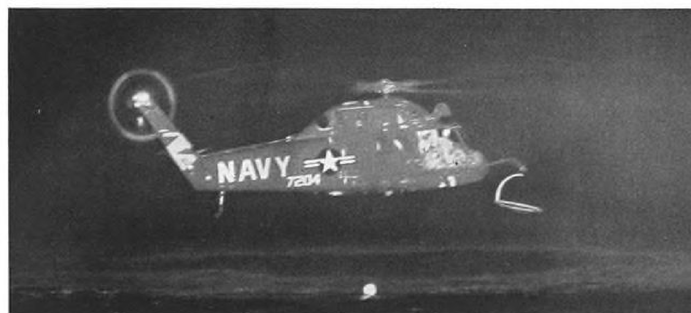
Helicopter open sea rescue equipment, developed by Kaman Aircraft under a $109,000 Navy contract, successfully makes a simulated rescue at night in moderately heavy seas about five miles off Block Island, N. Y. Waves were about five feet high as helicopter moved in toward test subject. Kaman engineer in water supposedly was immobile and unable to help himself. Above, left, is pilot's view of engineer in landing lights. Right, pilot swings ladle-like rescue net out on movable arm.
