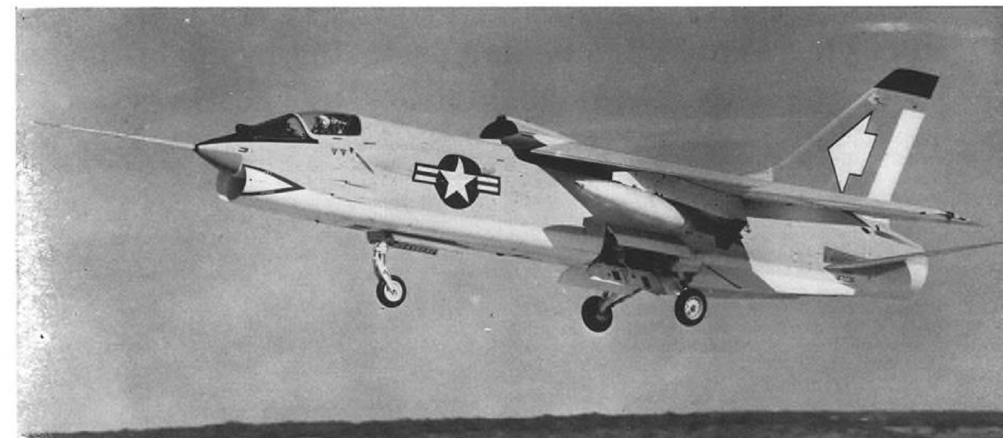
Crusader lands at Chance Vought's Grand Prairie, Tex., facility carrying two 2,000-lb. bombs, mounted on pylons under each wing.
