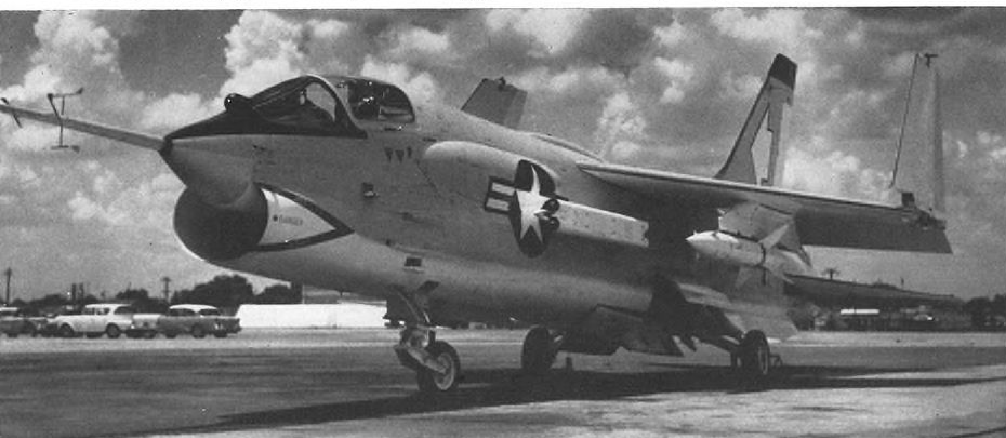
Above, F8U, which has maximum speed of approximately Mach 2, carries 30 Zuni rockets in wing pods. In flight tests, flames from salvo-fired Zunis extended far enough to scorch plane's horizontal tail surfaces, may necessitate fabricating them of stainless steel. Below, aircraft armed with Bullpups and Zunis is parked with wingtips folded in carrier-stowage configuration.
