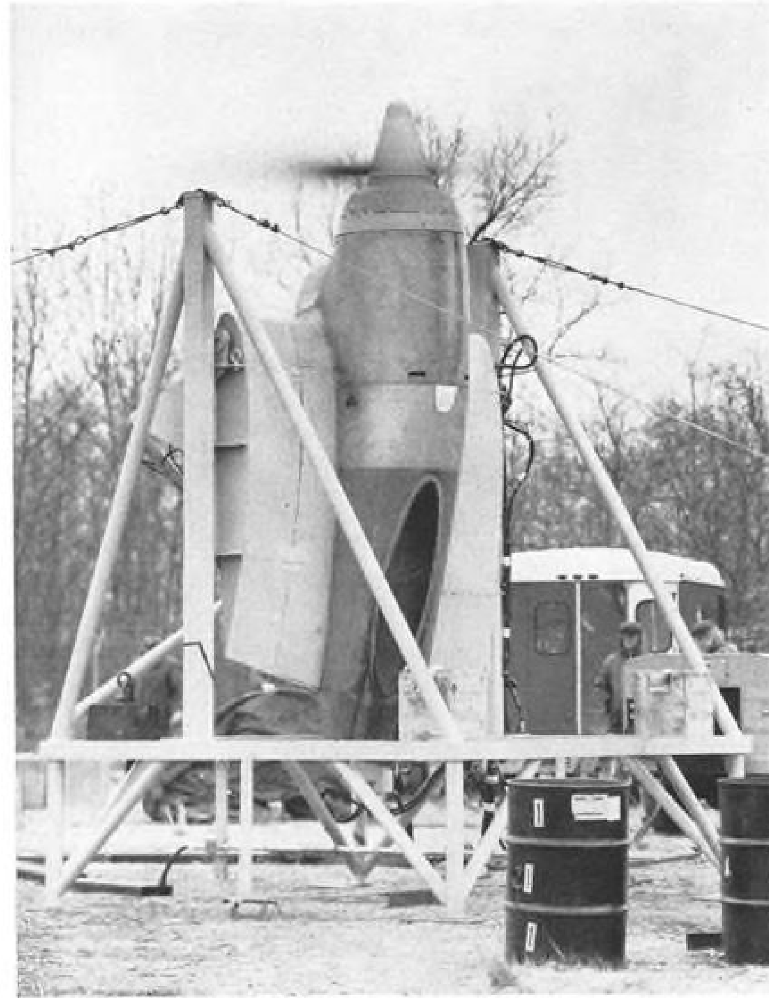
PRODUCTION LINE FOR T53 turboshaft engines is shown from overhead, above left. Right, vertical test stand with operating T53 is used to check characteristics of powerplant through typical VTOL operations. Wing can be pivoted during engine run.
