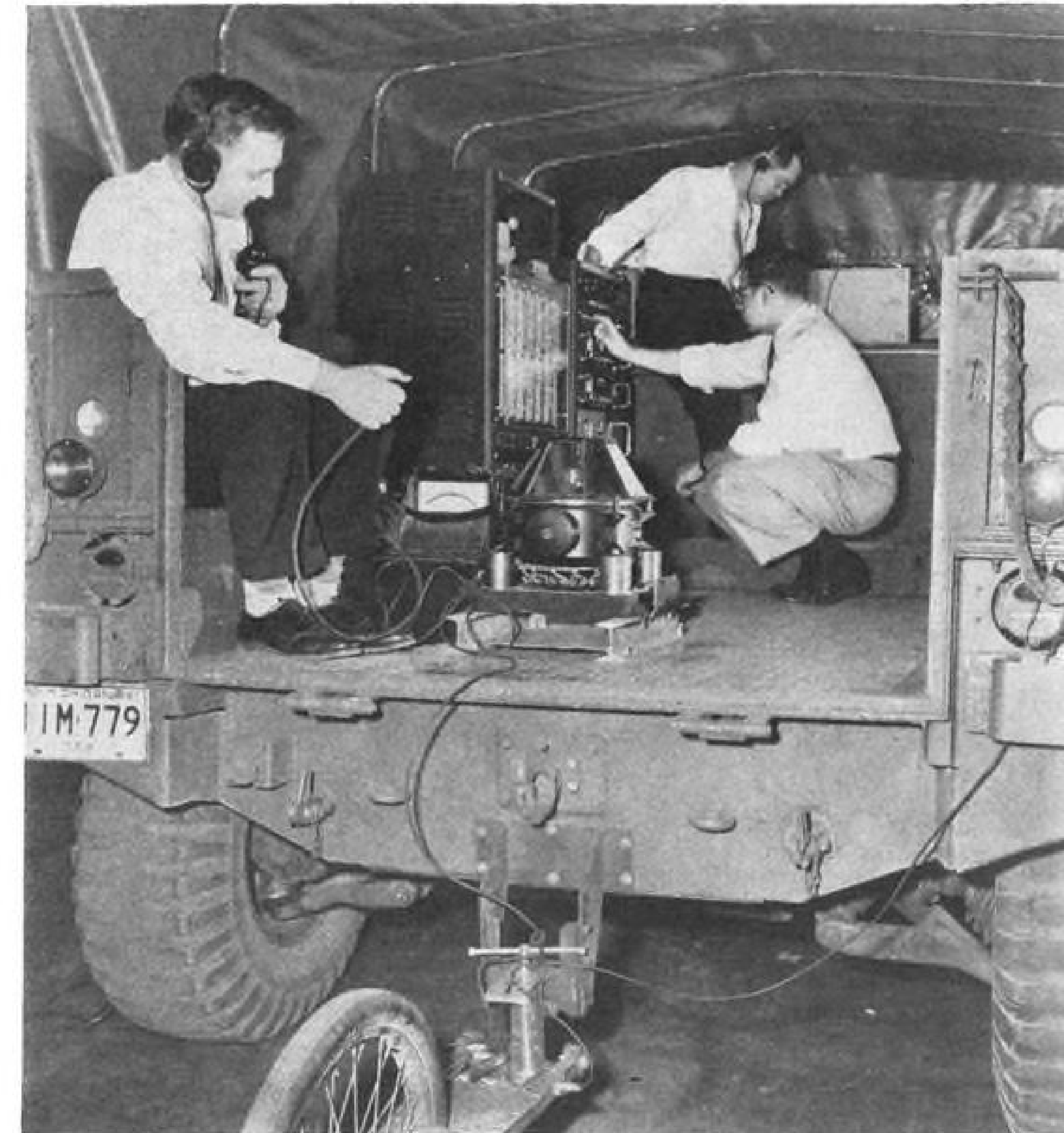
NAVIGATION SYSTEM for an MMRBM missile transporter-launcher, using a fifth-wheel type odometer in combination with a gyro-stabilized platform to measure vehicle tilt angle, reported by General Precision engineers, is based on earlier tests conducted by company and Chrysler Corporation engineers, shown in photo above.
