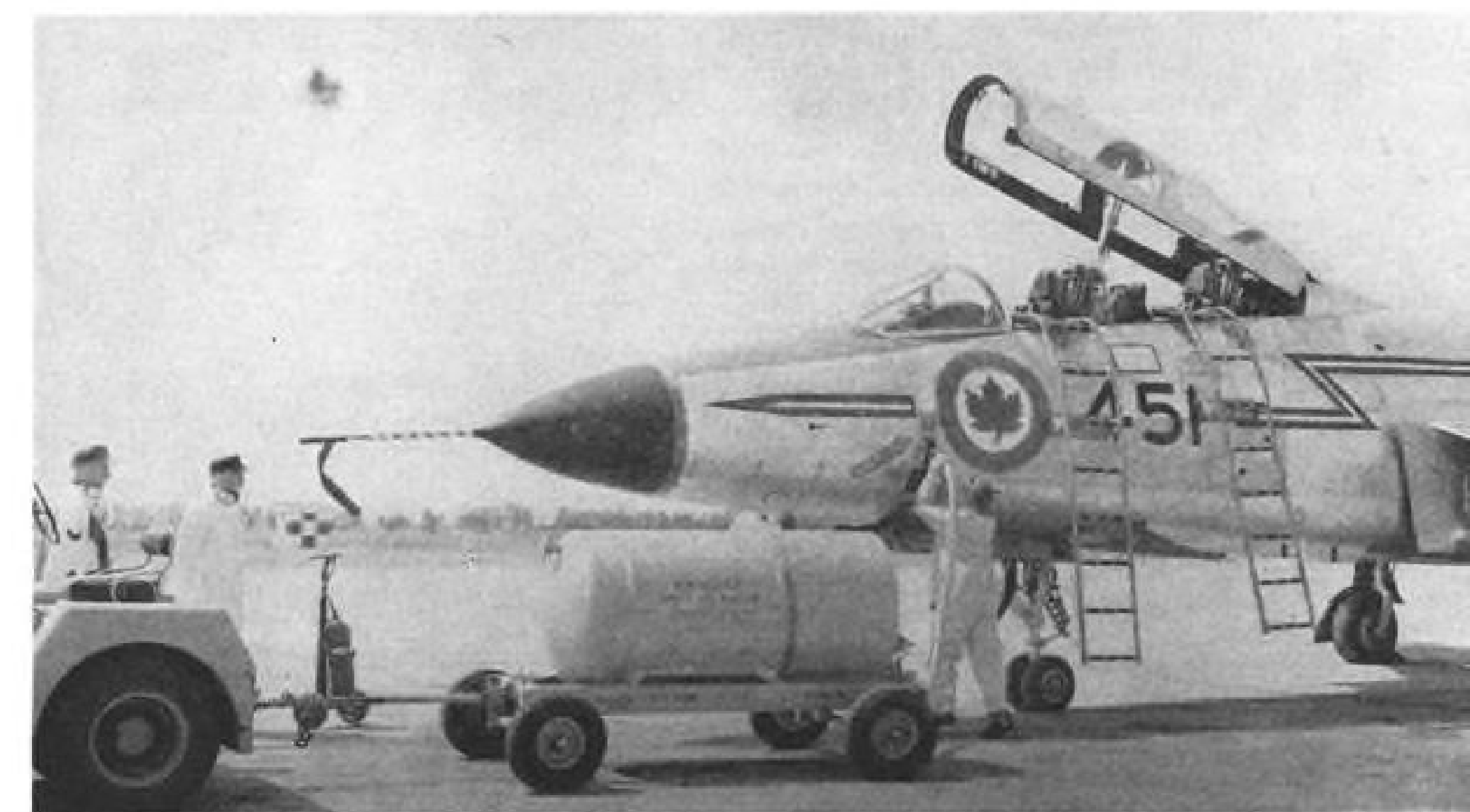
Ground personnel stand away from CF-101B, above, as safety precaution during liquid oxygen fueling. Drag chute landing is shown below.
