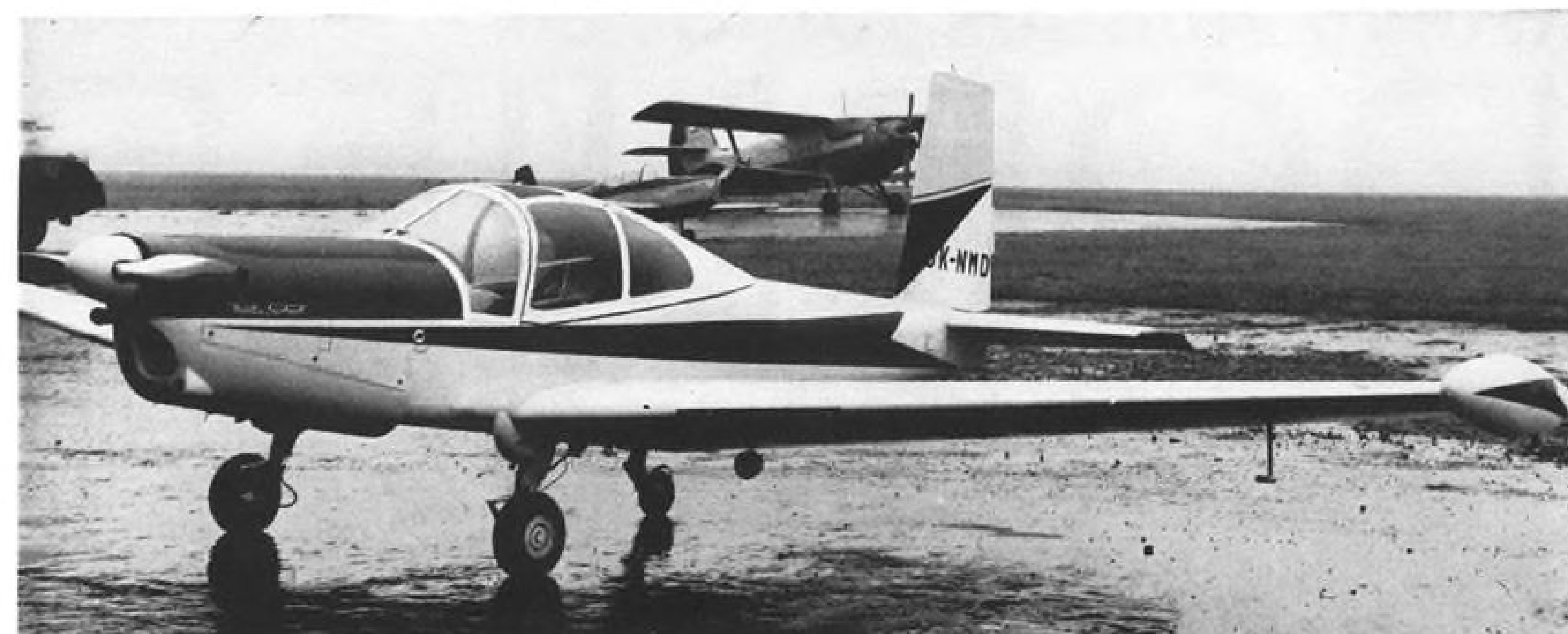
CZECHOSLOVAKIA'S L-40 META SOKOL business plane is fitted with a supercharged 140-hp. engine and features a reverse tricycle landing gear. Price of the airplane, delivered in the United Kingdom, is $12,880 duty paid. Note Czech An-2 in background.
