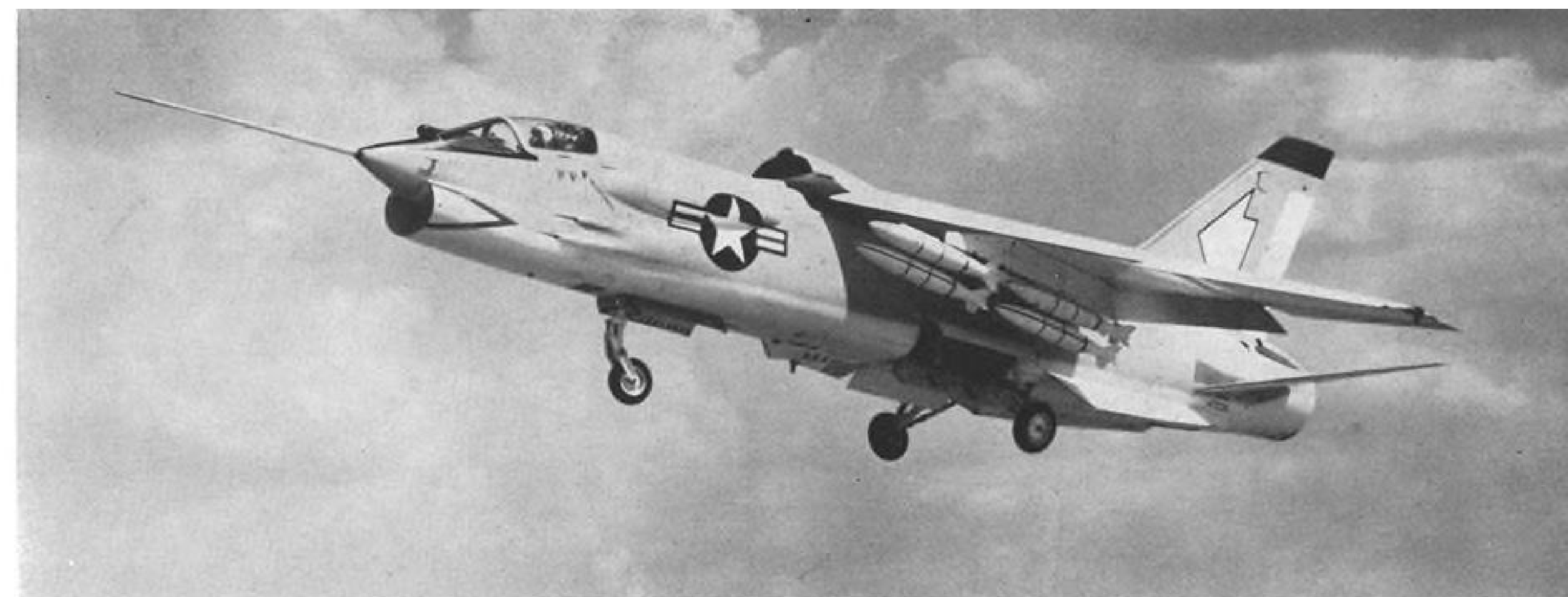
Crusader, powered by Pratt & Whitney J57-P-20 engine producing 18,000 lb. thrust, flares out for landing after flight with four 500-lb. bombs mounted on multi-purpose pylons under each wing. Note that two-position wing has been raised for carrier-type landing.
