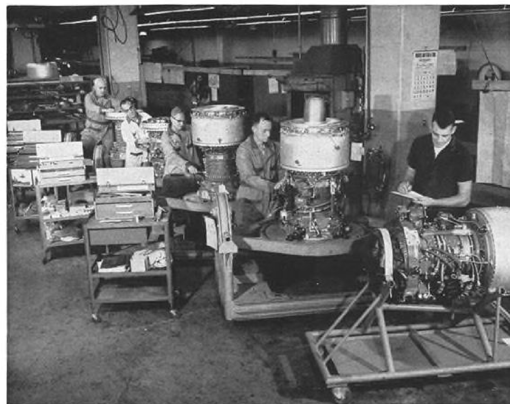
LYCOMING T55 ENGINES are assembled on this small line before being run and accepted. Rotatable holding fixtures are used for convenience.
