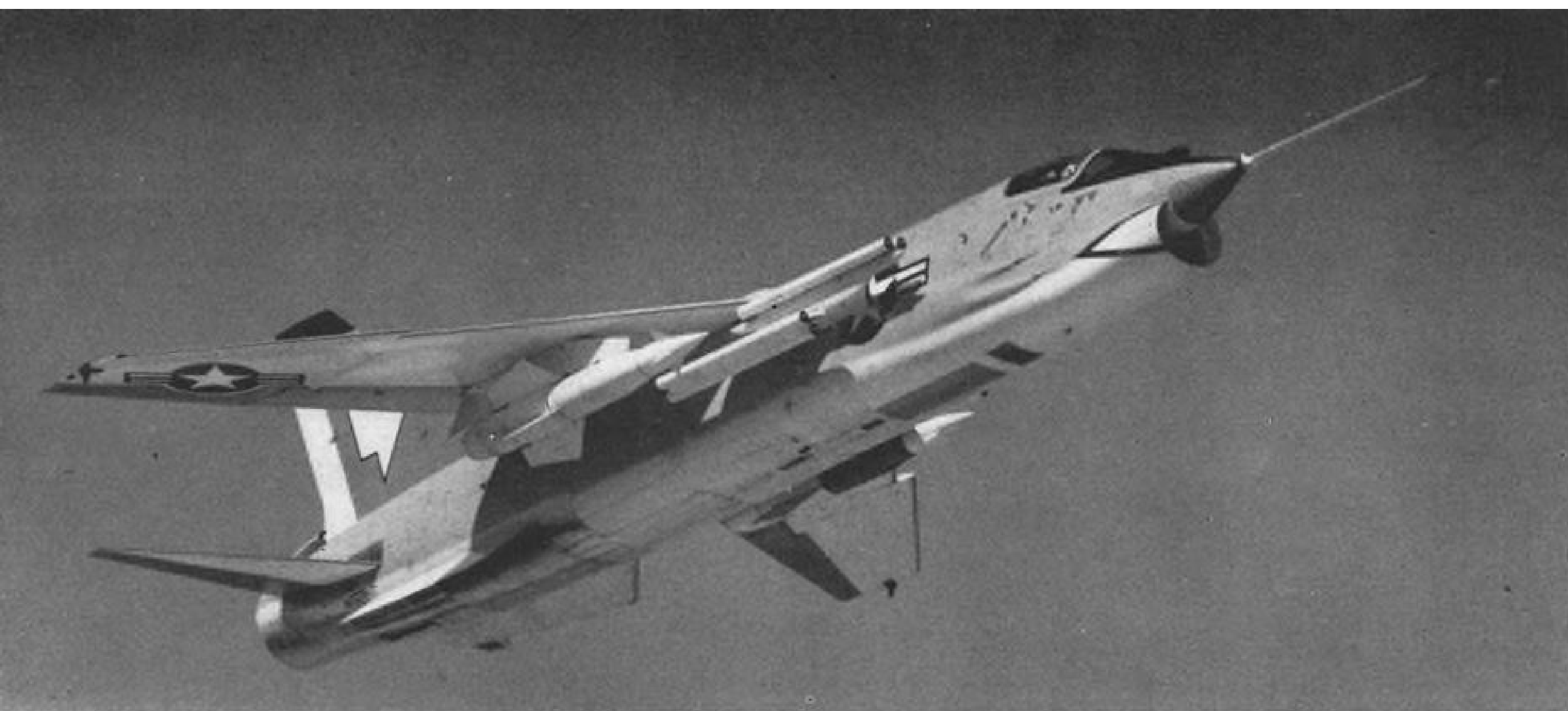
Navy is evaluating Chance Vought's F8U-2NE Crusader jet fighter for use as a strike aircraft. Above, the single-jet fighter is shown on an evaluation flight armed with two Bullpup B air-to-surface missiles and eight Zuni all-weather rockets carried in pods.
