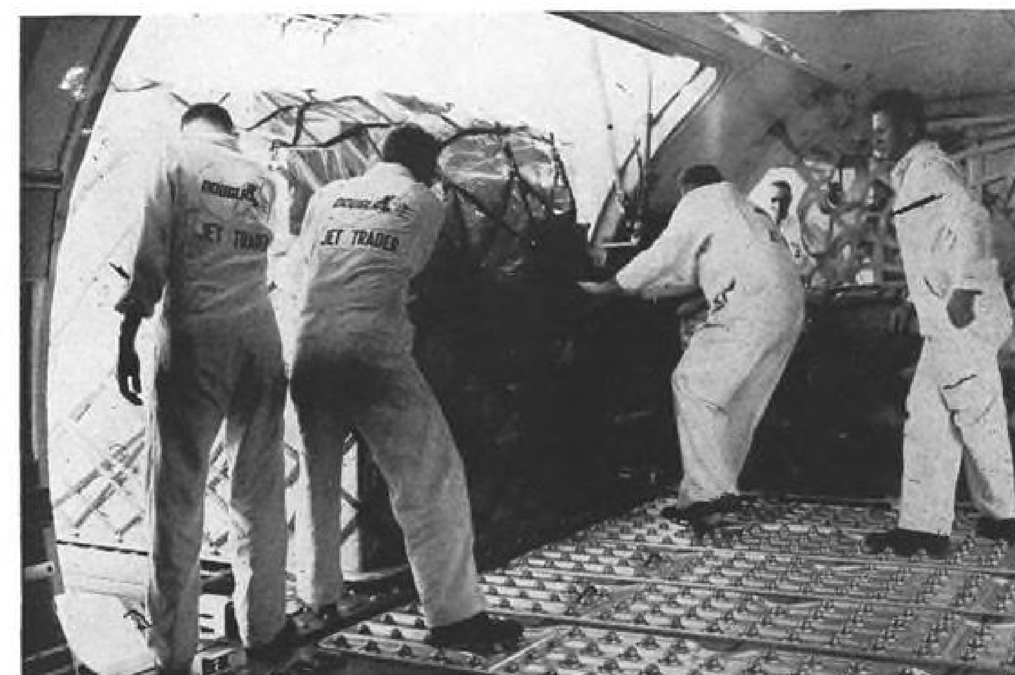
SPRING LOADED BALL BEARING rollers in the Douglas DC-8F facilitate easy movement of pallets. Mechanism is compatible with the military 463L system.
