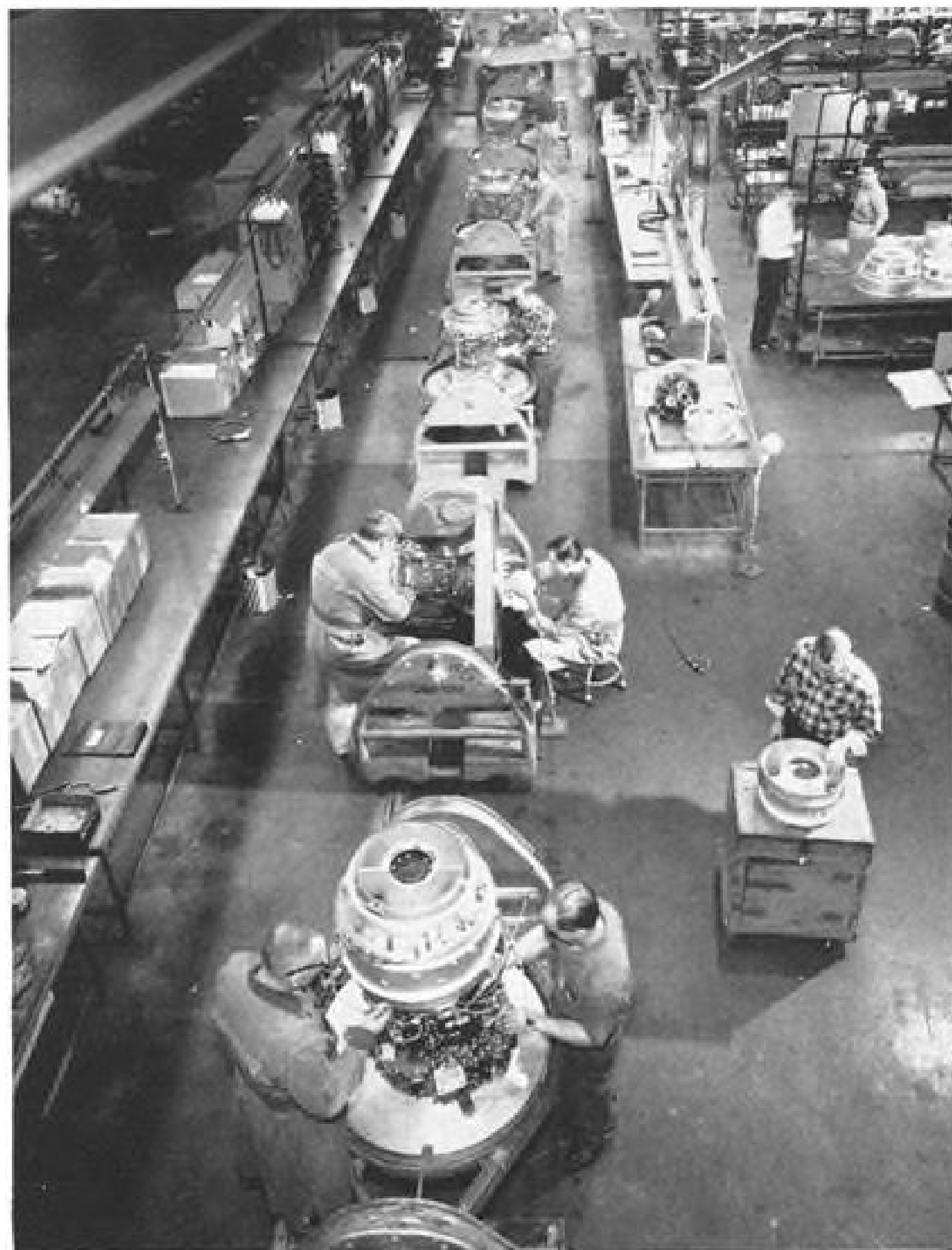
PRODUCTION LINE FOR T53 turboshaft engines is shown from overhead, above left. Right, vertical test stand with operating T53 is used to check characteristics of powerplant through typical VTOL operations. Wing can be pivoted during engine run.
