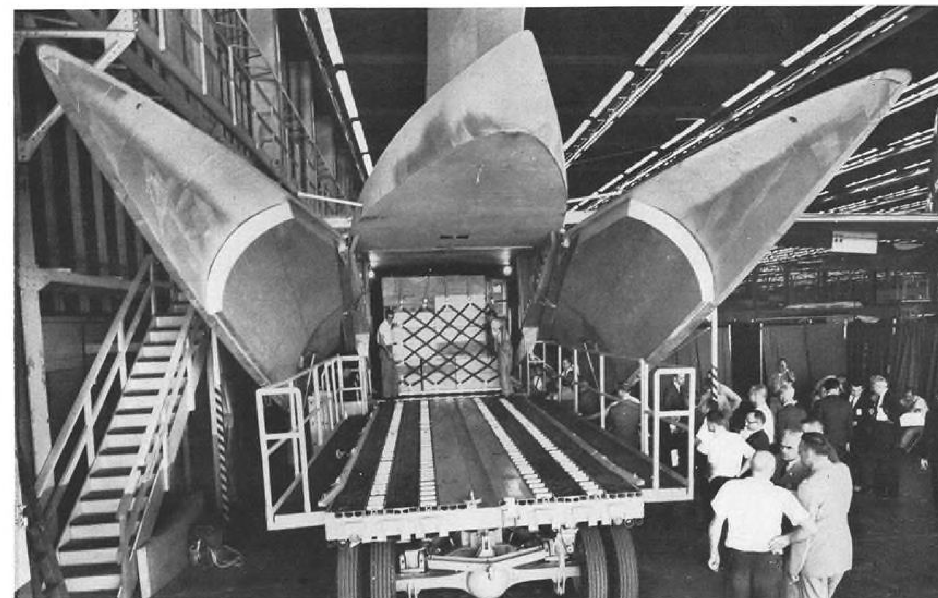
CARGO LOADER DEVELOPED for USAF 463L is demonstrated on wood mockup of Lockheed's C-141 at Marietta, Ga.
