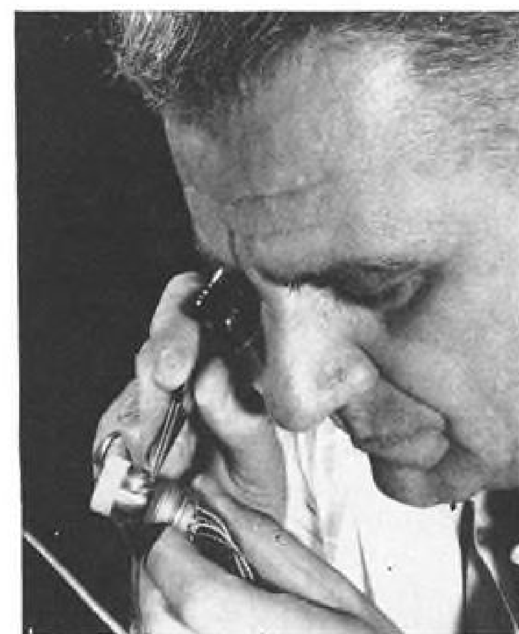
Precision engineering of Raytheon gyroscopes for guided missiles include a vibration-dampening silicone fluid that retains its fluidity below -55°F.
