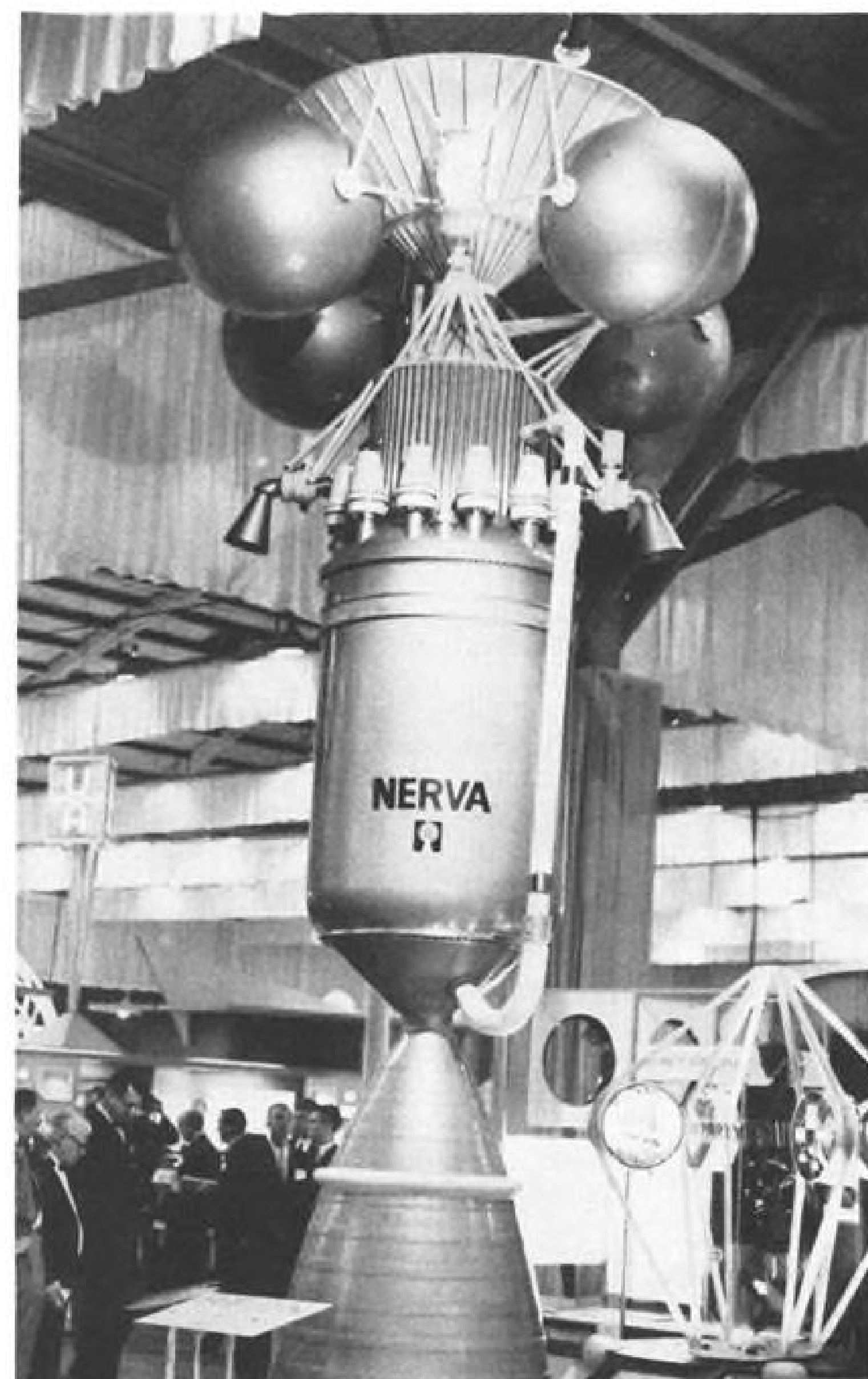
Quarter-scale Nerva mockup (below, left), exhibited by Aerojet-General Corp., indicates the size of the final unit planned for upper stage testing in the Rift vehicle. Martin Pegasus (below, right), a three- or two-stage high-altitude probe developed from the company's Pershing missile program, is detailed in this cutaway model. First details of the Pegasus were revealed in Aviation Week (AW Nov. 19, p. 27).
