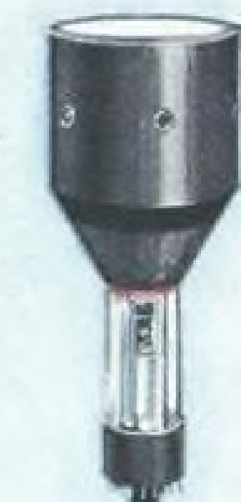
RCA Display Storage Tube —similar in principle to your home TV picture tube—paints a picture of electronic signals in radar systems and industrial test instruments.
