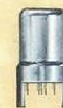
RCA Nuvistor Tube shown here actual size— improves performance of numerous electronic devices ranging from space satellites to home TV receivers.
