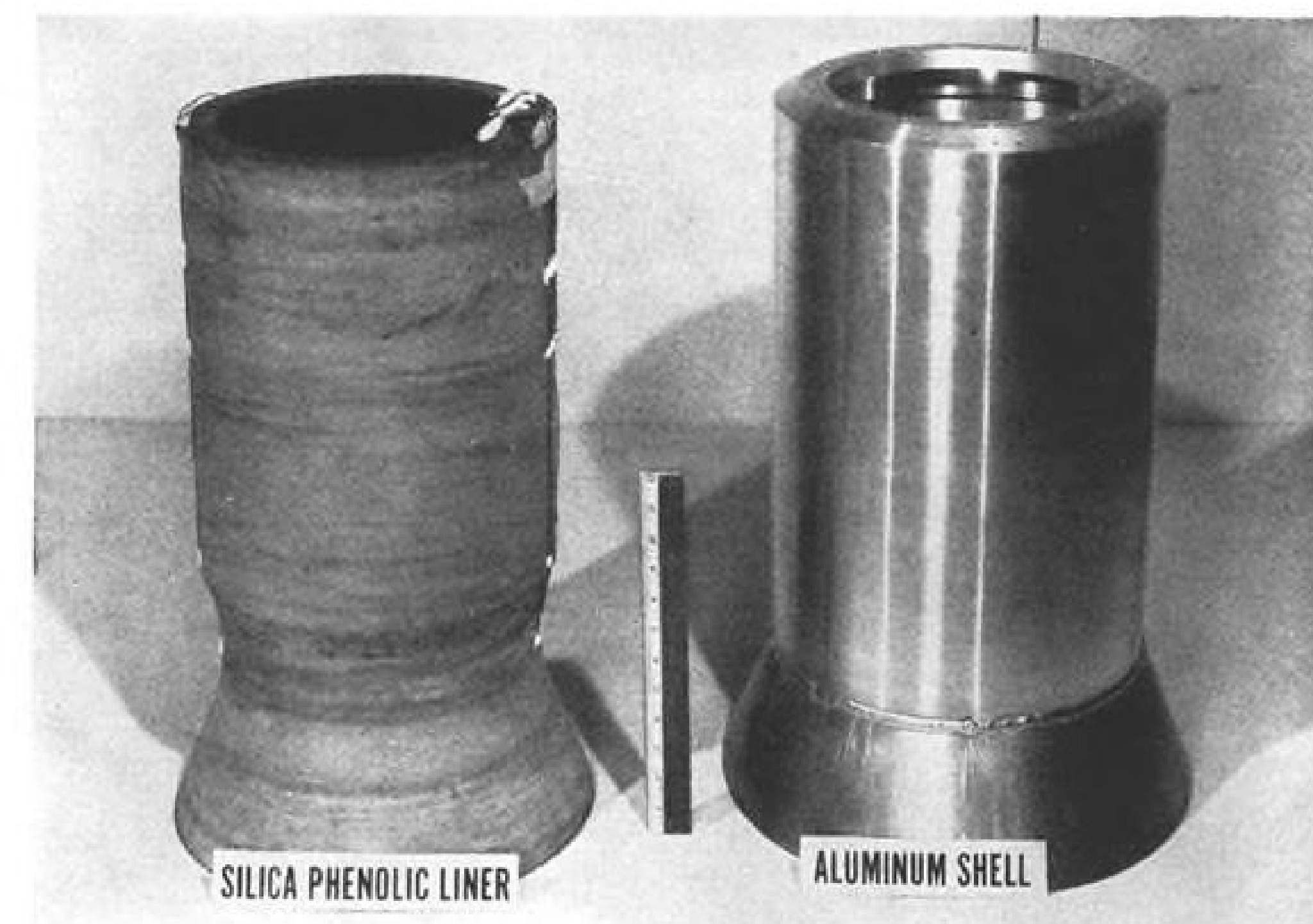
ABLATIVE LINER (left) of the TD-321 engine is fabricated from preferentially wrapped, phenolic-impregnated silica cloth. Plastic insulation layer, called Ablatalite, is pour-molded between it and the aluminum shell. Engine developed 5,300 lb. thrust in recent test firings.
