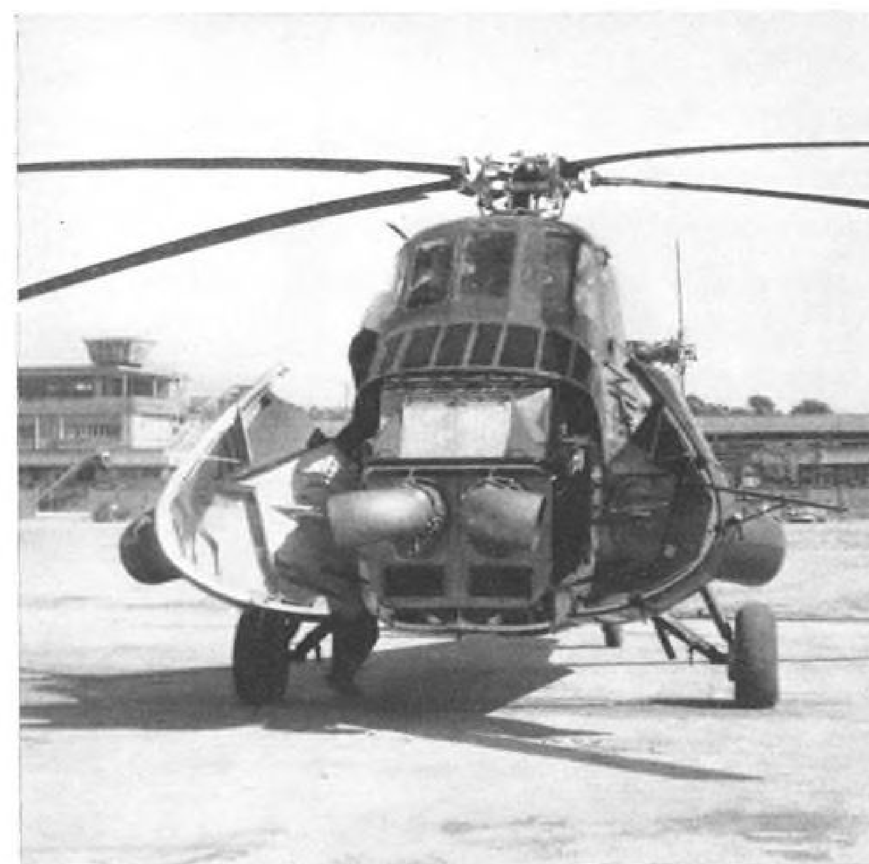
Empty weight of the helicopter is 8,000 lb. and gross weight is 13,266 lb. Sud's twin Bastan H-34 first flew in early October. Company assembled 92 S-58s purchased by the French government, then built 185 under license, including five for Belgium.
