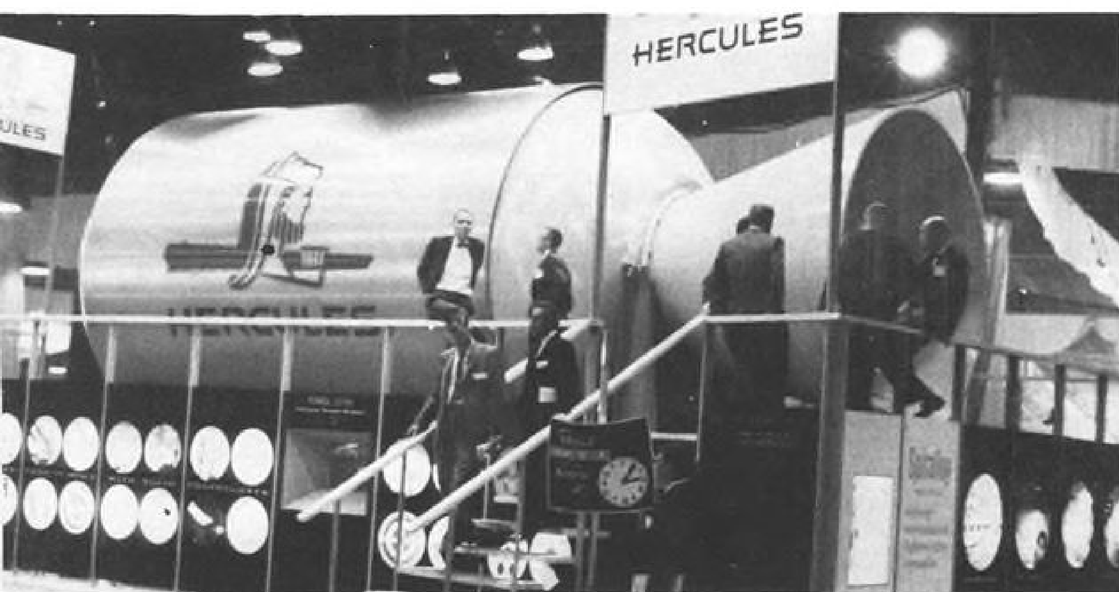
Hercules Powder Co. used a filament-wound casing (above, left) for a 156-in. dia. solid for its technical display at the 17th annual meeting of the American Rocket Society in Los Angeles (AW Nov. 19, p. 27). Subliming solid salt is the fuel for microrocket engine (above right) developed by Rocket Research Corp. Throat diameter is 0.01 in.; thrust is about one-ten thousandth lb.
