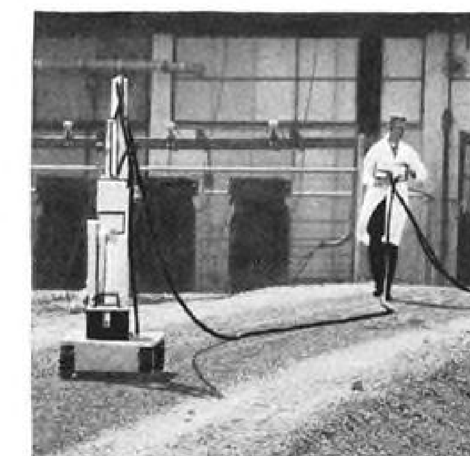
ROCKET ROBOT. Remotely controlled device carries experimental motors and "hot" propellant compounds from lab to test area. Speeds developmental work.
