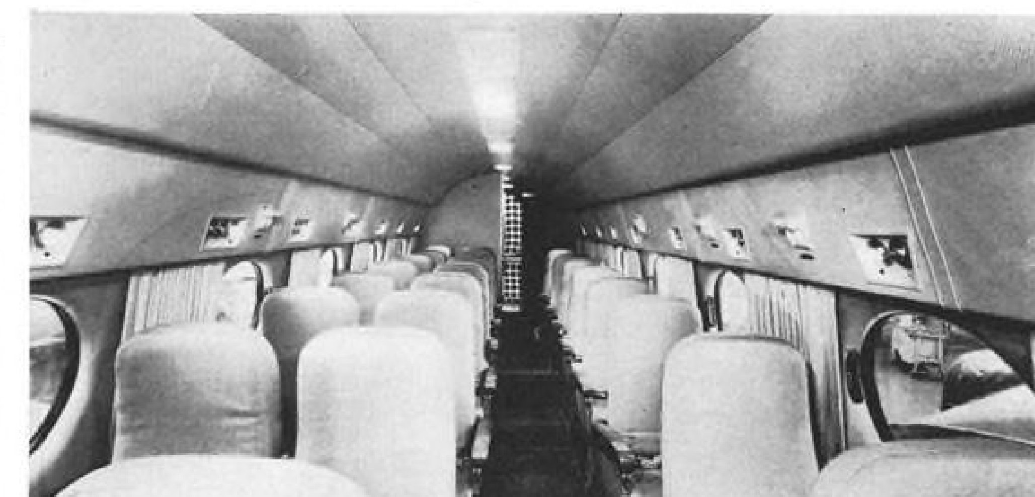
Seats in the 24-passenger Gulfstream have 33-in. pitch and are separated by a 16-in. aisle. The five-rail track system in the floor allows the seats to be removed from the aircraft cabin and cargo tie-downs to be substituted rapidly.
