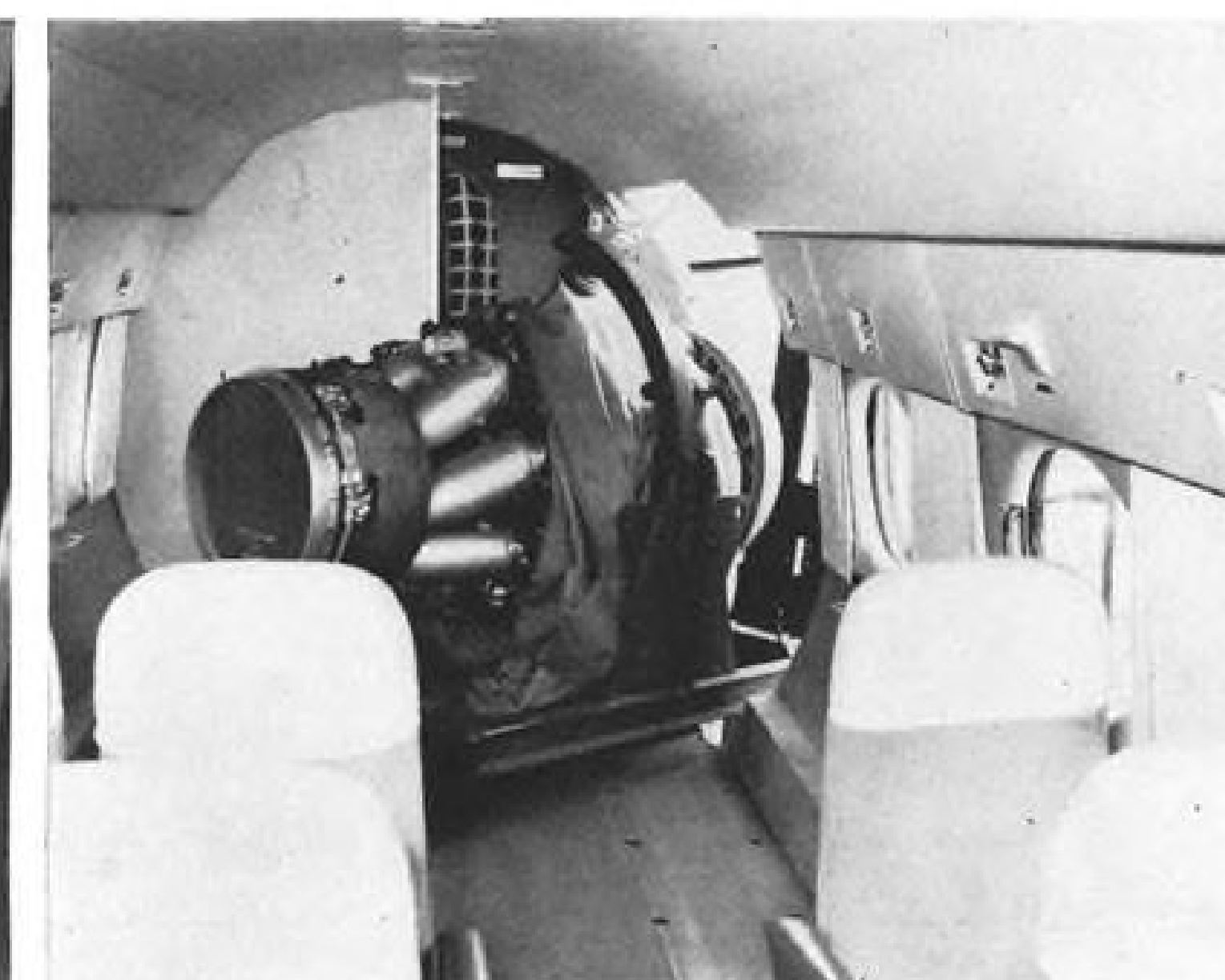
Cargo/passenger mix is shown above left with cargo at rear of cabin. Right, Rolls-Royce Dart engine is loaded aboard aircraft which still has 12 seats in place in 1,200 cu. ft. cabin. Seats can be stowed aboard aircraft after removal from cabin.
