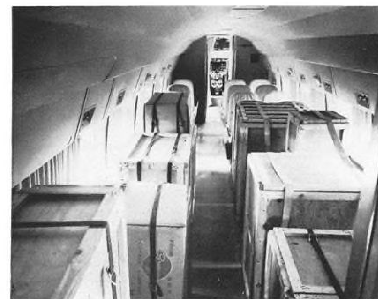
Cargo/passenger mix is shown above left with cargo at rear of cabin. Right, Rolls-Royce Dart engine is loaded aboard aircraft which still has 12 seats in place in 1,200 cu. ft. cabin. Seats can be stowed aboard aircraft after removal from cabin.
