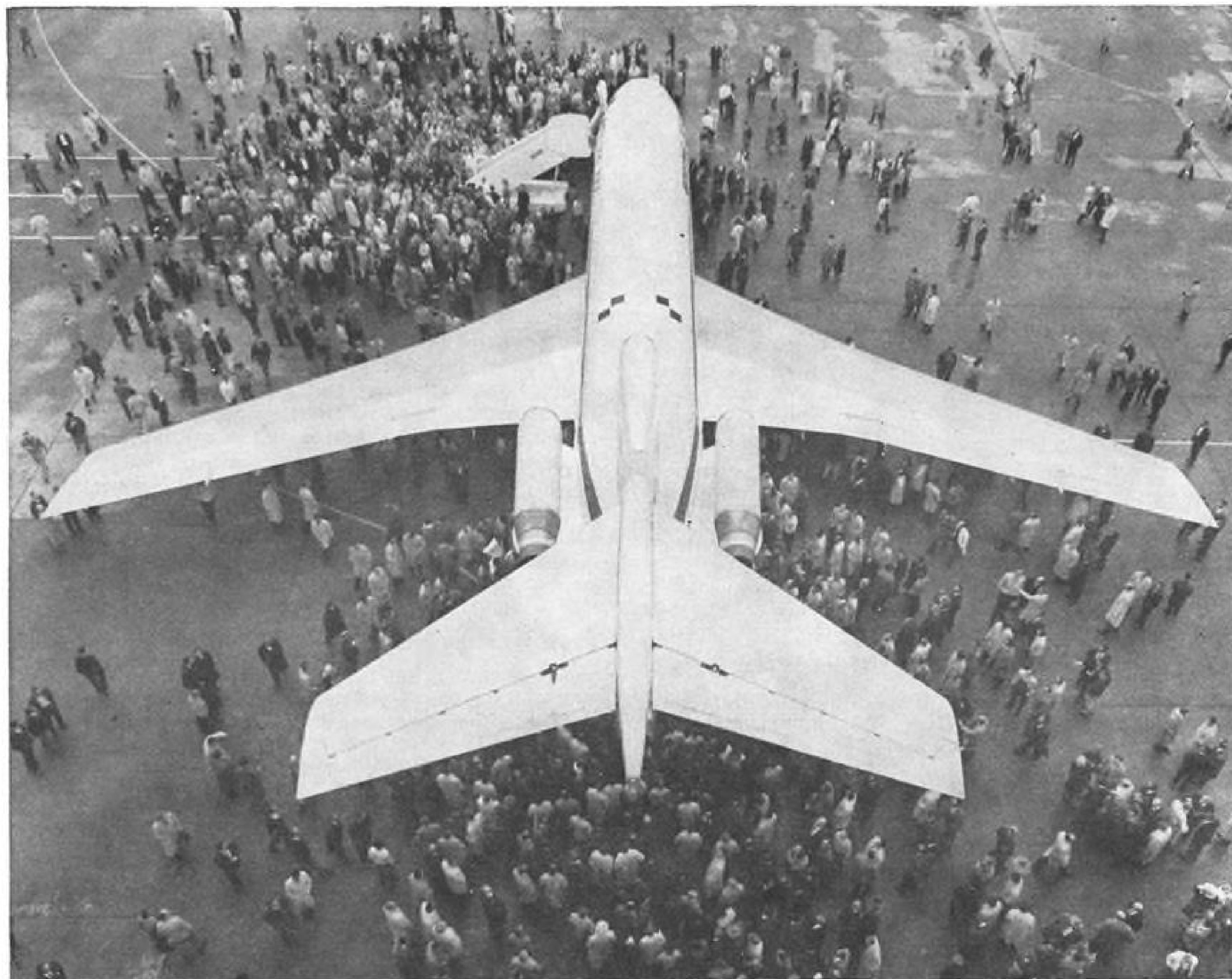
HIGH T-TAIL AND REAR-ENGINE configuration of the Boeing 727 are emphasized in this view of the new short- to medium-range jet transport at its rollout Nov. 27 (AW Nov. 26, p. 42). Plane is painted in brown and yellow color scheme featured on the original prototype Boeing 707. Aircraft is powered by three Pratt & Whitney JT8D-1 engines each rated at 14,000-lb. thrust for takeoff.
