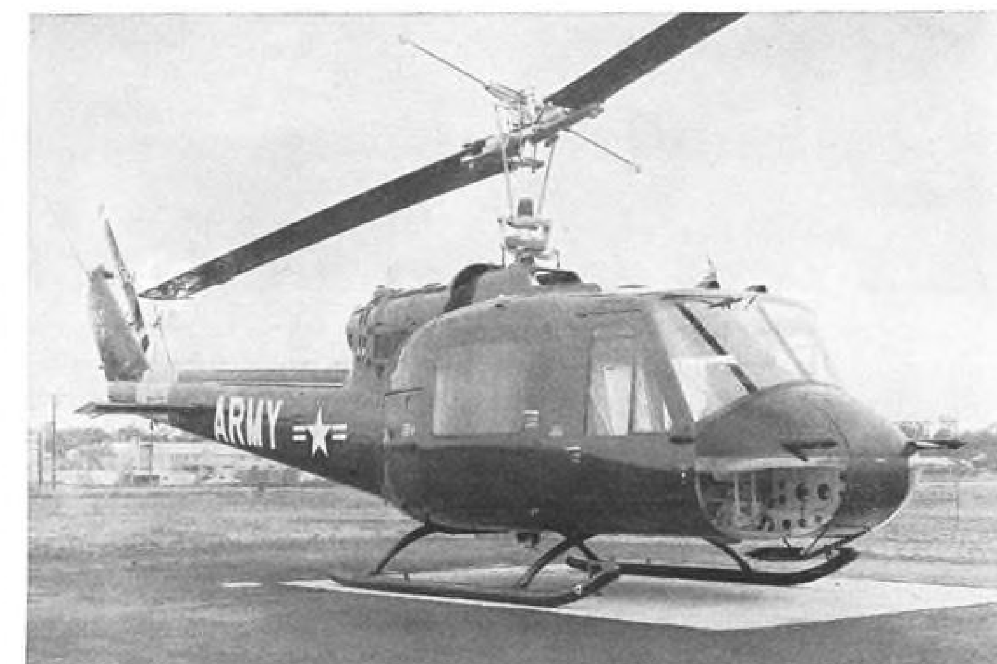
CLEANED-UP FRONTAL AREA of the modified research Bell UH-1B, top, is evident in comparison with standard model, below. Antennas and rear view mirrors on nose have been removed and landing skids considerably reduced in size.
