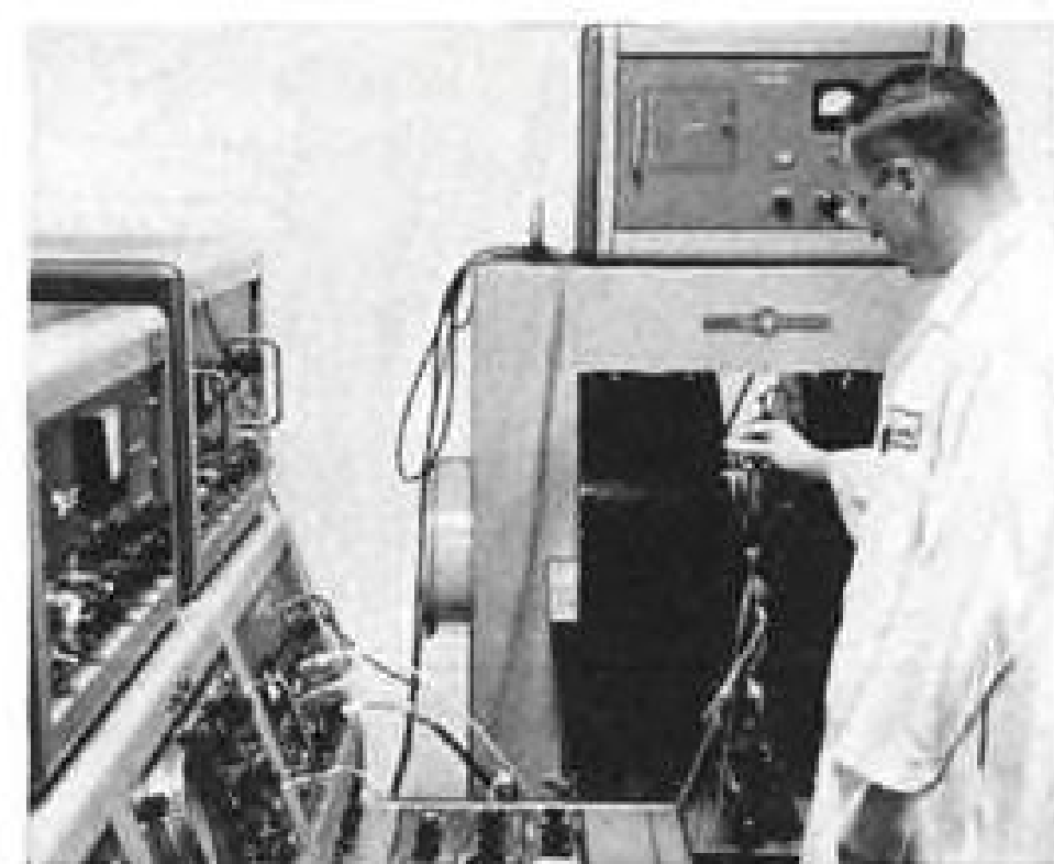
NUCLEAR MAGNETIC RESONANCE SPECTROMETER. Advanced scientific apparatus used to determine molecular structure of exotic fuel components for purposes of predicting their behavior.
