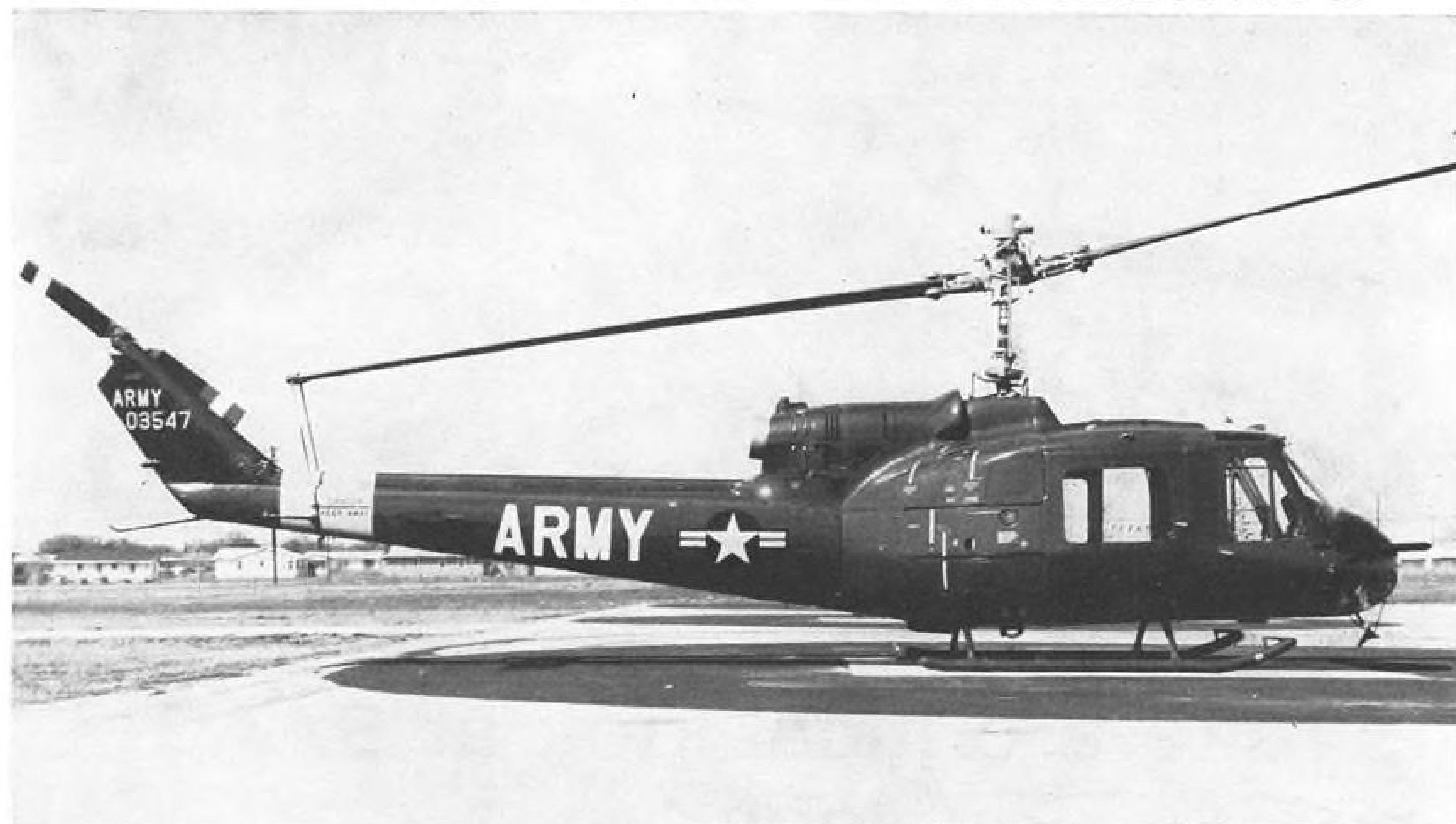
STANDARD ARMY UH-1B shows traditional cluttered appearance of most present-day rotary wing aircraft. Note drag-inducing rotor mast, unfaired engine cowling, and aft cabin area which recedes sharply into tail boom.
