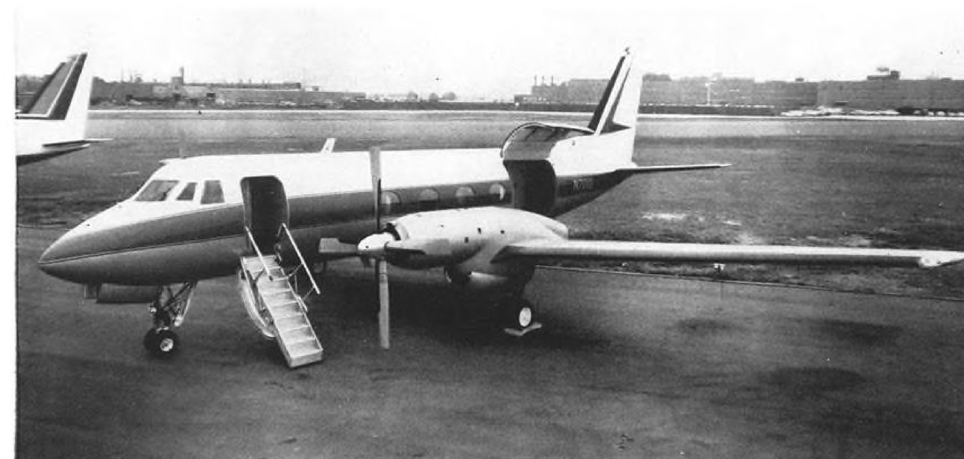
Grumman Gulfstream turboprop transport with large rear cargo door has received FAA certification. Aircraft seats a maximum of 24 persons.
