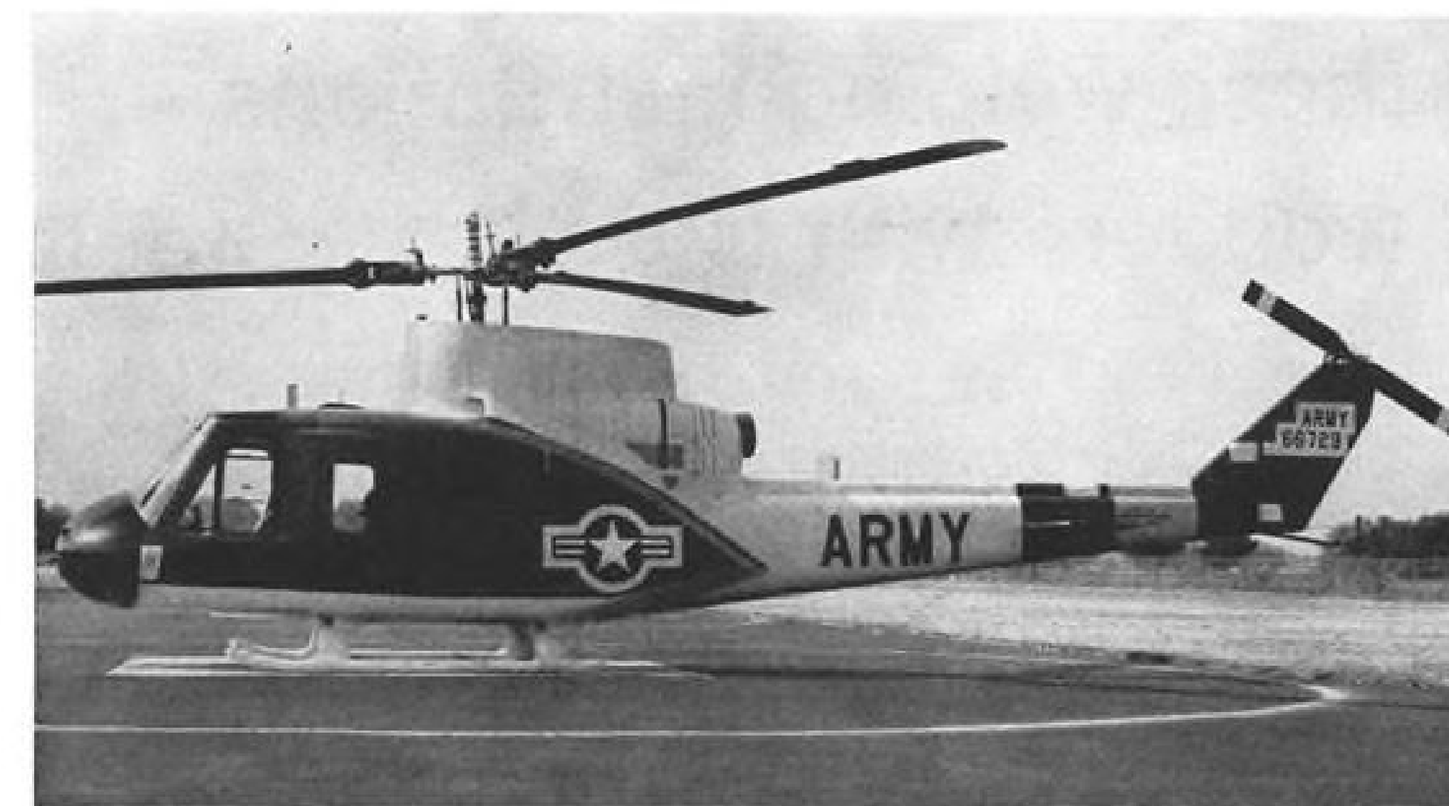
LATER VERSION of the research UH-1B has a three-bladed rotor and will be used to further extend the helicopter's speed range. Rotor configuration will include semi-rigid and rigid types. Note faired engine intake on lower portion of the forward pylon fairing.
