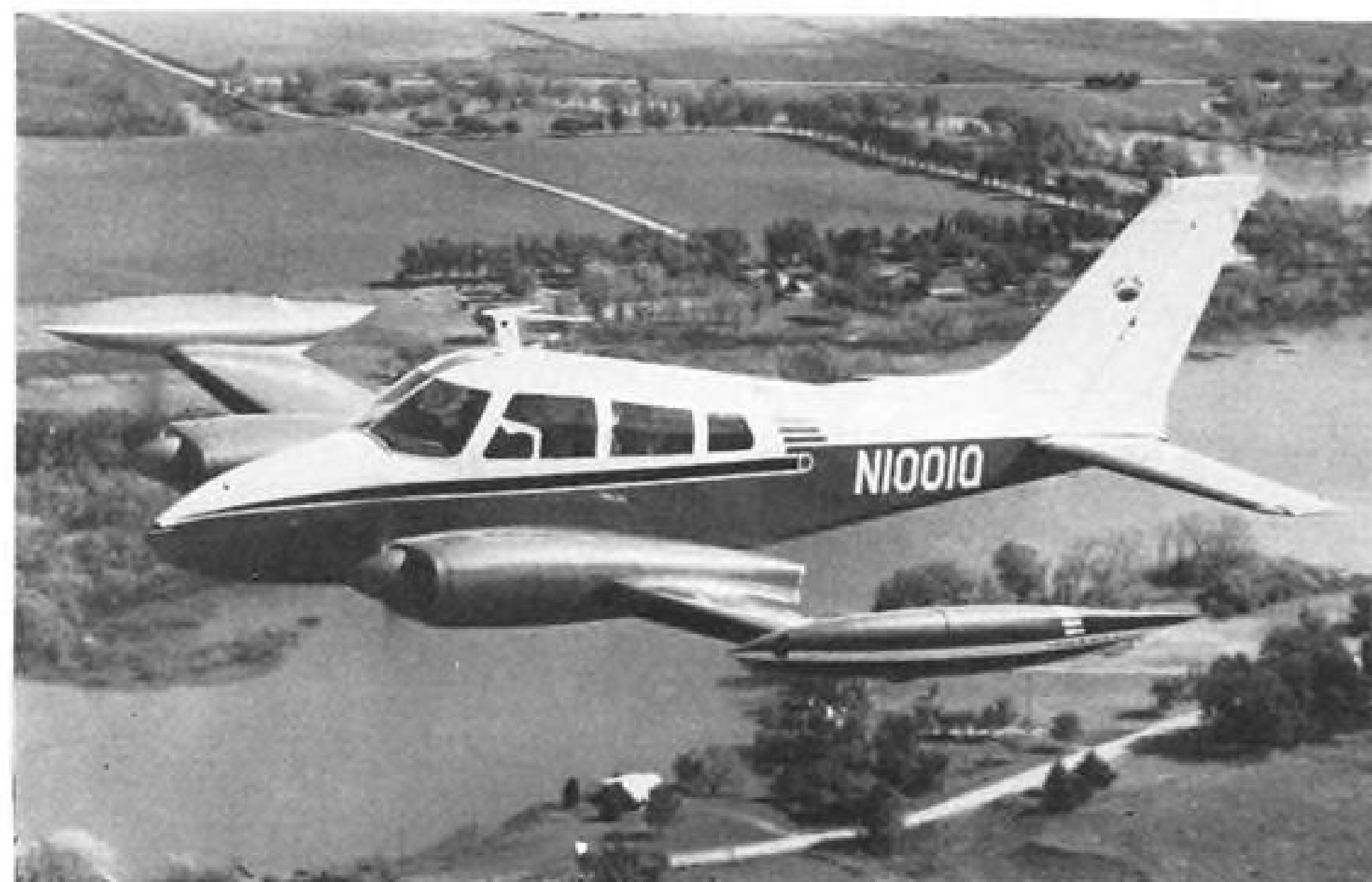
CESSNA 310H has larger cabin, increased useful load and redesigned landing gear.
