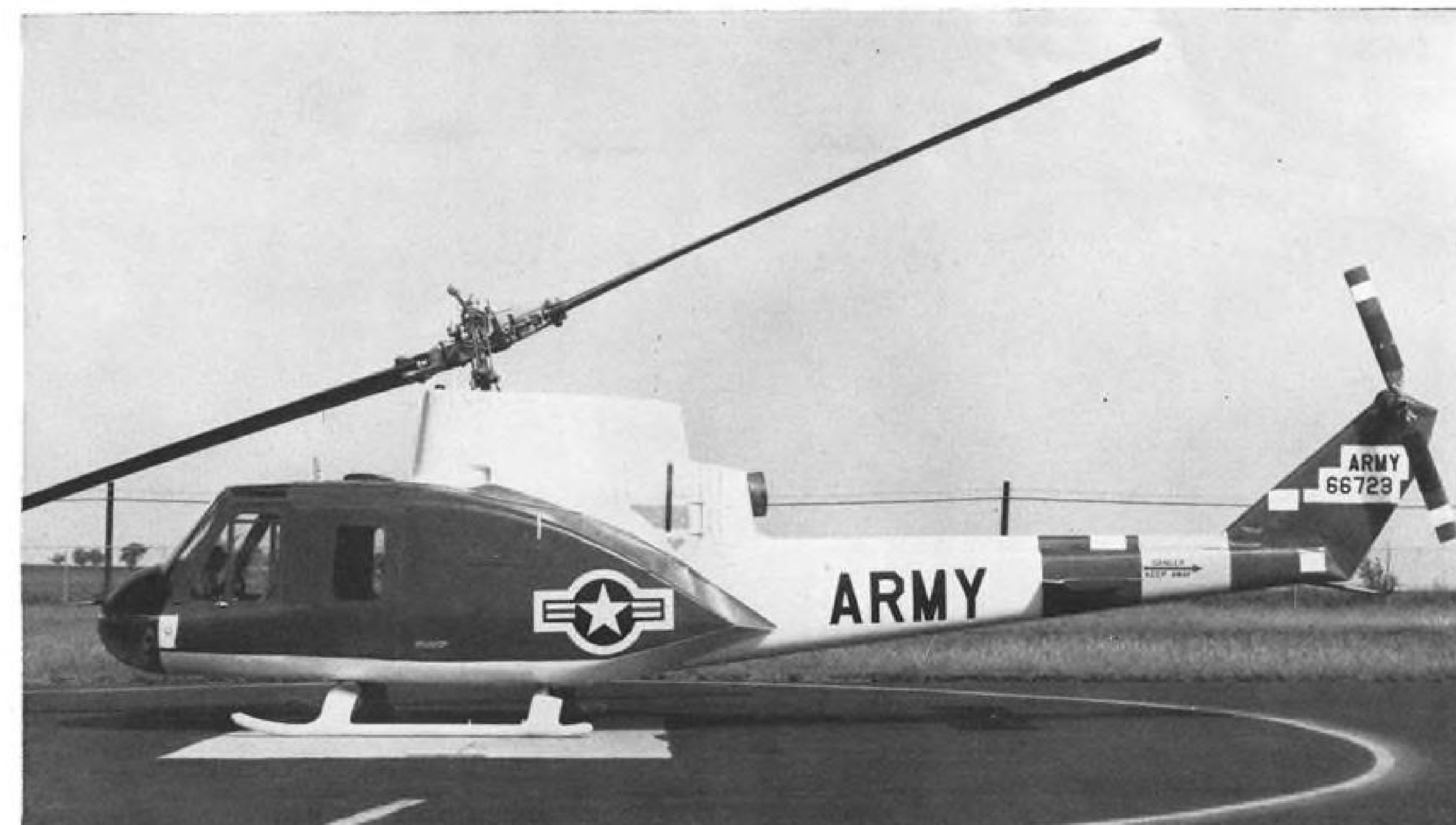
MODIFIED BELL UH-1B shows effects of aerodynamic cleanup. Helicopter still had cluttered mast when photo was taken, but fairing covered most of it, along with engine. Airfoil-shaped fairing was added to rear cabin and numerous minor changes were made.
