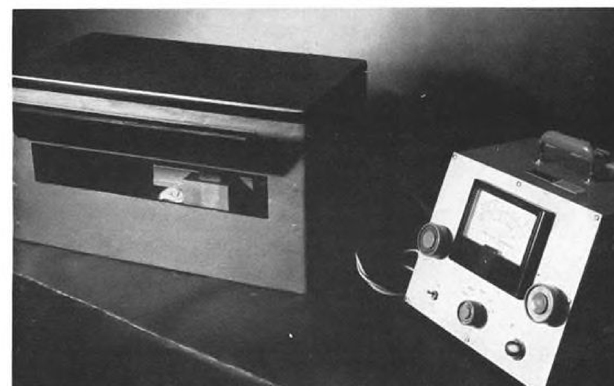
LIGHT TIGHT BOX , left, holds bioluminescent fungi and photomultiplier tube. Signal from tube is amplified and recorded on the instrument at right.
