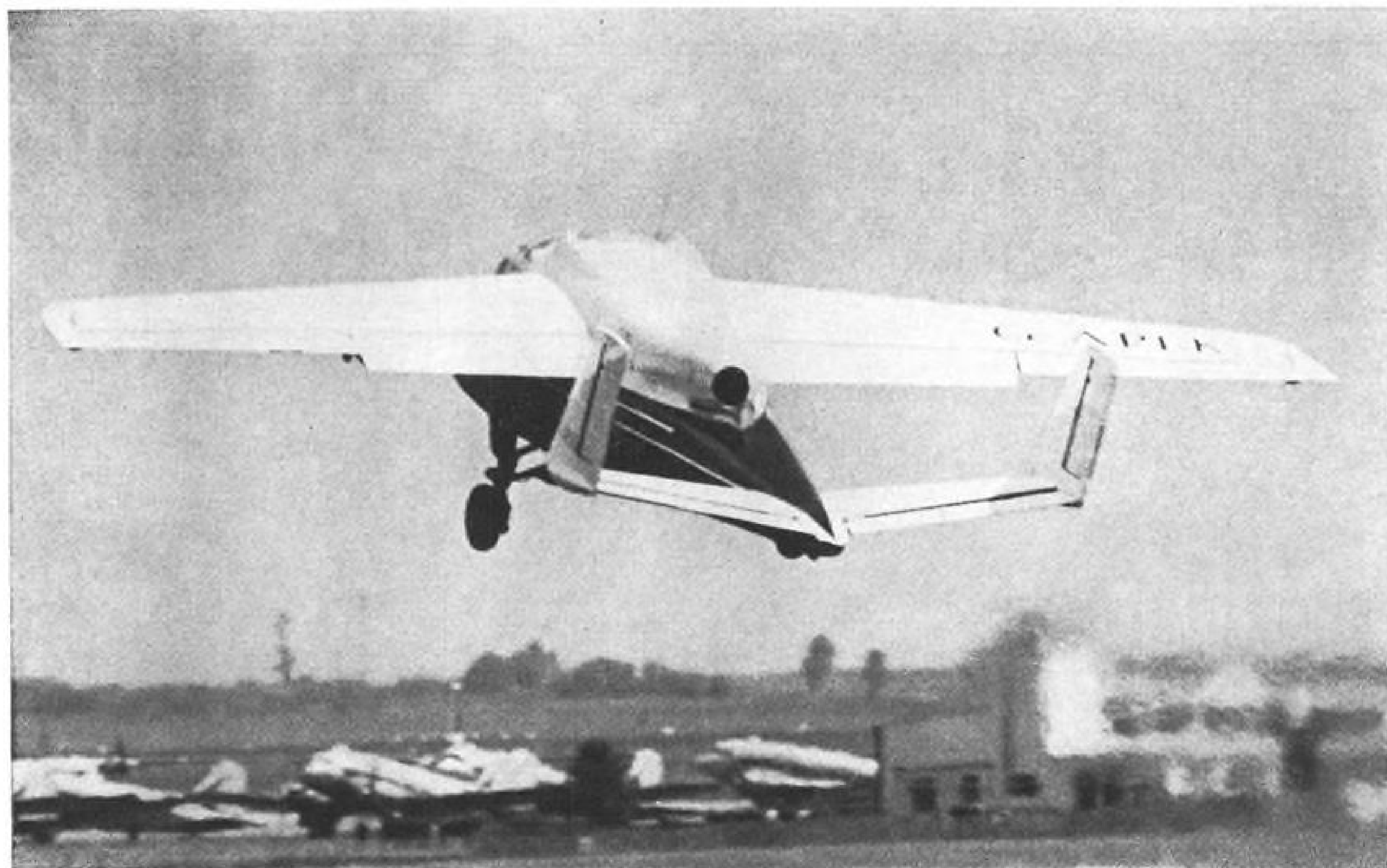
POWERPLANT FOR MILES STUDENT is a Turbomeca Marbore 2A turbojet engine of 880 lb. thrust. Follow-on Miles Graduate will be powered by a Turbomeca Aubisque turbopan of 1,550 lb. thrust; no major changes to airframe are needed.
