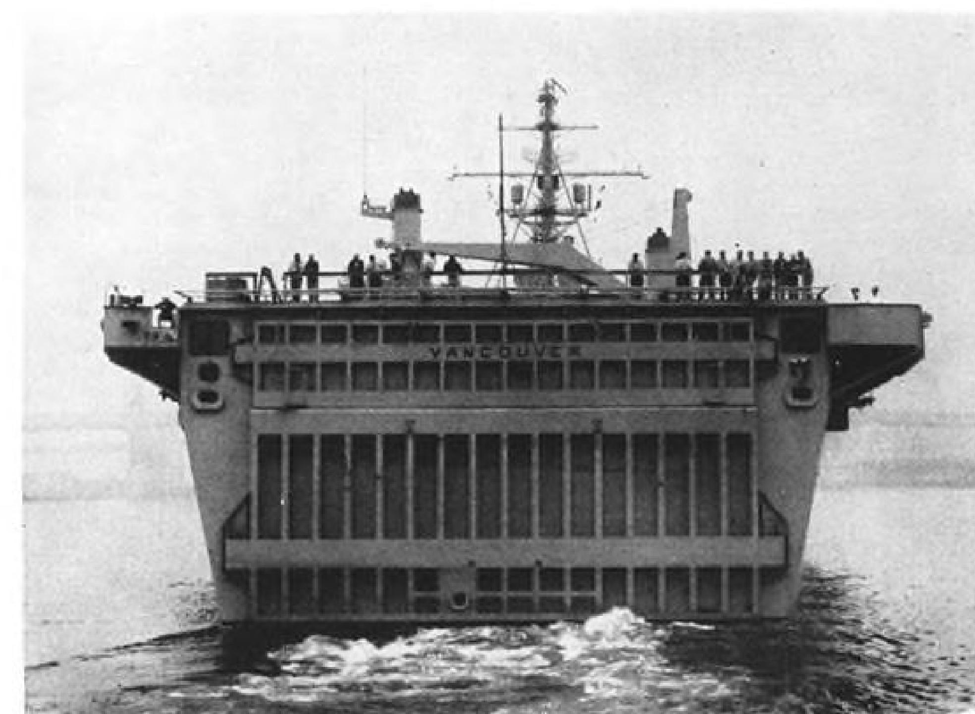
VANCOUVER'S STERN shows the hinged doors leading to the well or dock, through which landing craft carrying equipment are launched while troops are airlifted ashore.
