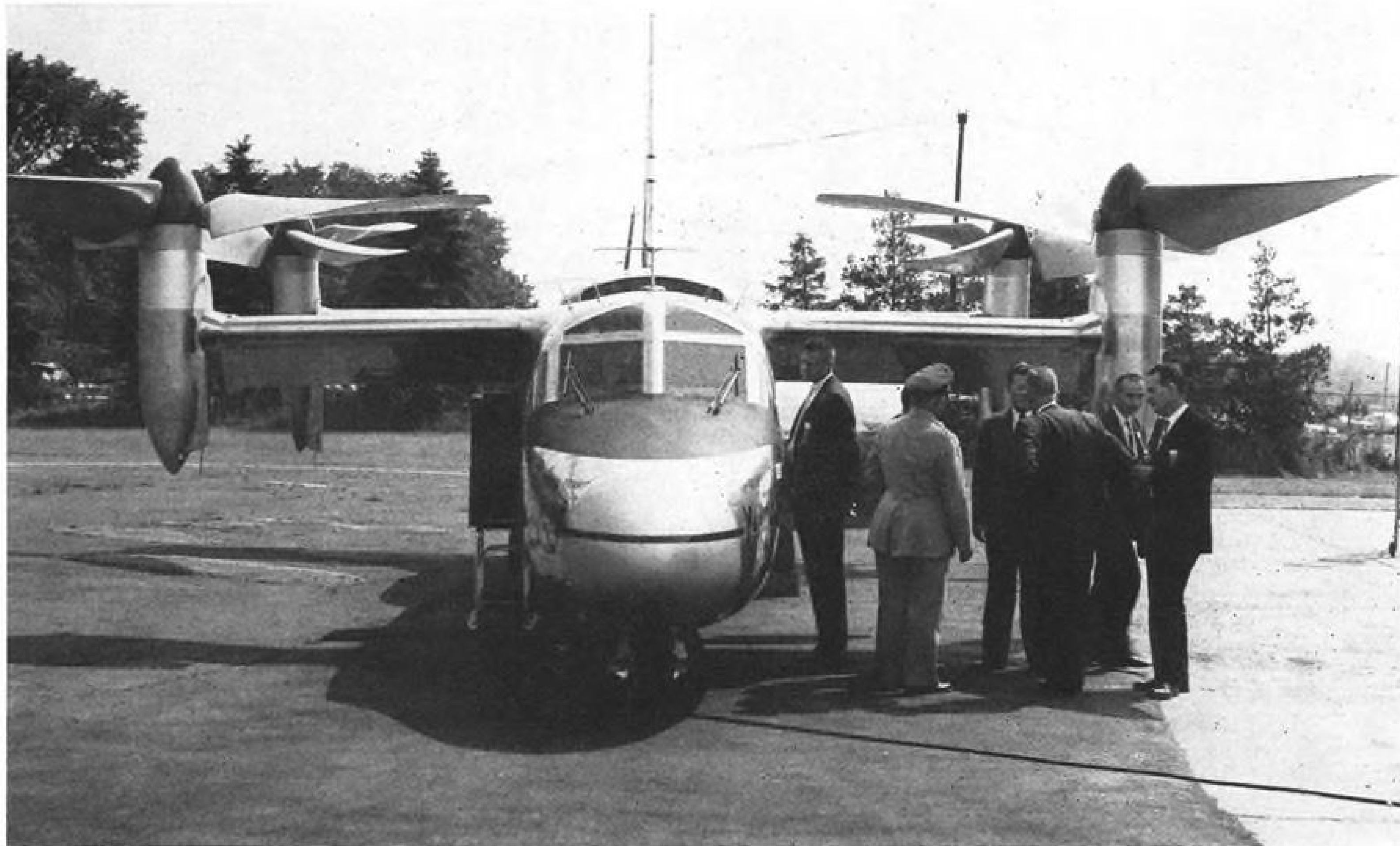
Curtiss-Wright X-19 VTOL is beginning ground engine runs and taxi tests prior to the first flight scheduled for October. The research vehicle was rolled out recently (AW July 29, p. 25) at the company's Caldwell, N. J. facility.
