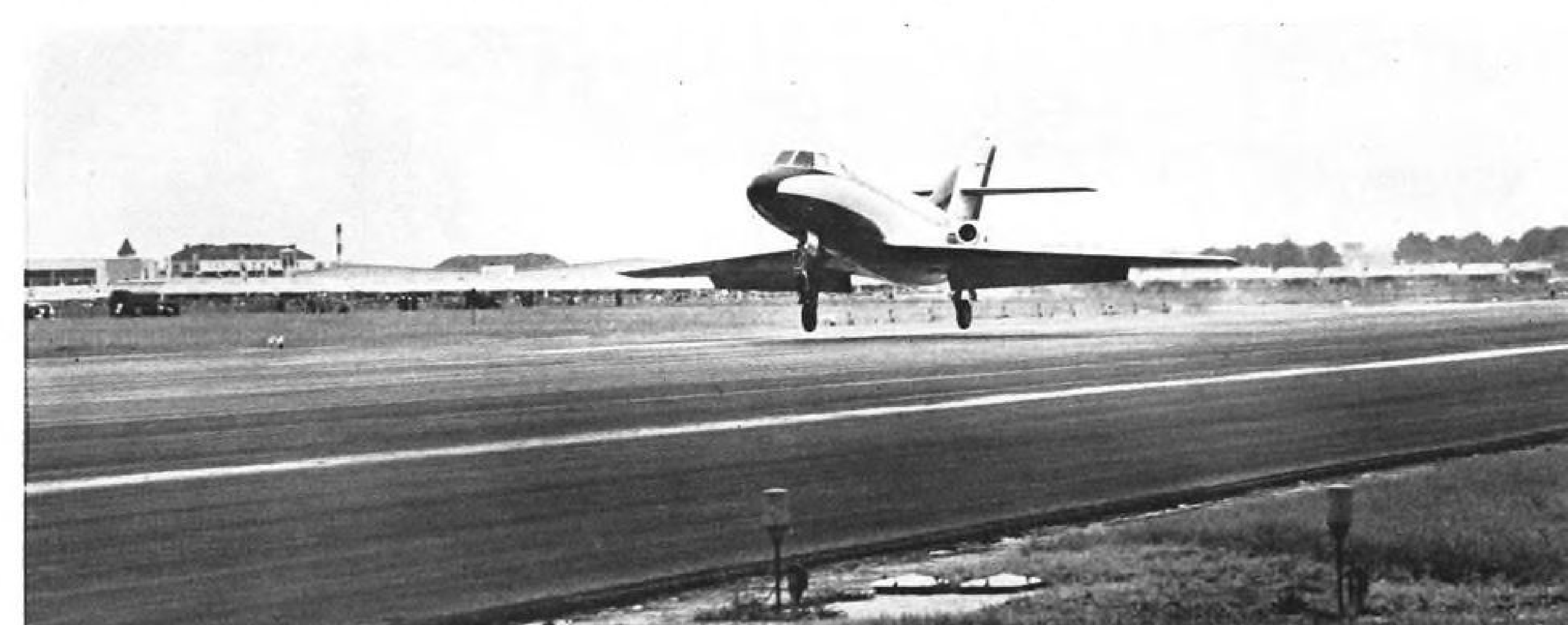
Landing distance for the Mystere 20 is given as 2,624 ft. for either the Pratt & Whitney- or Bristol Siddeley-powered version. Approach speed for both is 110 kt. Maximum range with IFR reserves for either aircraft is quoted at 1,366 mi.
