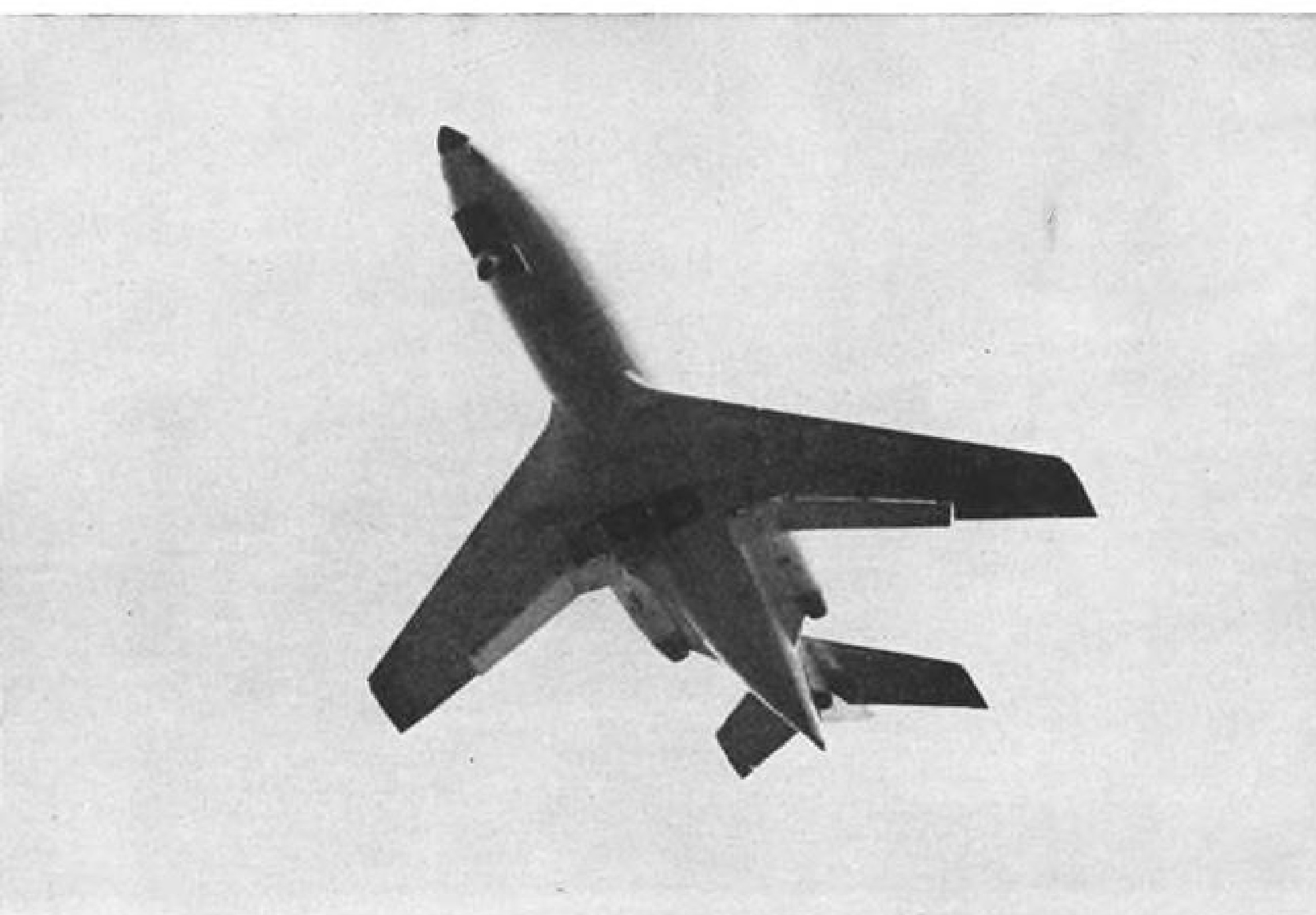
Dassault Mystere 20, powered by Pratt & Whitney JT12A-8s in eight-passenger configuration, has maximum takeoff weight of 19,290 lb.
