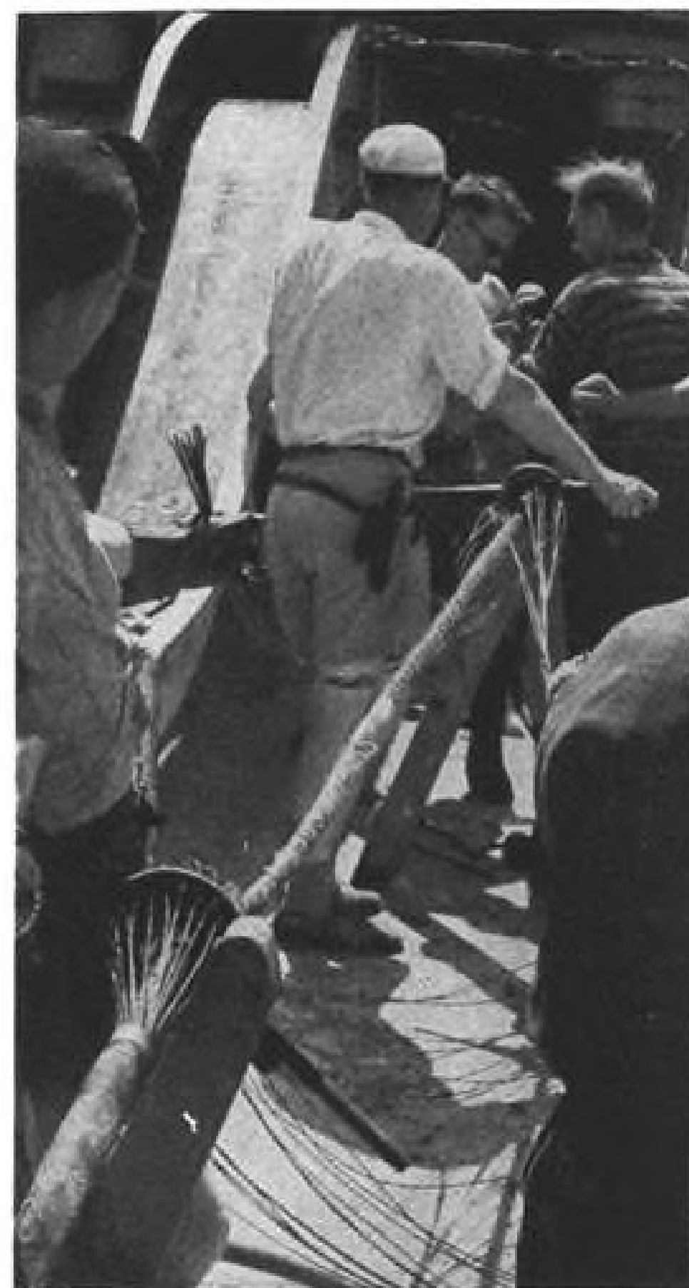
CONTRAST with modern technology is provided by these cable-wrapping operations on deck of Neptun involving techniques dating back to 19th century.
