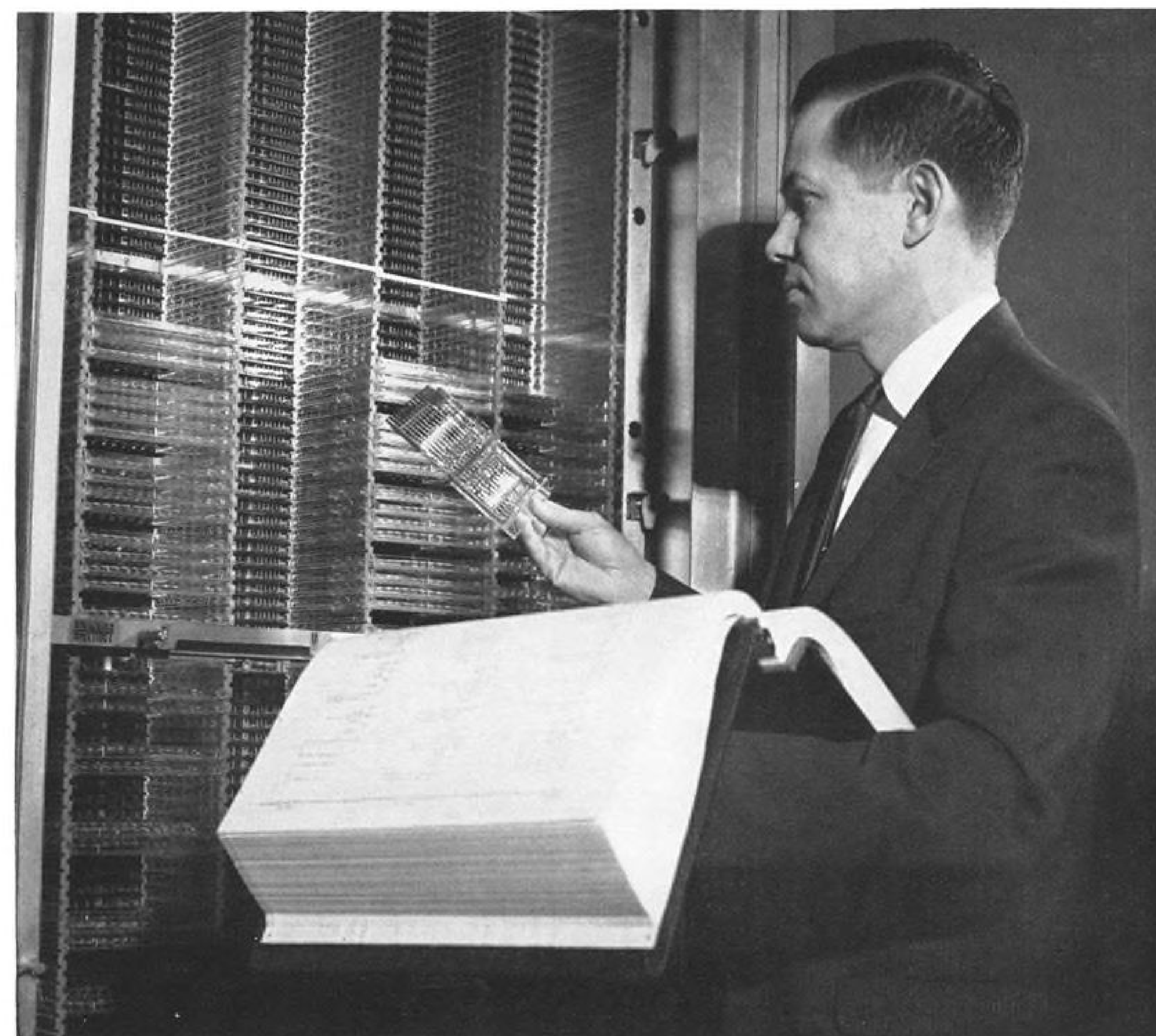
Dictionary refers R. Ketchledge, Director of the Bell System's Electronic Switching Laboratory, to faulty components in a model of the electronic switching system.
