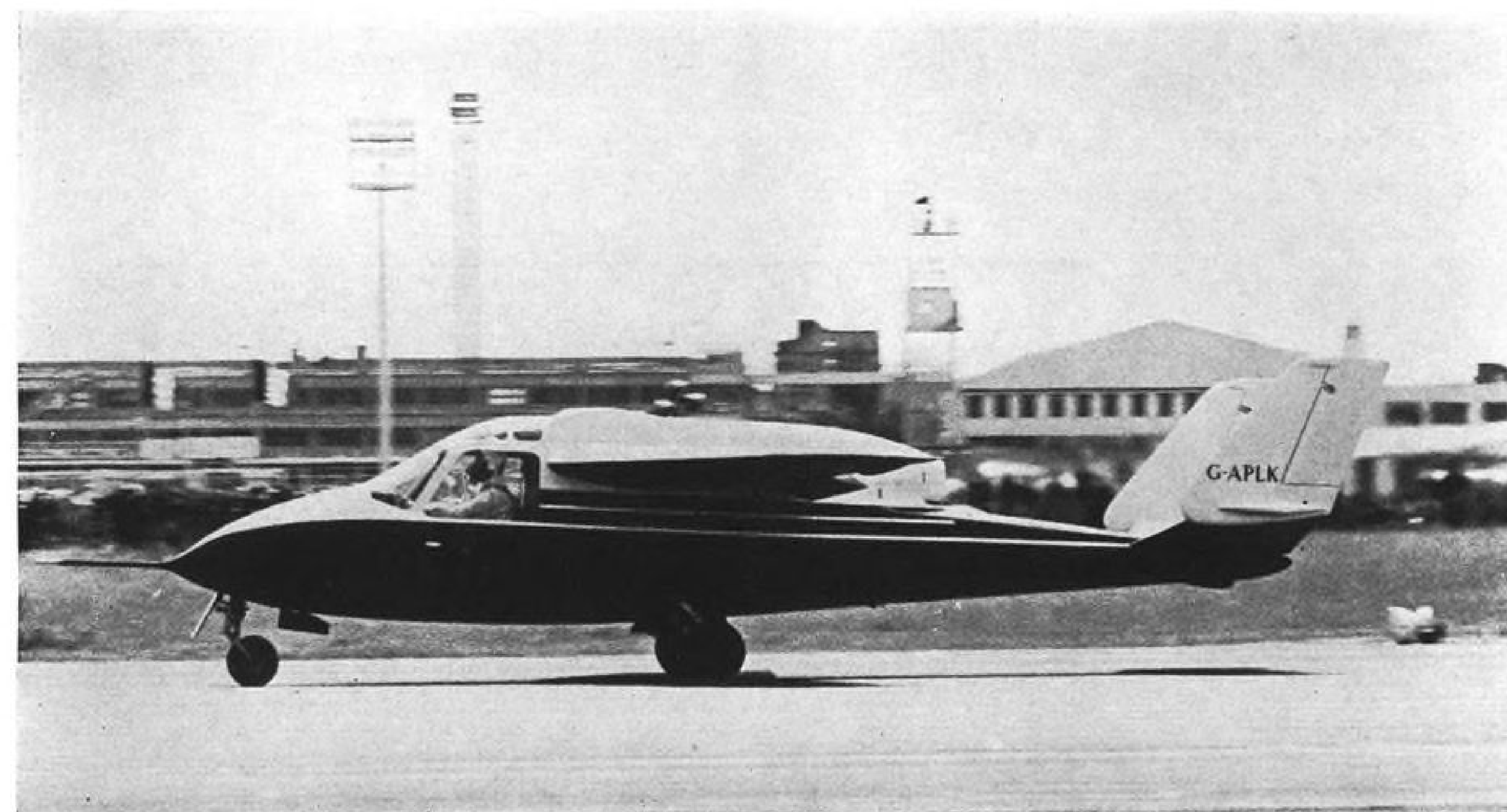
MILES M-100 STUDENT , ready for takeoff at Le Bourget Airport during the Paris Air Show, is two-place, side-by-side trainer which can be stretched to a four-place communications airplane by adding seat in equipment section.
