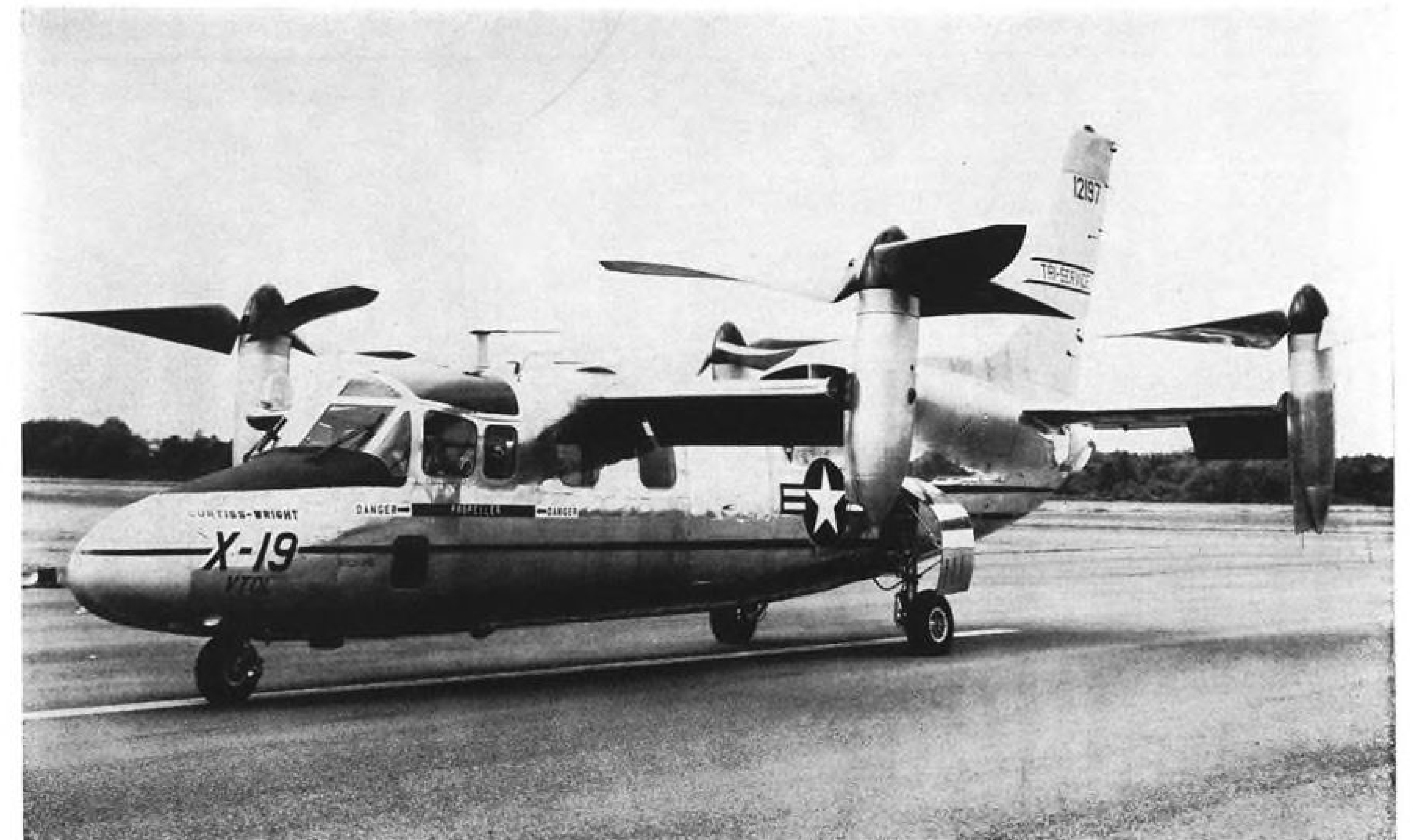
Short-span wings, located fore and aft of the X-19's center of gravity, provide lift during high-speed flight. Lift in hover is provided by propeller thrust alone and during transition lift is provided by a combination of wing, propeller and radial propeller force.
