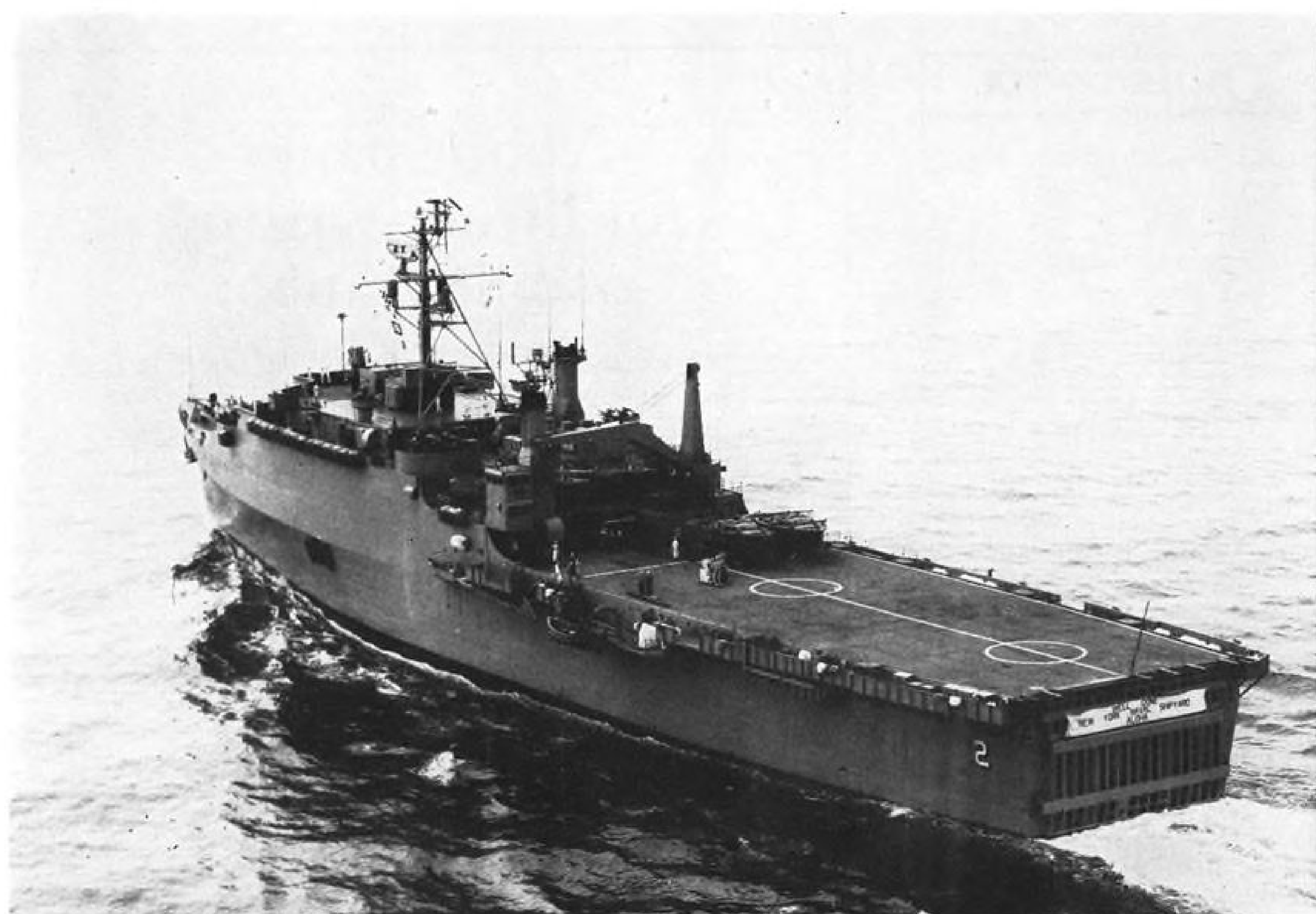
USS VANCOUVER (LPD-2), shown under way above, features a landing deck for six to 10 helicopters, an approach control tower (port side amidships) and a crane for lowering boats. Ship carries 900 Marines and landing craft for heavy equipment.
