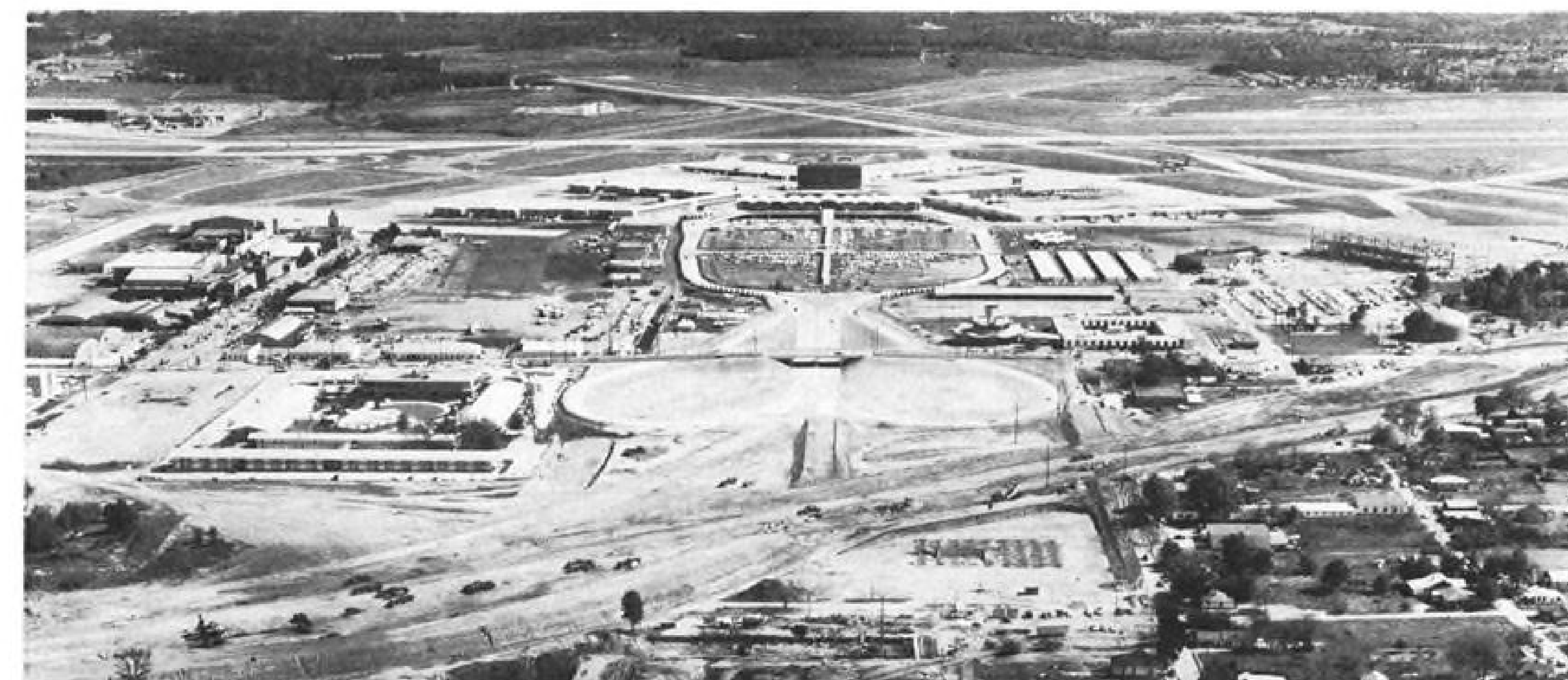
LONG-RANGE VIEW of Atlanta Municipal Airport shows layout of finger design and proximity to the runway system. Area at upper left is portion of old terminal center, now used to accommodate cargo and general aviation operations.
