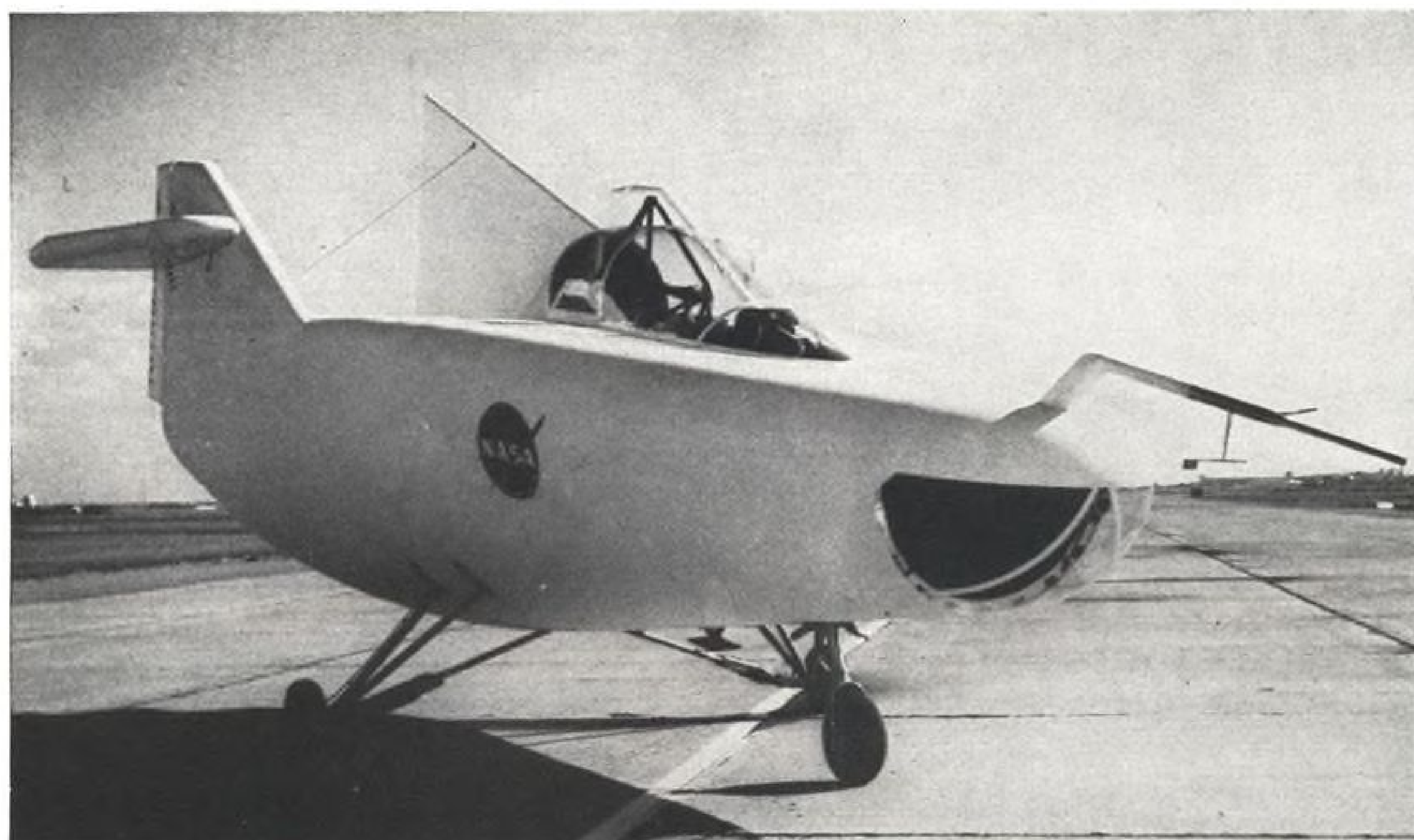
CONICAL LIFTING BODY model developed by Flight Research Center is a 900-lb. glider model of the M-2 lifting body under study.
