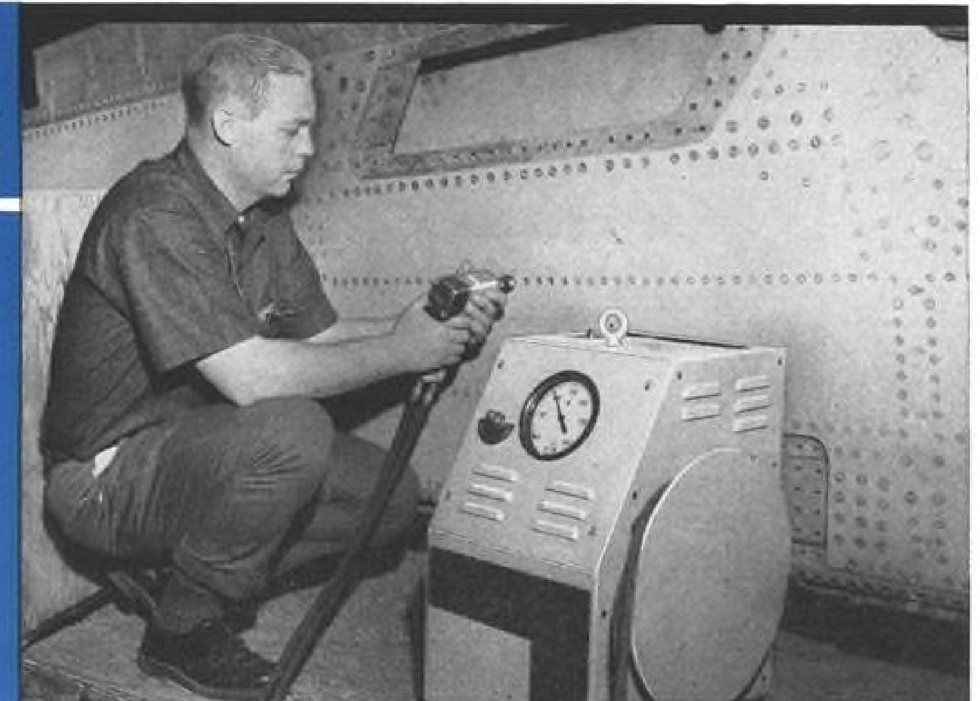
Blind Bolts being installed in RF101C lower tapered skin covering main torque box after wing removal from rework jig. Hi-Shear Corp. portable power units (BP4000 electrically operated model shown) provide hydraulic power to the Blind Bolt Gun. Air operated model is non-sparking and safe for use near fueled aircraft or launch ready vehicles.
