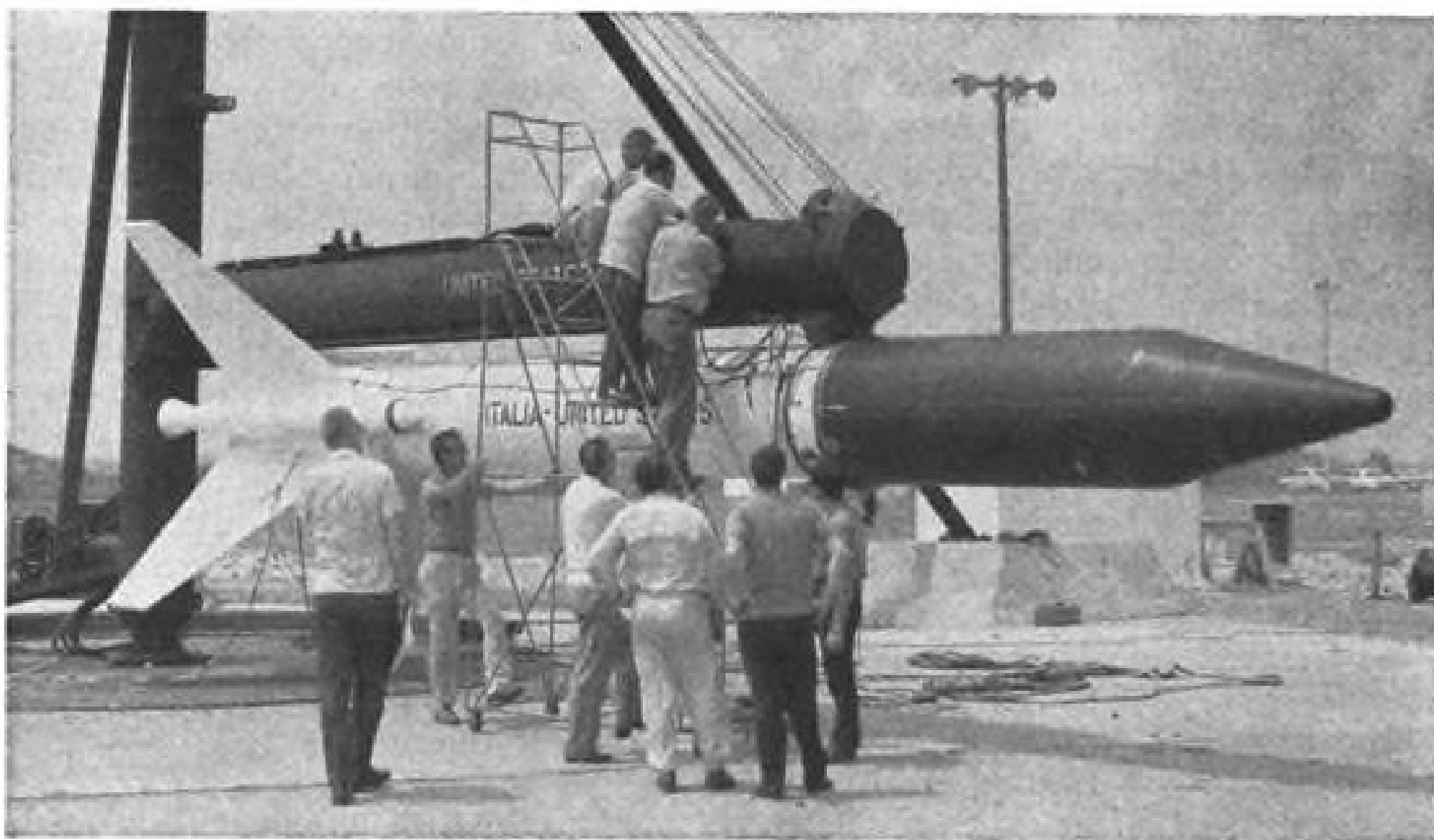
SAN MARCO PAYLOAD is prepared for a sounding rocket test from Wallops Island, Va., by U.S. and Italian technicians. The payload is shown both with the fairing removed and in place. San Marco, which is scheduled to be launched from a platform in the Indian Ocean near the equator, is one of a number of bilateral space projects in which the U.S. is involved. The sounding rocket, called Shotput, consists of a Thiokol Pollux E6 first stage with two Thiokol Recruit assist rockets. At launch, the combination provides 120,000 lb. thrust. The second stage is an X248 Altair, manufactured by Hercules Powder Co.-Allegany Ballistics laboratory. The vehicle has a launch weight of 11,000 lb., and is 32 ft. long with a 33-in. dia.
