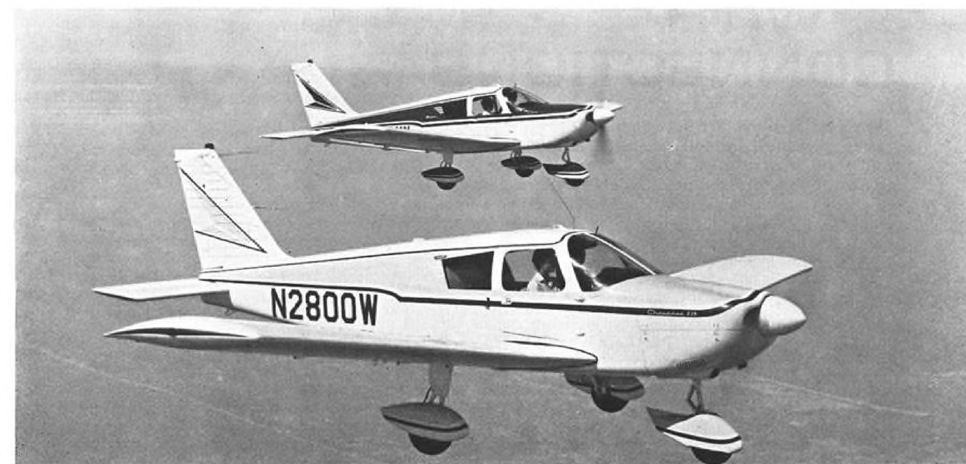
PIPER CHEROKEE 235, latest addition to the company's four-place, fixed-gear airplane, has a distinctive contoured glass-fiber cowl to accommodate the 235-hp. Lycoming O-540-B2B5 engine. Gross weight has been increased to 2,900 lb. and useful load is 1,490 lb.
