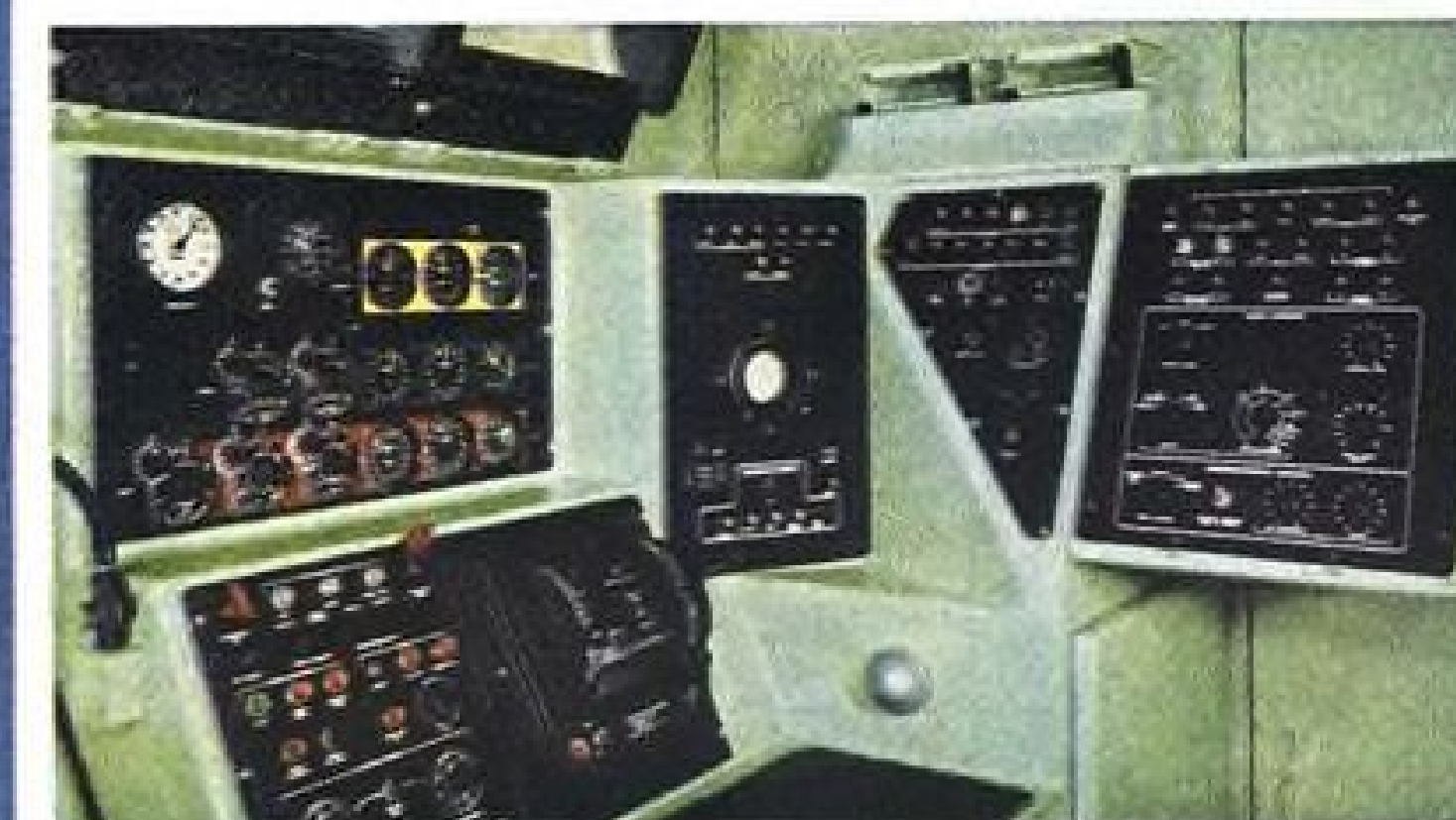
MOBILE TACTICS SIMULATOR for F8U-2N all-weather fighter. GAC-designed and built for U.S. Naval Training Device Center. Trains Navy pilots to intercept, select armament and make "kill," under conditions where target can be seen only as radar blip.
