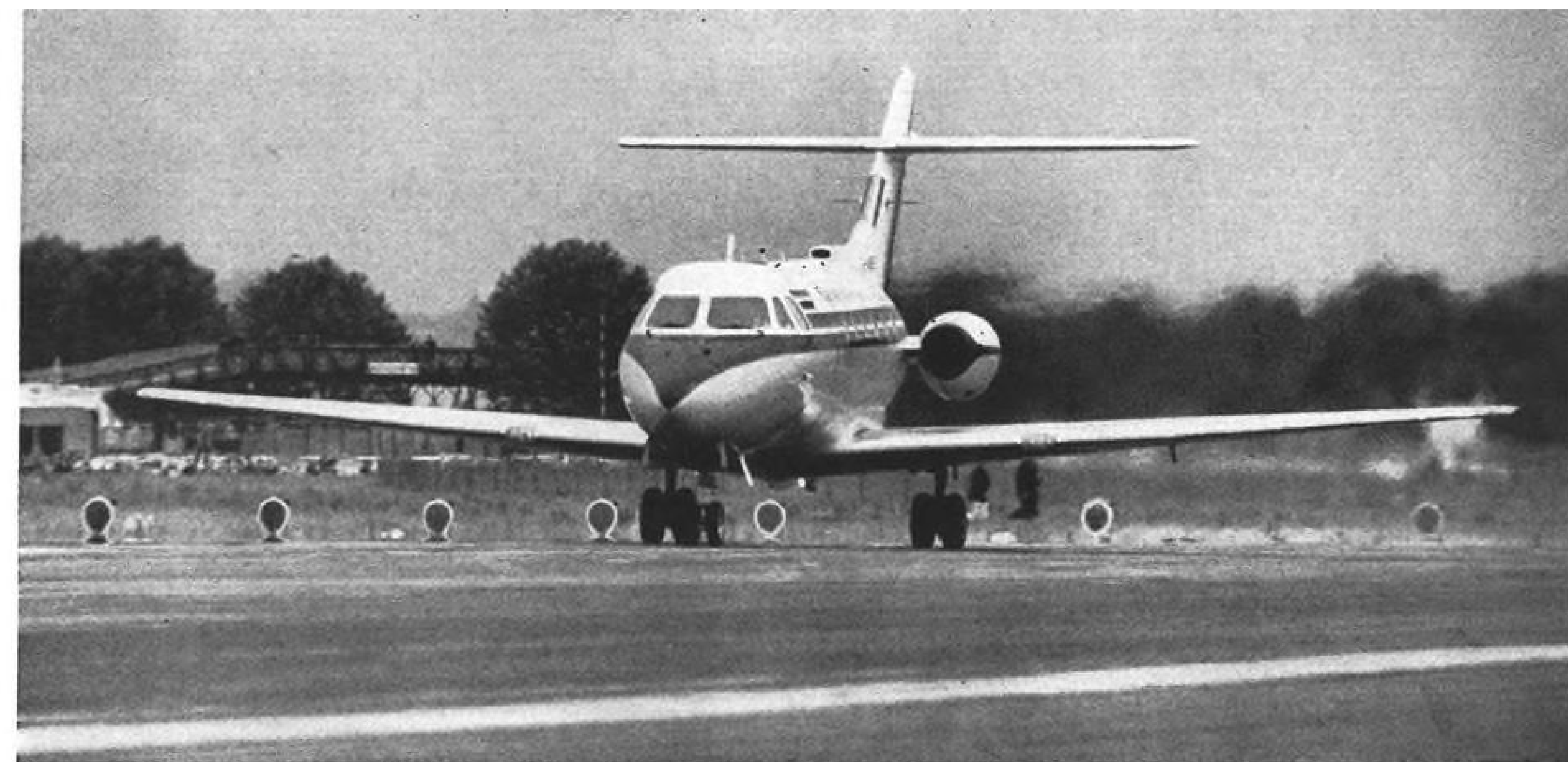
DH-125 TENDS TOWARD flat approach on landing, due to swept wing. Pilot does not have to begin flareout until reaching the runway lip. The aircraft requires a short ground run after settling on its main gear.
