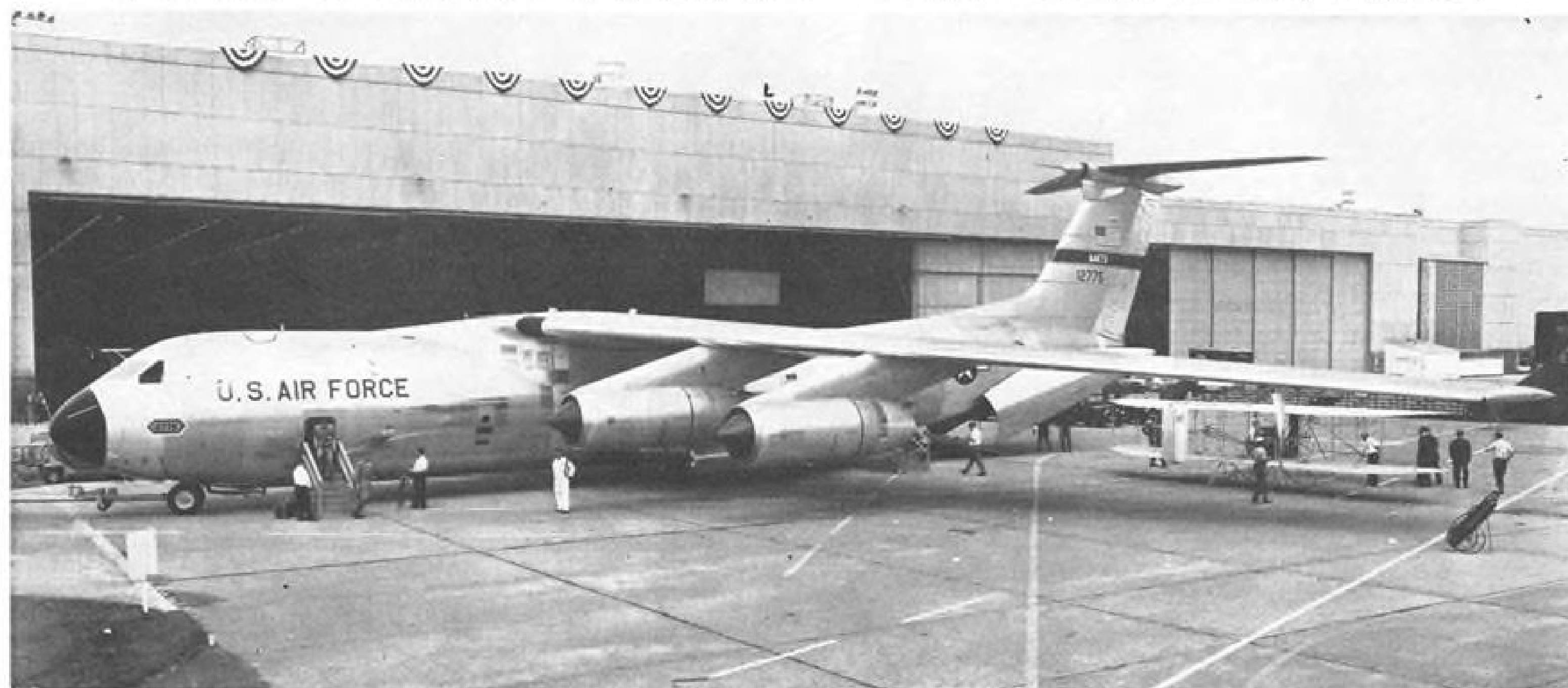
CLEAN FEATURES OF THE C-141 are evident in external view. Ground clearance at maximum gross weight is 19 in.
