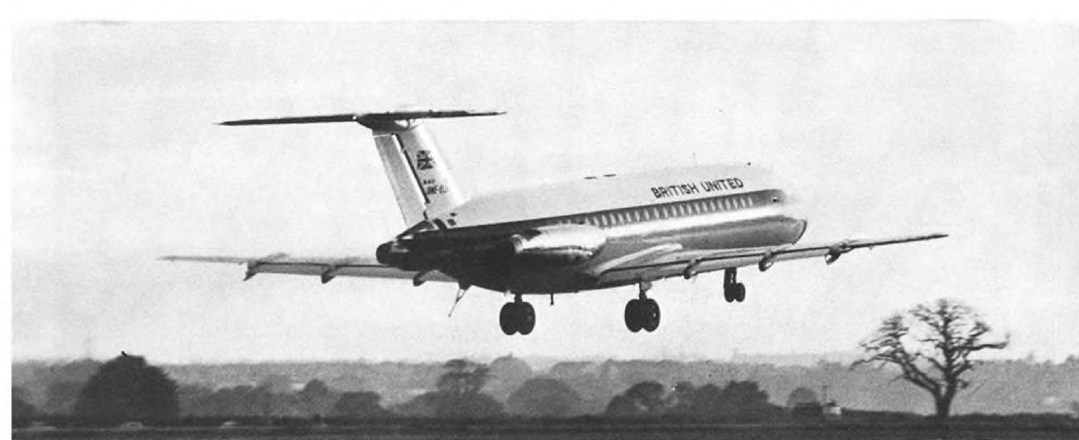
Starting climbout (above) with takeoff flap setting of about 15 deg., BAC 111 begins 27-min. maiden flight. Note slight upward deflection of the elevators on aircraft's moving tail plane. Landing (below), BAC 111 is shown crossing the runway threshold at Hurn, prior to full-flap touchdown. Note Hunting Provost chase plane in background. Six BAC 111s will soon enter a flight testing and certification program.
