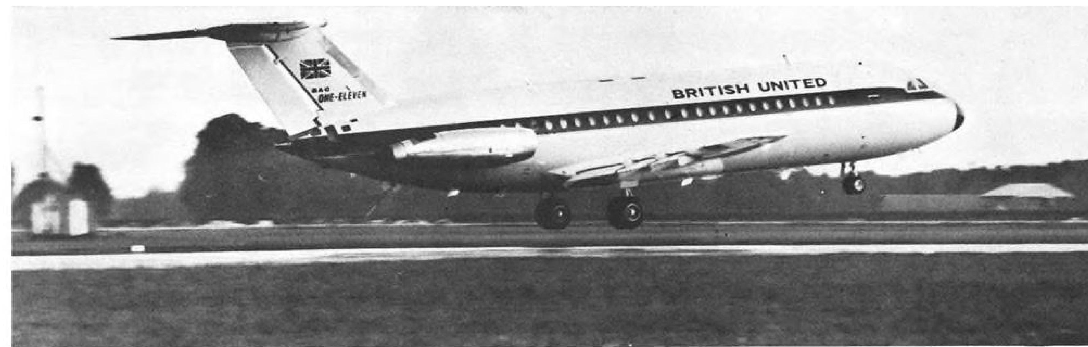
British Aircraft Corp.'s BAC 111, which made its maiden flight recently at Hurn, England, main assembly plant (AW Aug. 26, p. 39) is shown (above) as BAC chief pilot G. R. (Jock) Bryce lifted the aircraft after a ground run of about 3,000 ft. Gross takeoff weight was 59,000 lb. Tailhook-like extension from the fuselage is a proximity warning rod to provide cockpit warning if rotation is too steep.
