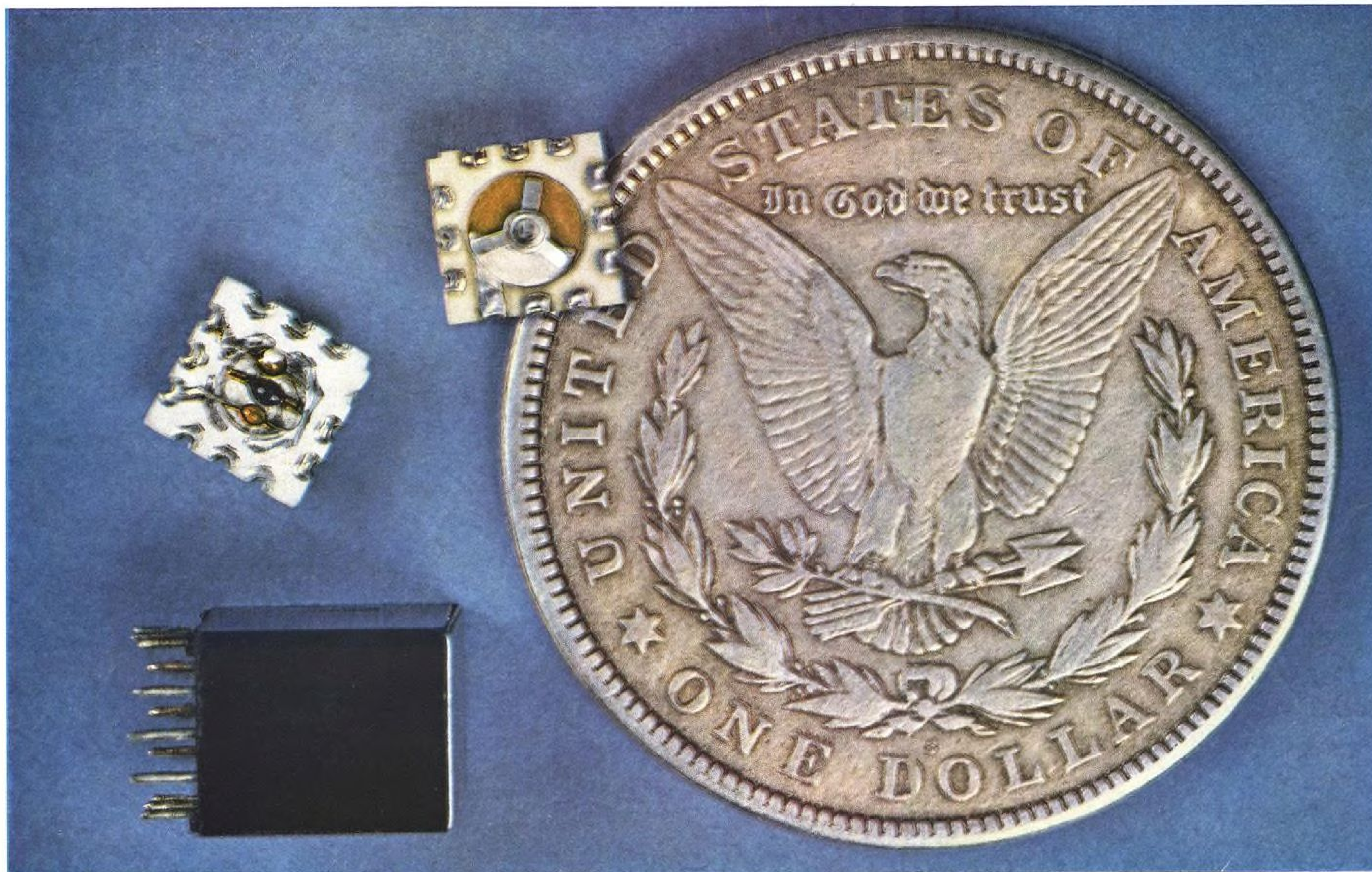
MICROMODULES —Micromodule element wafers and an encapsulated micromodule amplifier used in microminiature circuitry.
