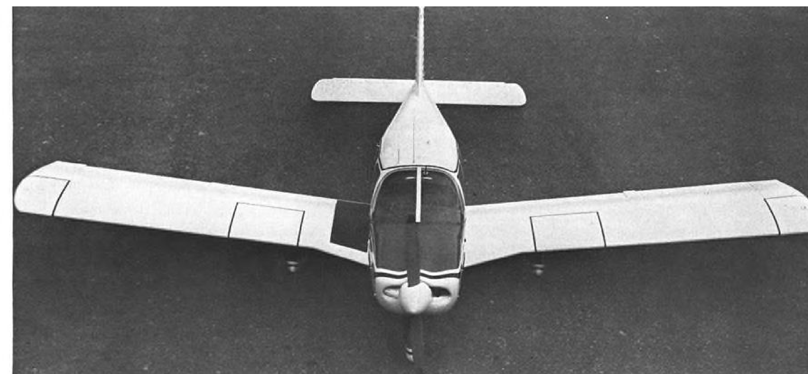
LONGER WINGSPAN of the new Piper Cherokee 235 is shown with additions to wingtips beginning at black lines, which indicate 17-gal. wingtip fuel tanks. Standard 25-gal. tanks are outlined on inboard leading edge of wing.
