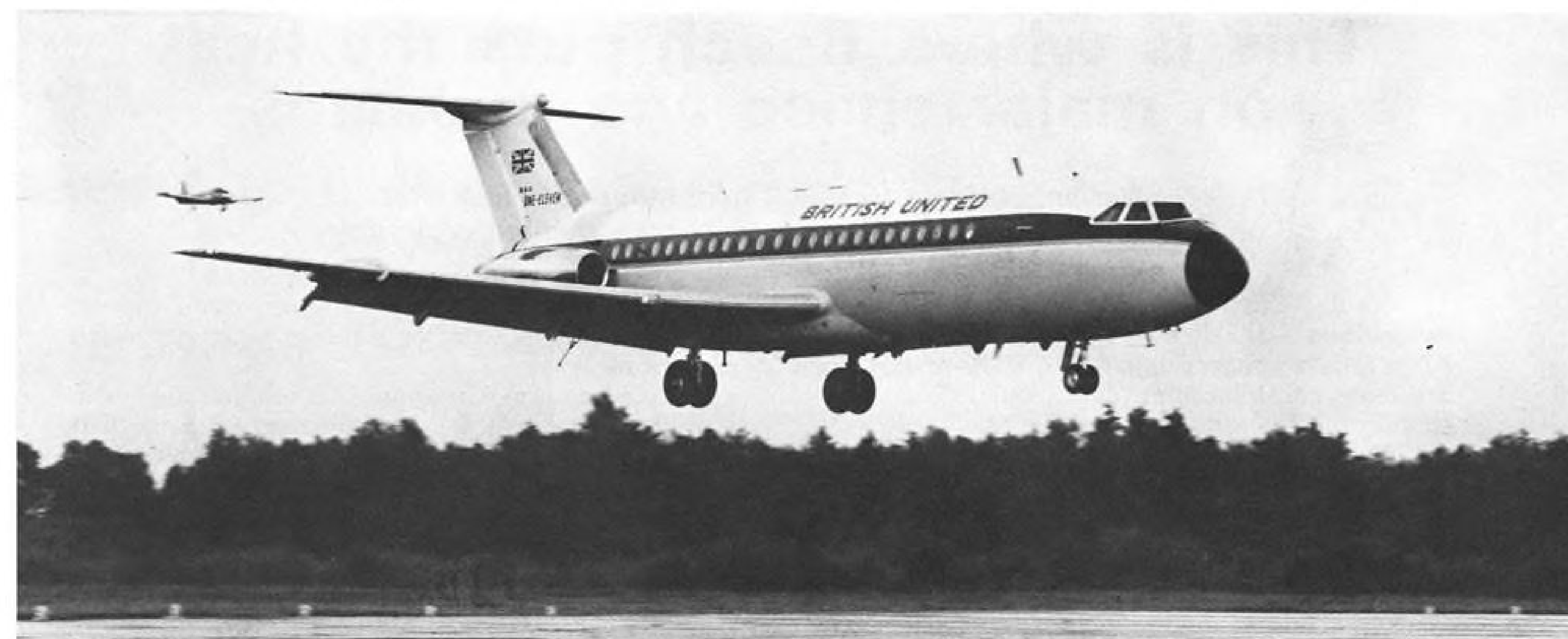
Starting climbout (above) with takeoff flap setting of about 15 deg., BAC 111 begins 27-min. maiden flight. Note slight upward deflection of the elevators on aircraft's moving tail plane. Landing (below), BAC 111 is shown crossing the runway threshold at Hurn, prior to full-flap touchdown. Note Hunting Provost chase plane in background. Six BAC 111s will soon enter a flight testing and certification program.
