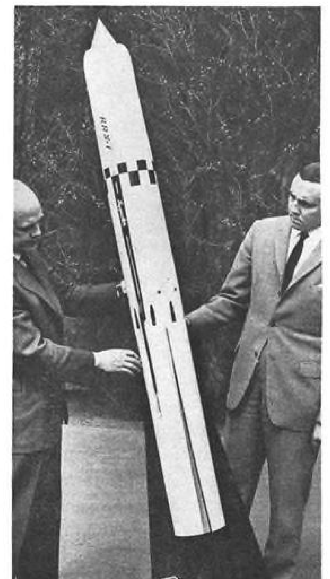
RB.322 TEST VEHICLE is shown, above, on launcher near Kiruna in northern Sweden. Vehicle reached Mach 3 speed and 75,000 ft. altitude in test series. RRX-1 ramjet, below, is for Mach 5 speed ranges.
