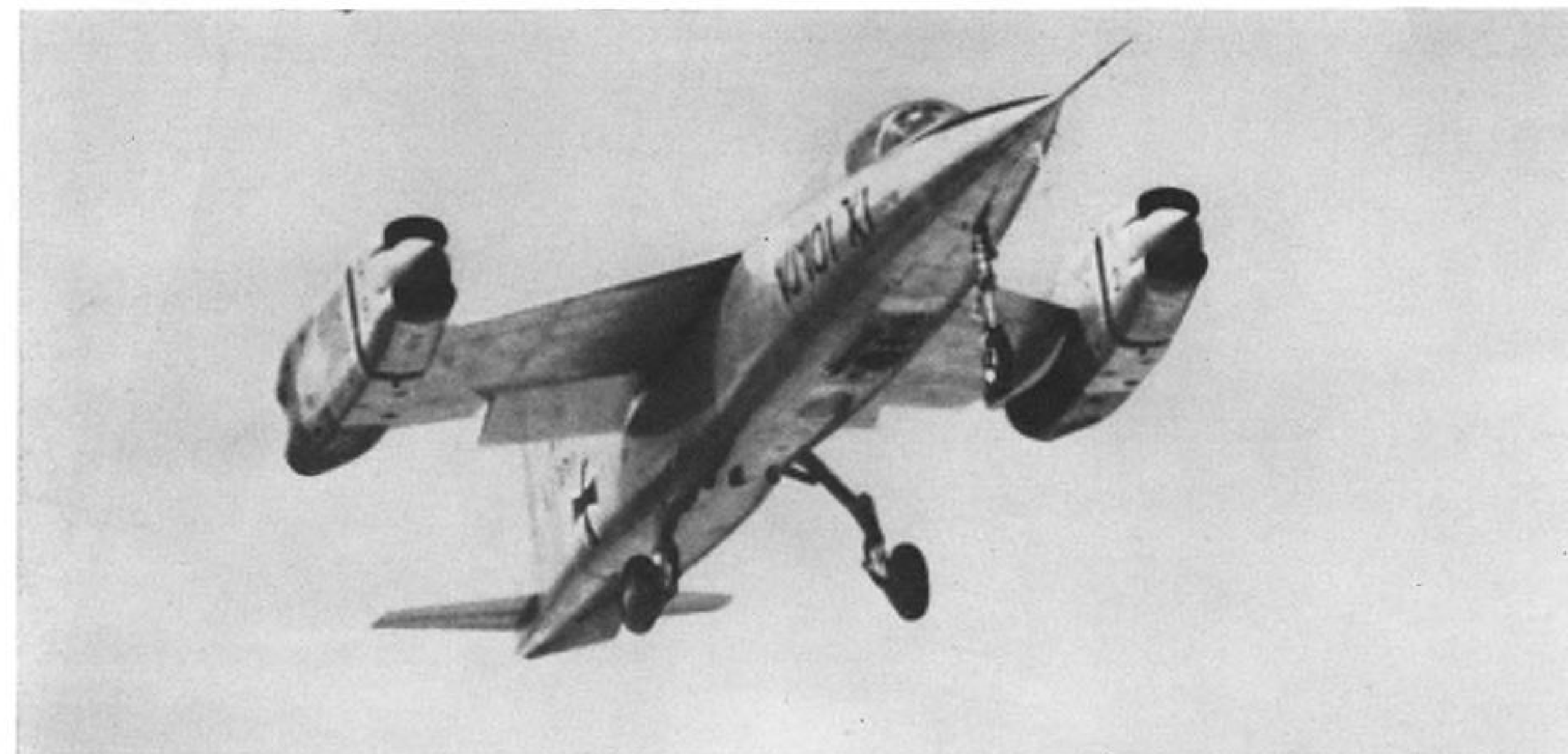
West German VJ-101C VTOL fighter is shown (above and below, left) in first full flight demonstration, including transition from vertical to horizontal flight. Photo above shows the aircraft accelerating into forward flight after the transition phase.
