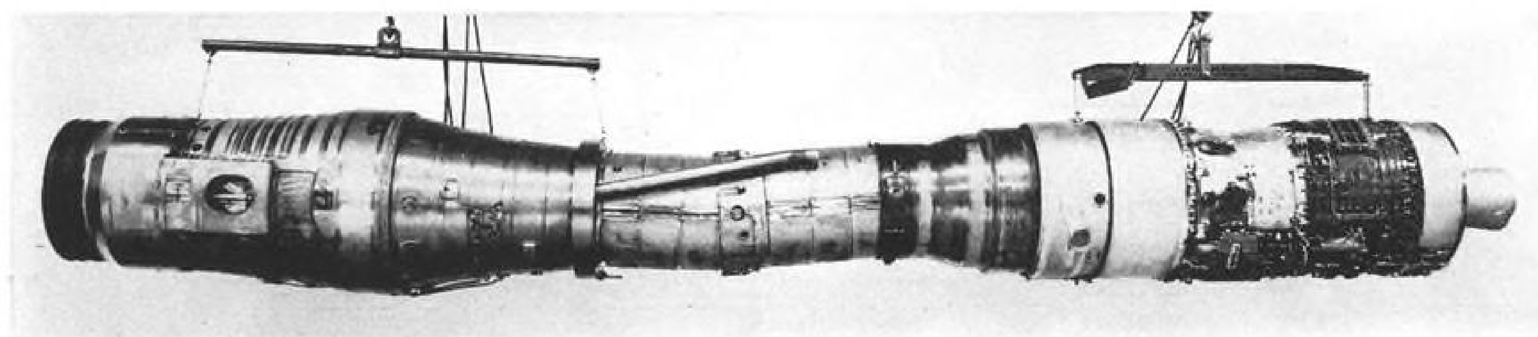
RM-6C POWERPLANT for the Swedish Air Force's J35D Draken interceptor is a modified Rolls-Royce Avon 300 turbojet developing 17,600 lb. thrust with a Swedish-designed afterburner. Middle section is length adapter connecting engine with afterburner.
