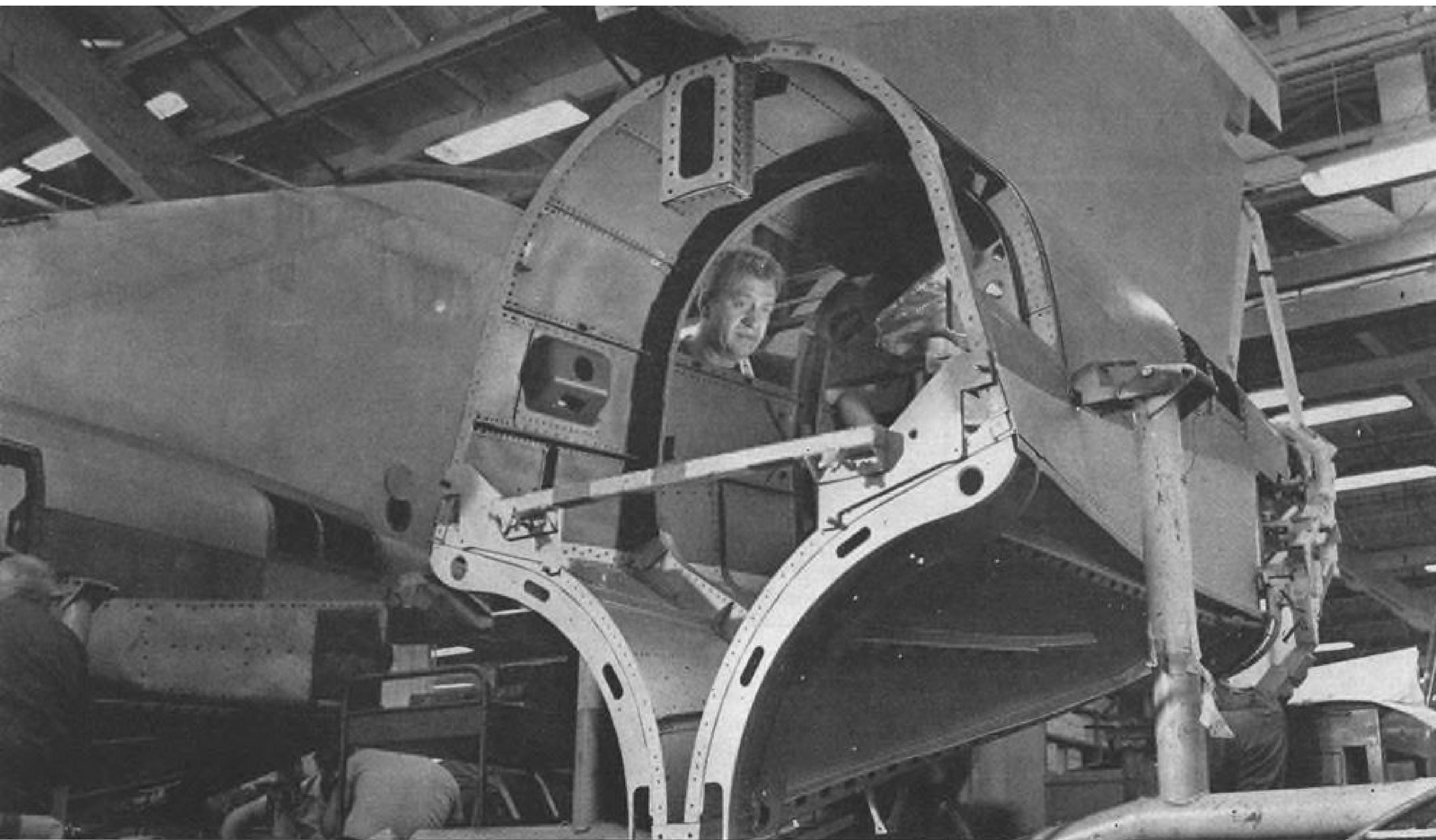
Phantom aft fuselage section (above) and stabilator (below) being assembled at Republic Aviation Corp., under subcontract for McDonnell, are 25% titanium, must withstand jet wake heat.
