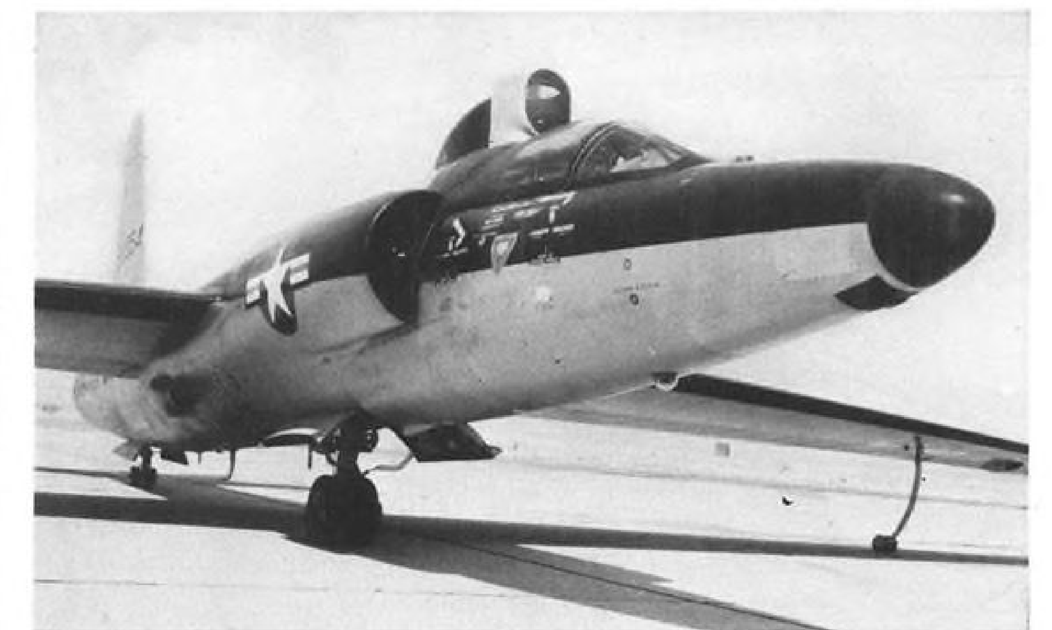
MIRROR SYSTEM FOCUSES radiation from missile launches to instruments mounted in rear seat of monitoring U-2. "Pickel barrel" covers external parts and it has a fastback-type fairing located directly behind it to reduce aerodynamic turbulence.
