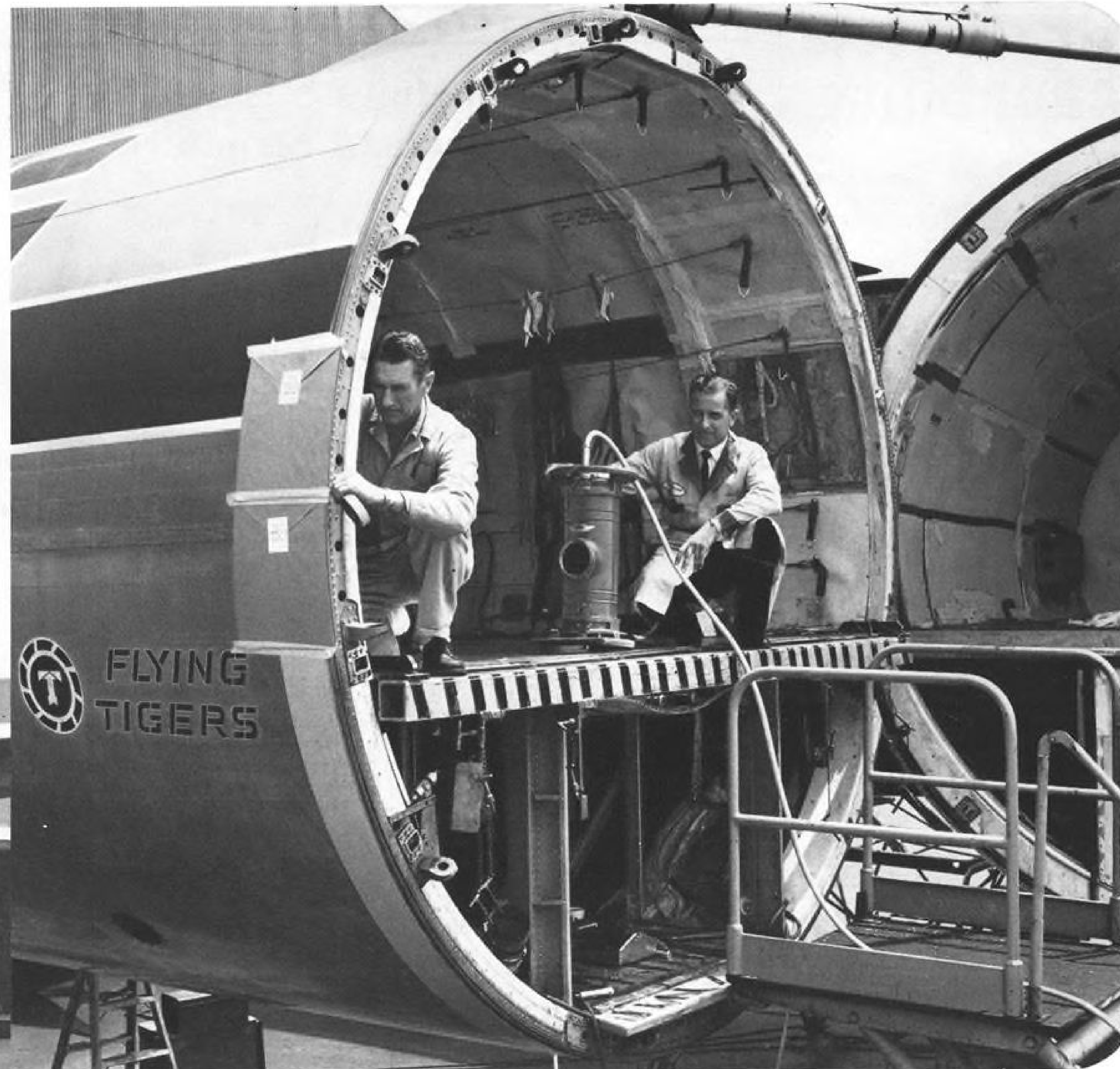
Flying Tiger Line technicians at the line's main base of operations in Los Angeles, Calif., inspect the fuselage break area of one of their famous swingtail air freighters
