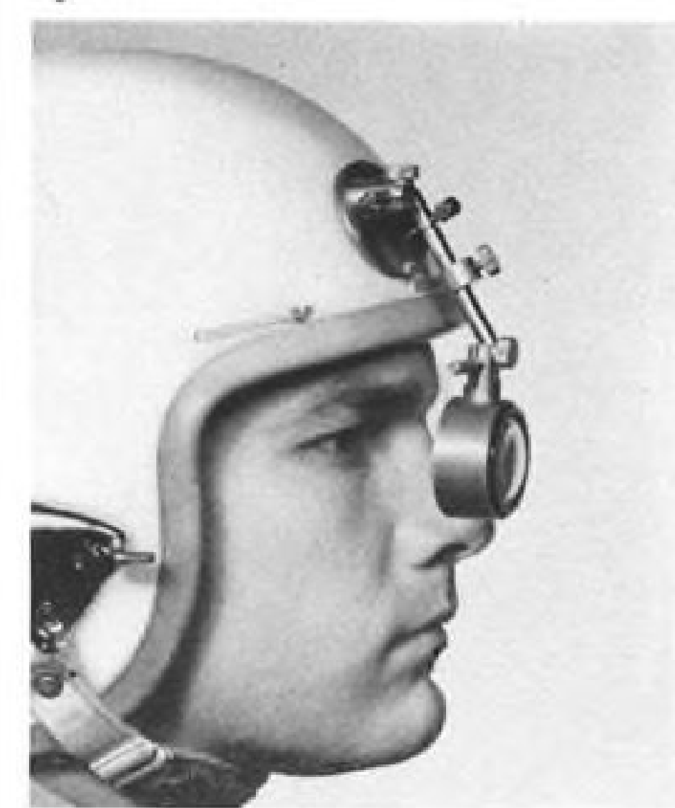
EVALUATION MODEL of helmet-mounted target sighting device is used in human factors studies at Honeywell probing search behavior and predicting the performance level of the human eye while a pilot is flying a low-altitude tactical mission.
