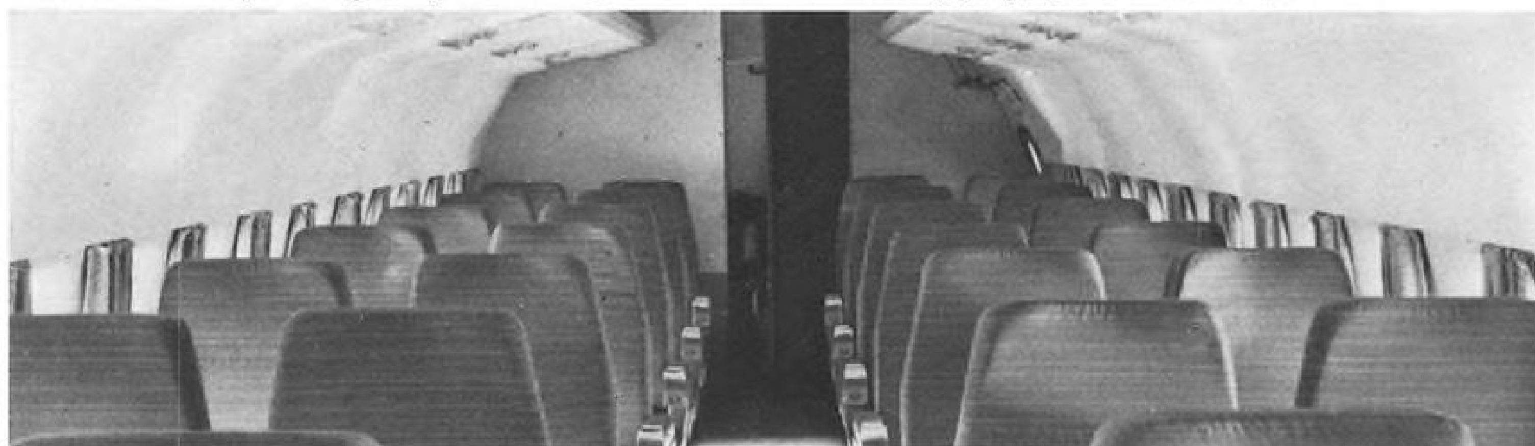
3. Using 34" pitch seats, the YS-11 is capable of carrying 60 passengers.
