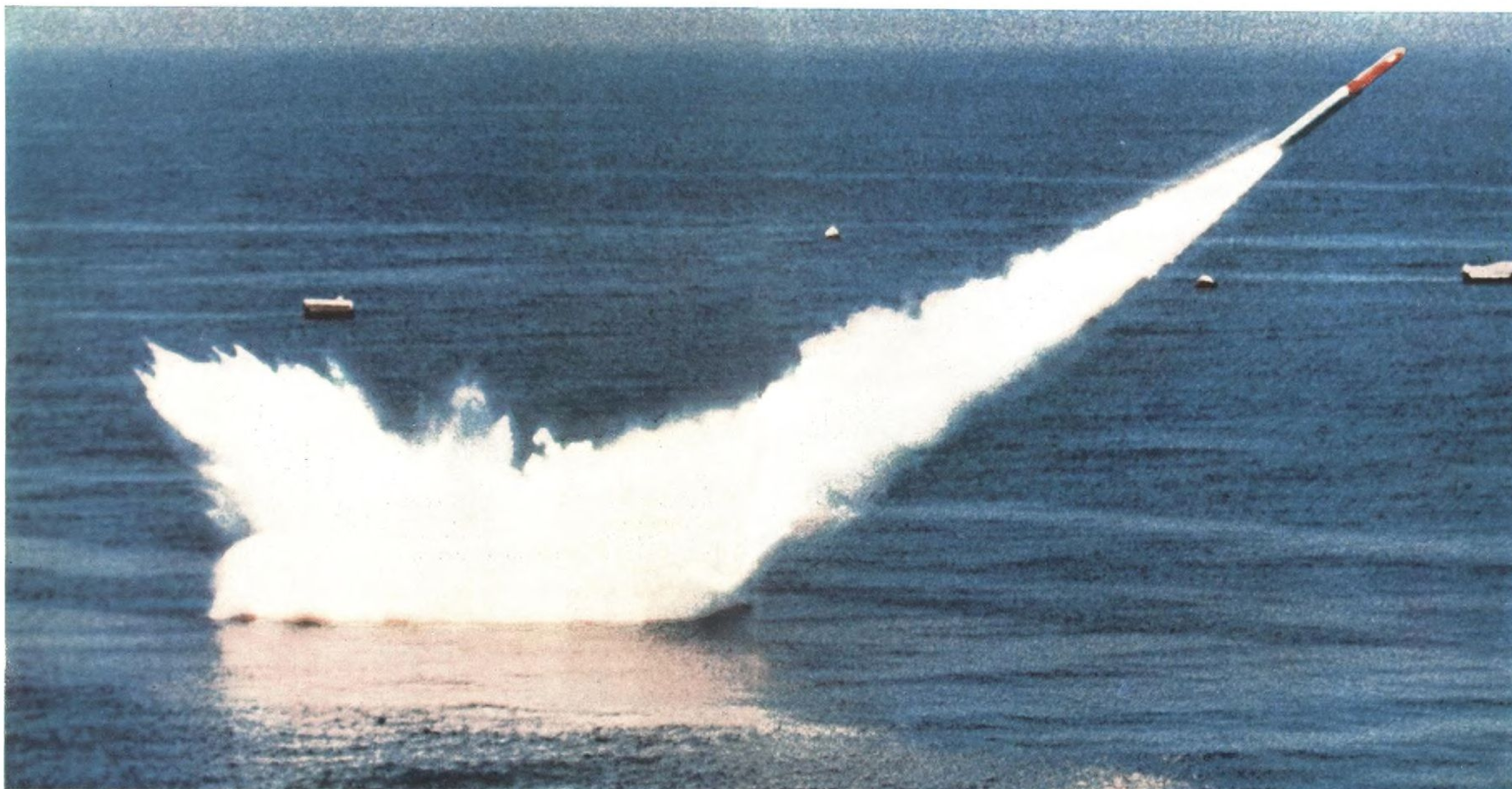
SUBROC antisubmarine missile bursts out of the water and streaks skyward during recent test firings in the Pacific. GAC is prime contractor. SUBROC is launched from a submerged submarine, is designed to kill enemy submarines at long range.
