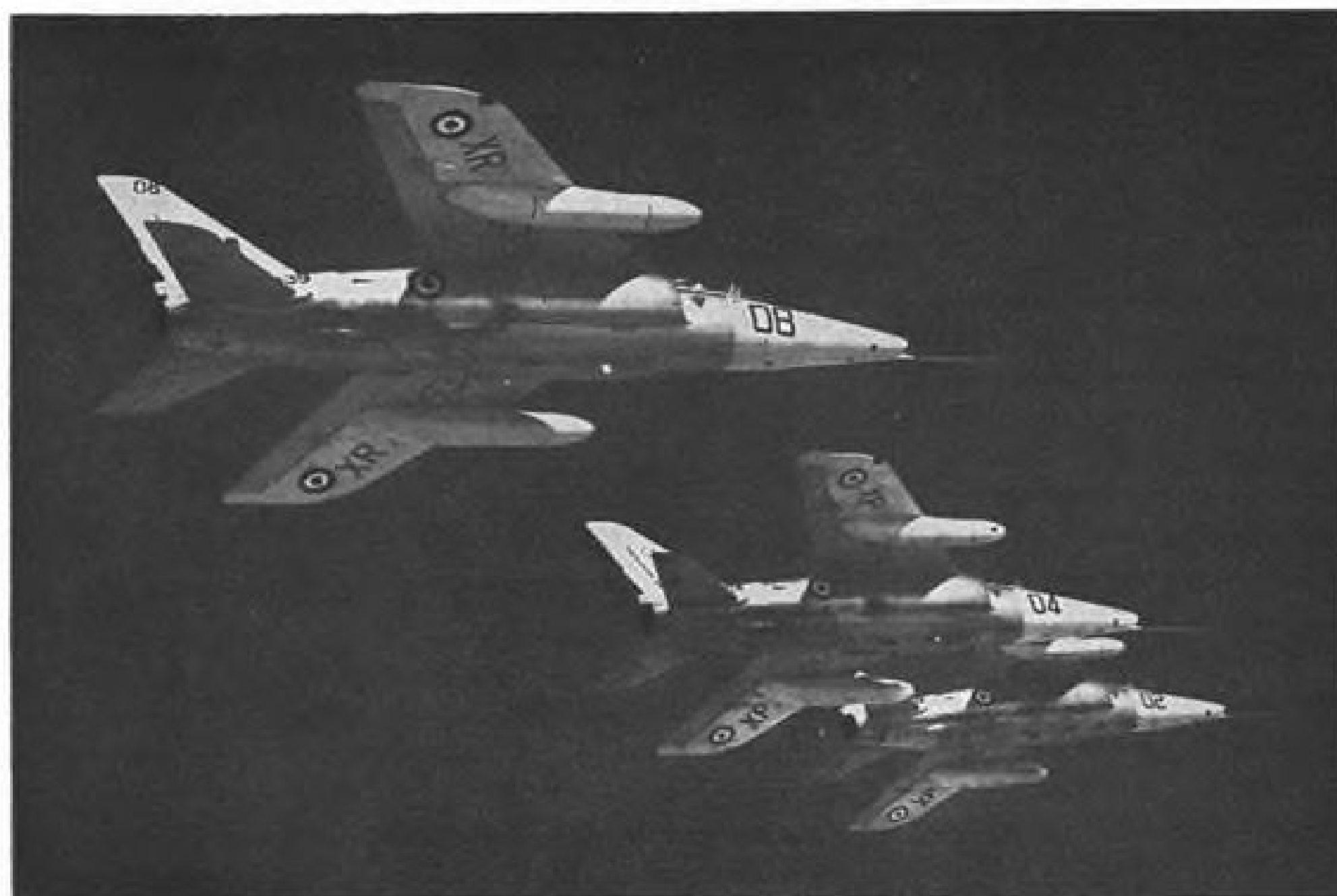
FORMATION OF THREE Hawker Siddeley Gnat trainers, flown by students of Royal Air Force Training Command, shows general arrangement of slipper tanks on the aircraft.
