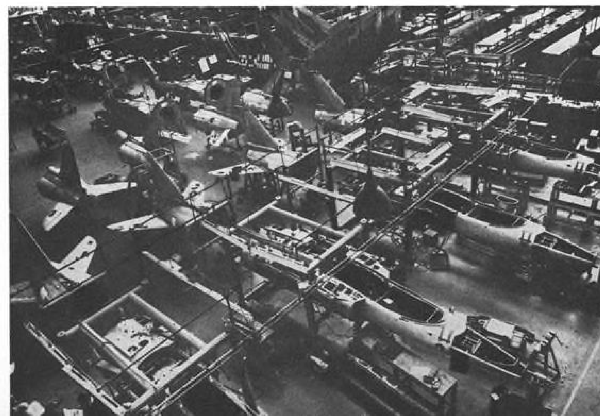
PROMINENT POSITIONING of artificial horizon and navigation display unit is shown in photo of Gnat's front cockpit (above). Warning lights are in strip over the two instruments and below altimeter and airspeed indicators. Relight button is atop the throttle at left. Over-all view of main Gnat production line (below) is shown at Hawker Siddeley's Folland Div. plant. Note complete single-section wings at the top of the photo.
