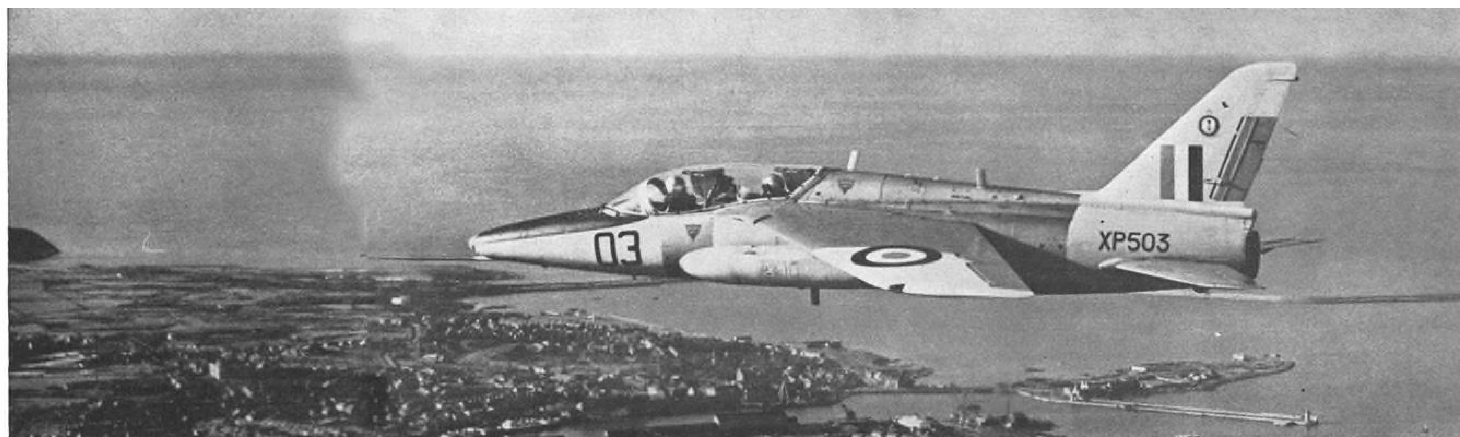
STUDENT PILOT GAINS a high degree of visibility from the front cockpit of the Gnat trainer, as shown above, but visibility is sharply limited in the rear cockpit.
