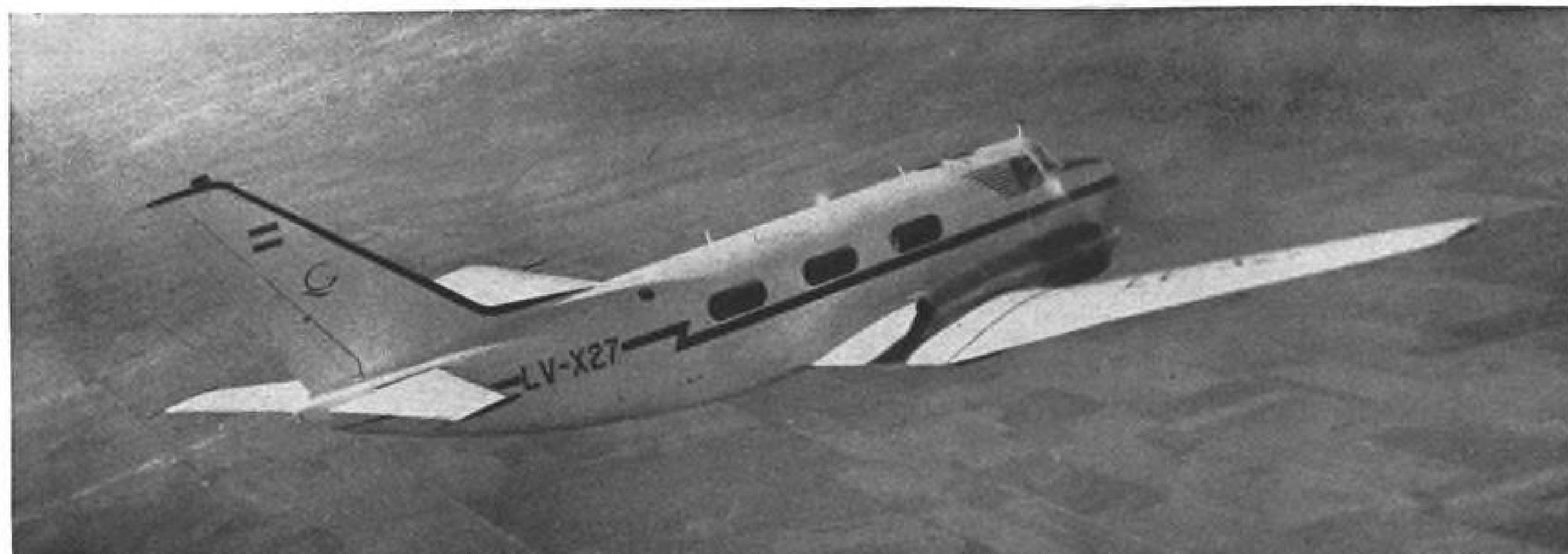
GUARANI 2 PROTOTYPE POWERED by two Turbomeca Bastan 6A turboprop engines made its first flight in April.
