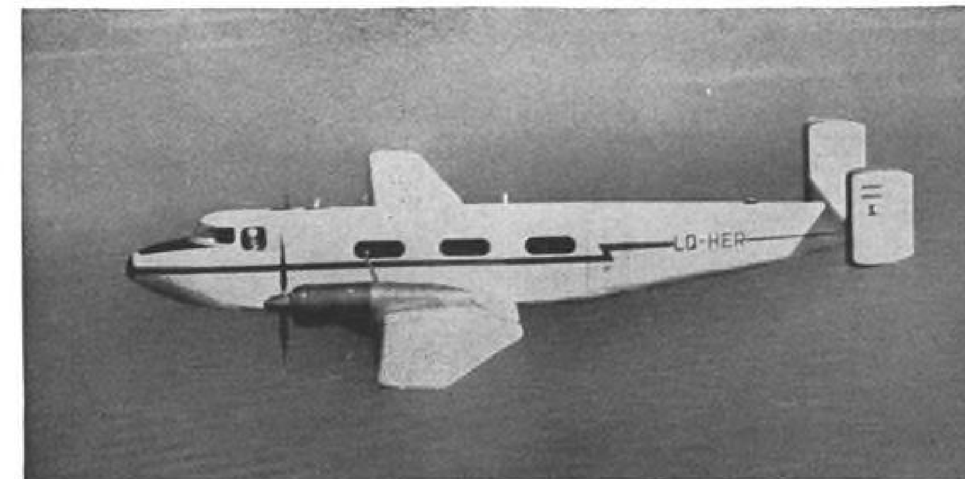
GUARANI 1 PROTOTYPE POWERED by Turbomeca Bastan 3As first flew in February, 1962. Twin fin and rudder of earlier Huanquero were scrapped to improve one-engine stability. Before first test flight, project engineers had completed a mockup of the Guarani 2 incorporating improvements already considered necessary to the first version.
