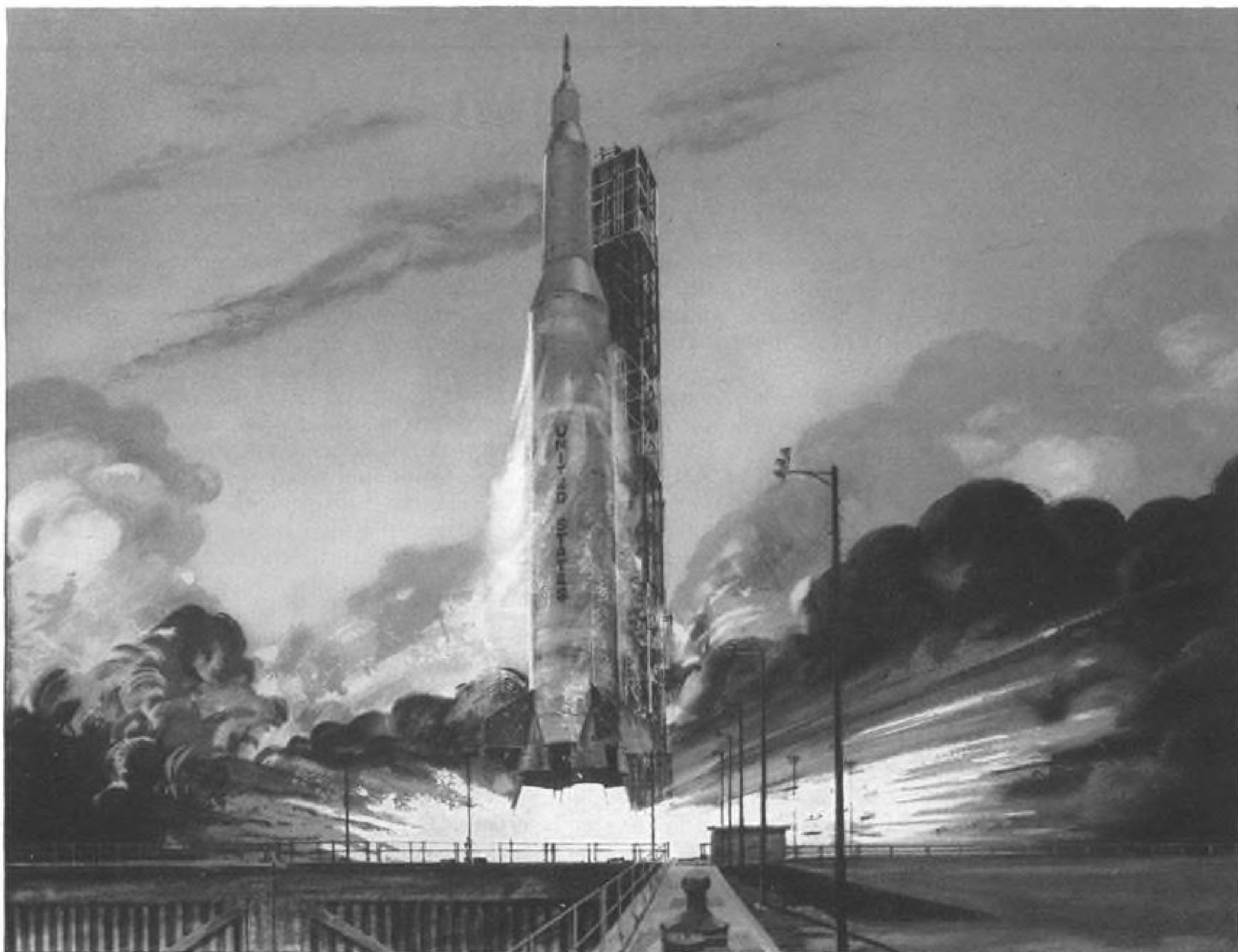
SATURN V , pictured in drawing above, will be the free world's largest rocket, standing tall as a 30-story building and measuring 33 feet in diameter. A National Aeronautics and Space Administration program, Saturn V will be used to launch men and equipment into earth orbit, lunar orbit, moon landings and deep
