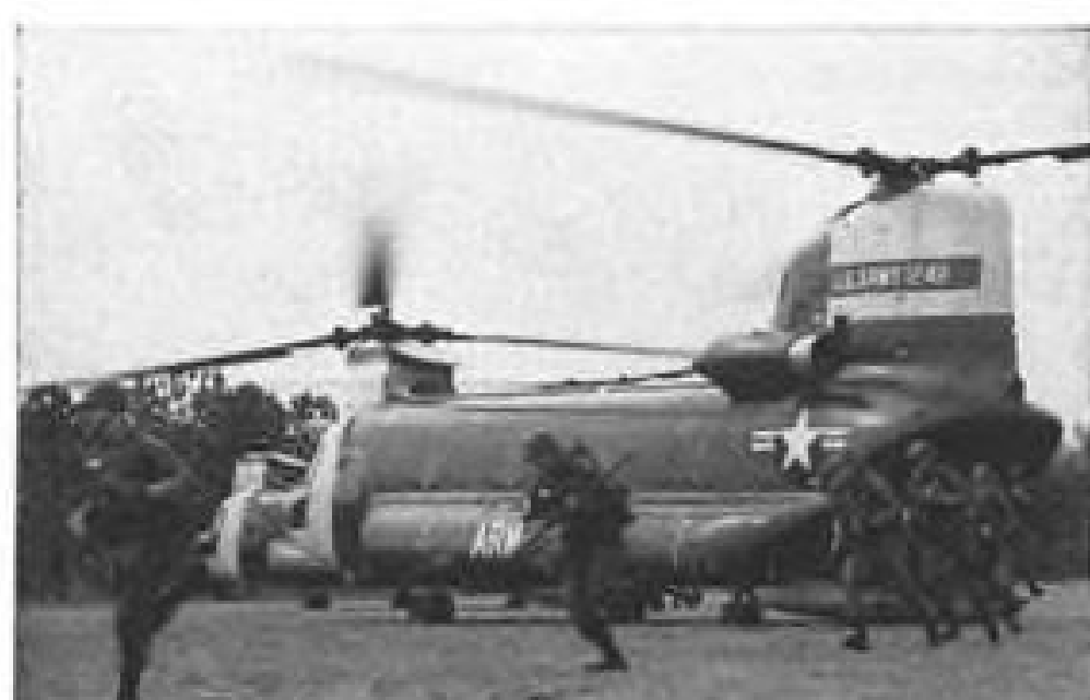
TWIN TURBINE Chinook, new Boeing-Vertol tactical transport helicopter, now in operation with U.S. Army. Chinooks carry 33 fully equipped troops, cruise at 150 mph.
