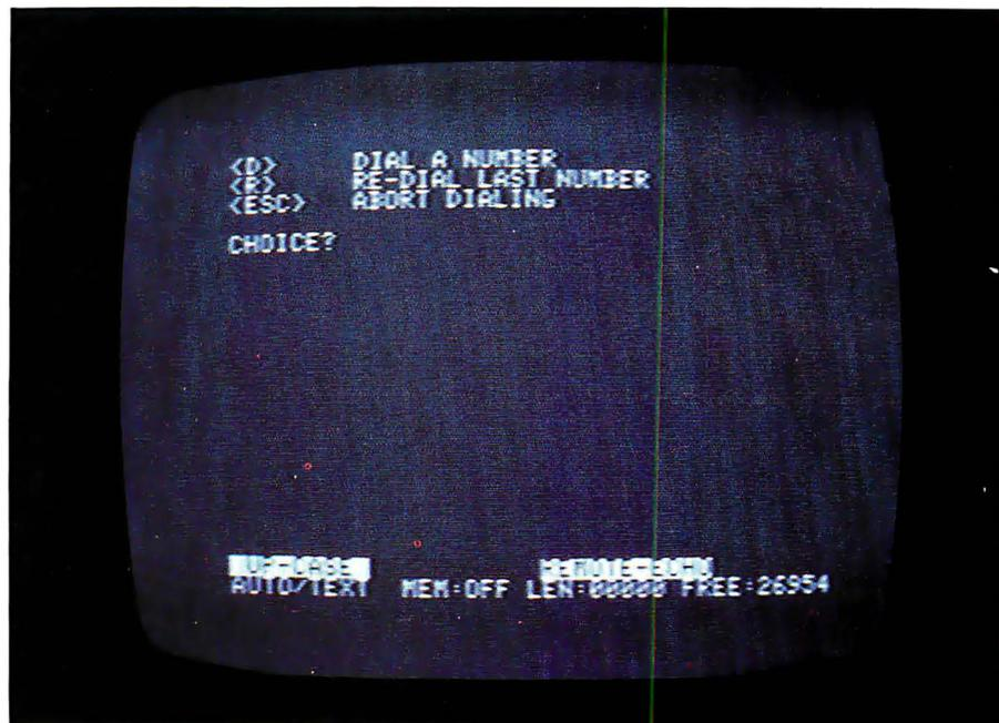
Photo 5: After typing A in the main menu (photo 4), you get this screen, which shows the auto-dial menu. Pressing R now will redial the last number entered. Pressing D will give you the next screen (photo 6).
