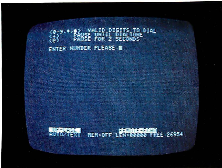
**Photo 6:** Selecting D from the previous screen (photo 5) gives this entry screen for phone numbers. Note that the options include pauses and waiting periods for a second dial tone. Since the Apple-Cat II can dial using either tone or pulse dialing, it can be used with private branch exchanges (PBX) or long-distance services that require tones, such as MCI. Most other modems do not function in both dialing modes.
