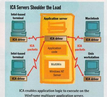
cution (see the figure above). The client doesn't have to be a PC; it can be a Mac or a Unix workstation running suitable client software. Citrix has invented an efficient protocol, called Intelligent Console Architecture (ICA), to send the display commands.
