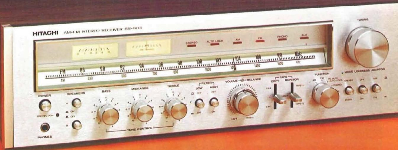
Stereo Review went on to explain that this exclusive circuitry "uses...a low power and a high power output stage operating together... At low signal levels the lower power stage drives the speakers. The transition to the more powerful output transistors...takes place smoothly at the point where it becomes advantageous to do so."
