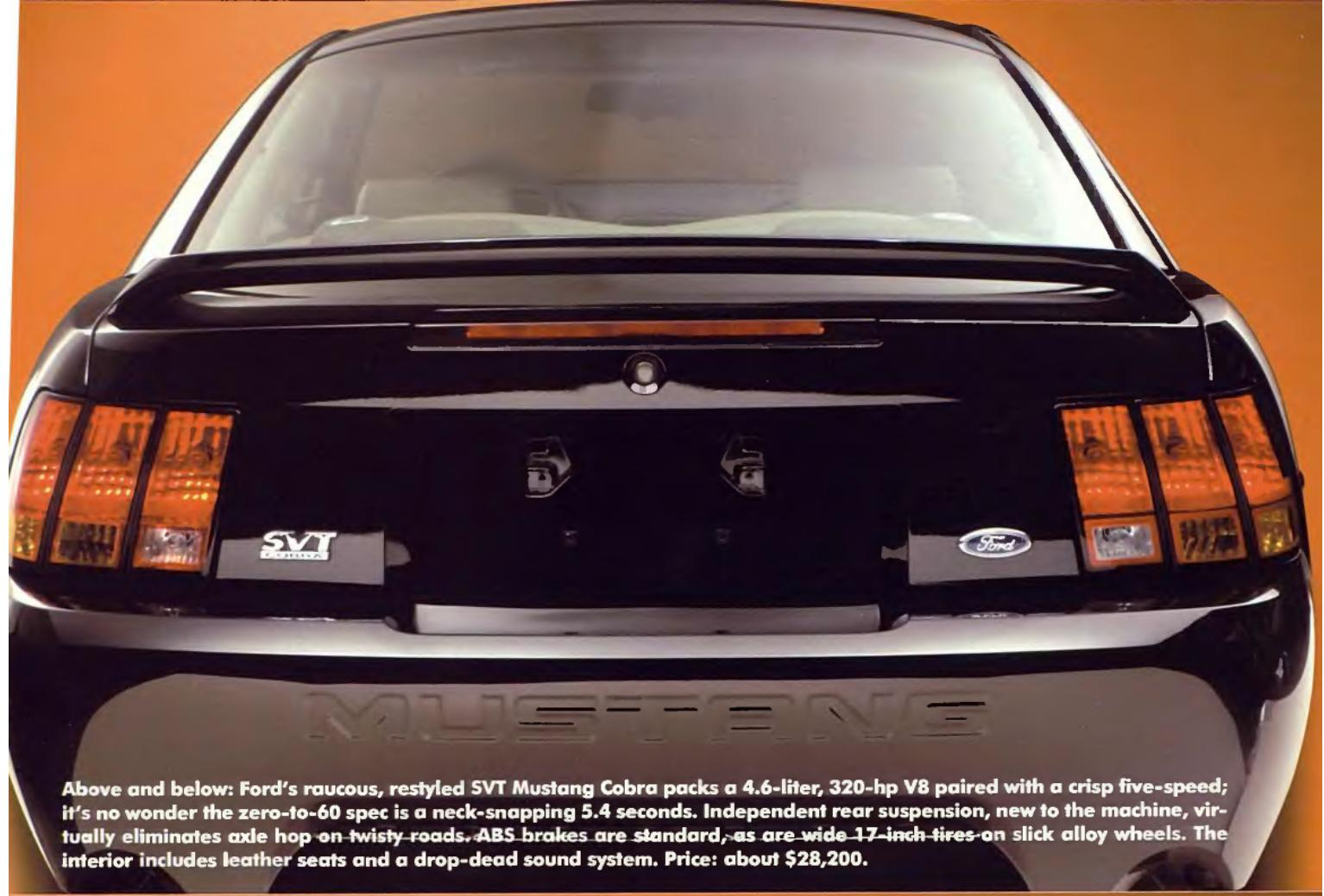
Above and below: Ford's raucous, restyled SVT Mustang Cobra packs a 4.6-liter, 320-hp V8 paired with a crisp five-speed; it's no wonder the zero-to-60 spec is a neck-snapping 5.4 seconds. Independent rear suspension, new to the machine, virtually eliminates axle hop on twisty roads. ABS brakes are standard, as are wide 17-inch tires on slick alloy wheels. The interior includes leather seats and a drop-dead sound system. Price: about \$28,200.
