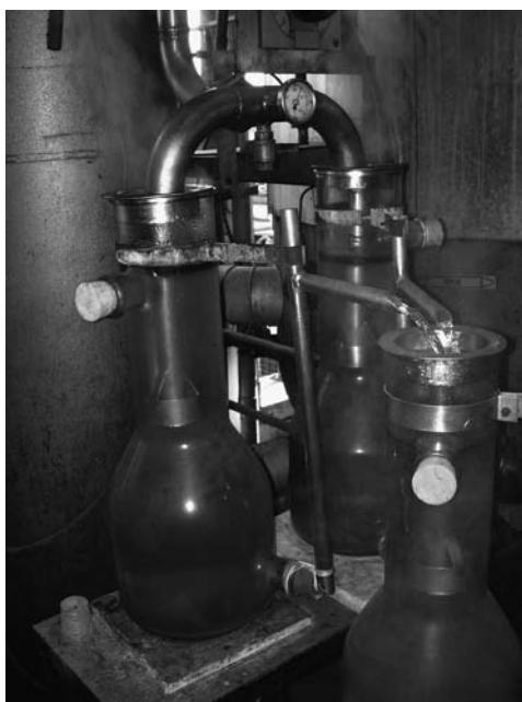
FIGURE 4.19 Orris distillation, Florentine flask at nearly 98°C.
