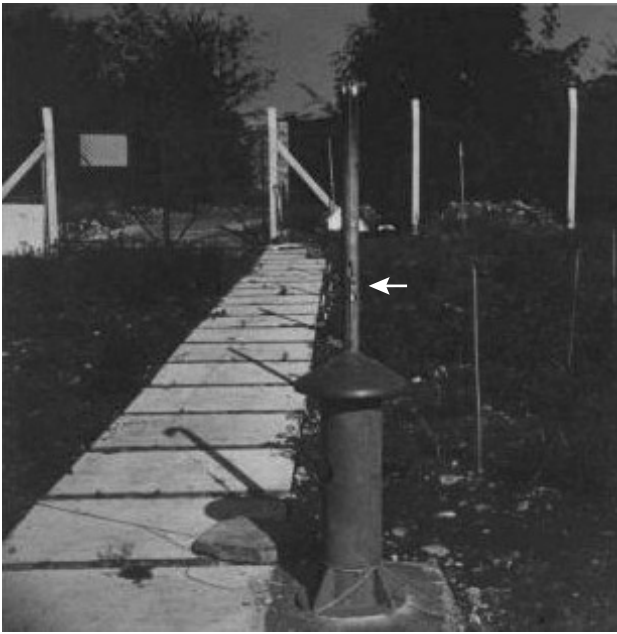
Figure 5.3 A radiation device (installation) with the special raising mechanism for irradiating the source, in operation.
