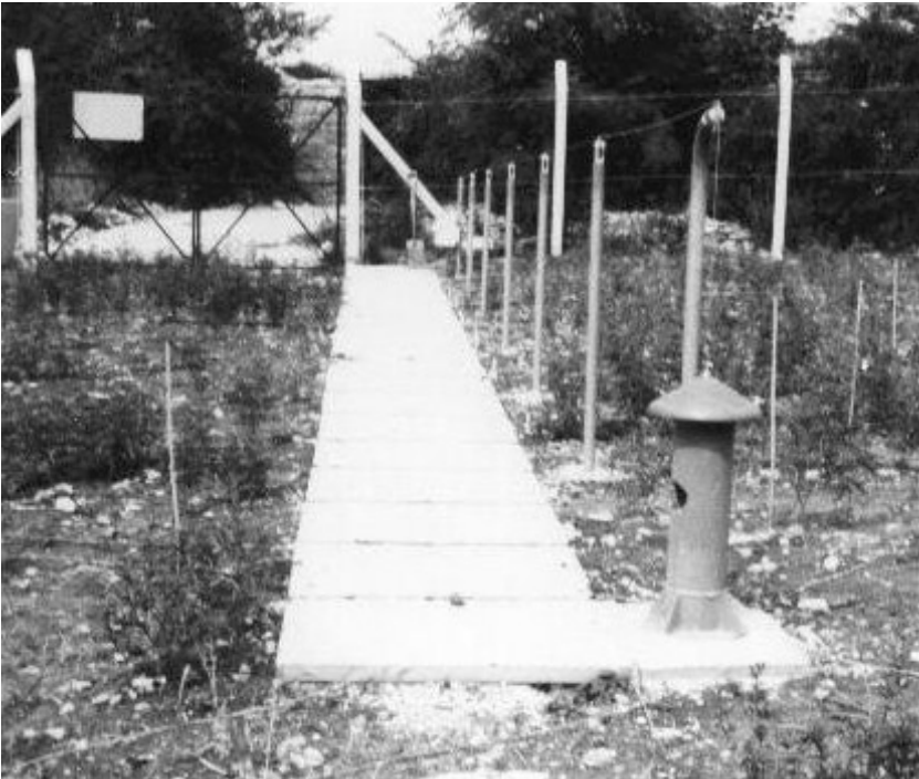
Figure 5.4 The same device with the special mechanism to lower the source into its protective lead shield, during visits to the experimental area.
