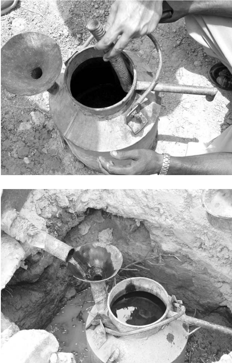
FIGURE 6.8 The converted milk can receiver (oil separator) used in India.
