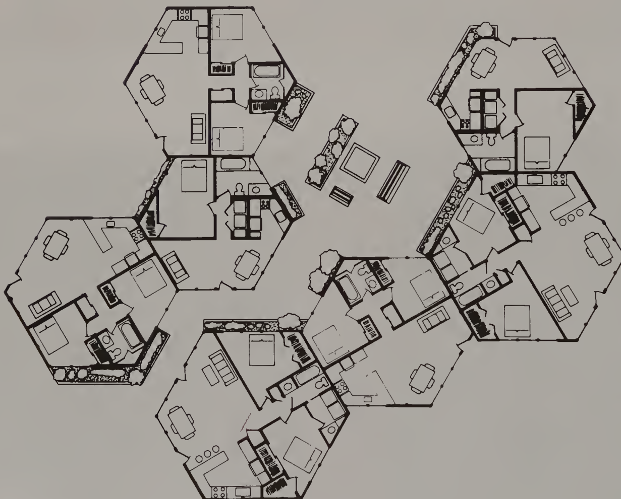
Fig. 1-25. Architectural plan for multi-unit complex using prefabricated "HEXAN" hexagonal shell units
