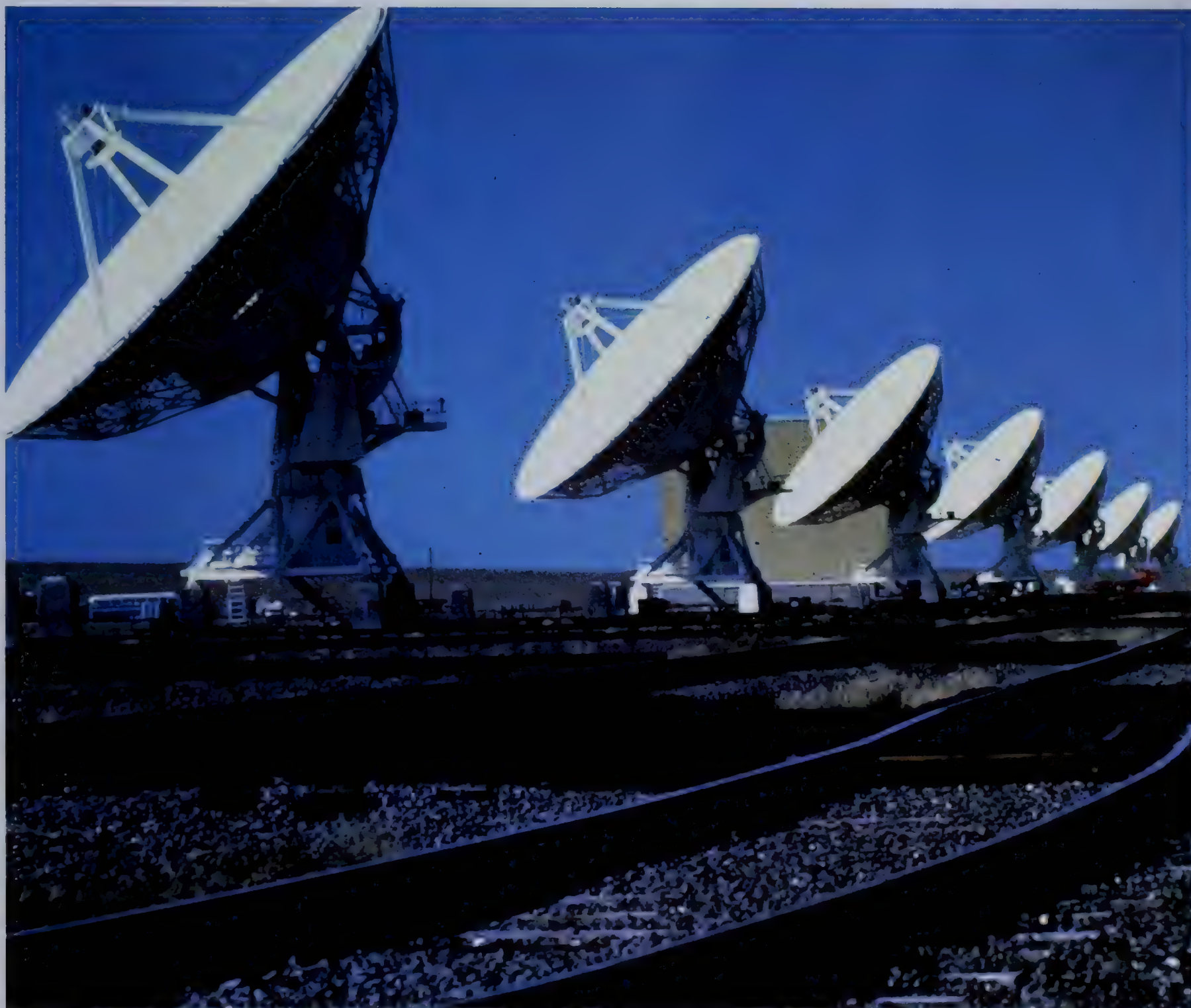
8.15 A few of the radio dishes that make up the Very Large Array, located in New Mexico. Working in harmony, these radio telescopes can record emission from celestial sources with very high resolution.
