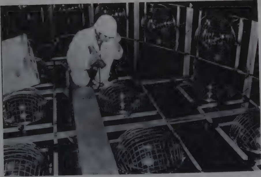
FIGURE 66: A graduate student at the University of Tokyo examining the photomultiplier tubes in the tank of the Kamiokande neutrino detector. When the detector is operating, the entire cylindrical tank, 16 meters high and 16 meters in diameter, is filled with water. The photomultipliers detect light produced by particles passing through the tank. (University of Tokyo-Kamiokande.)
