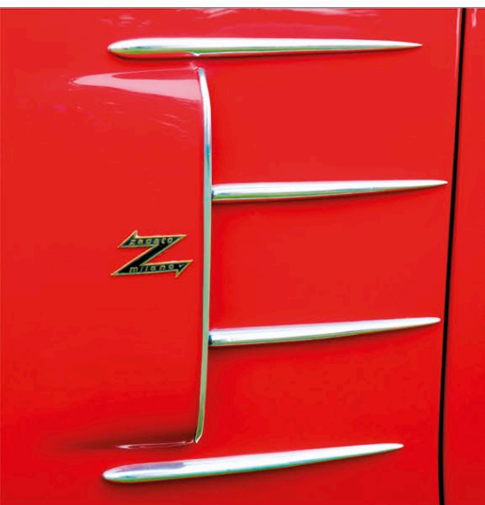
COOLING VENT, MASERATI-A6G 1953
