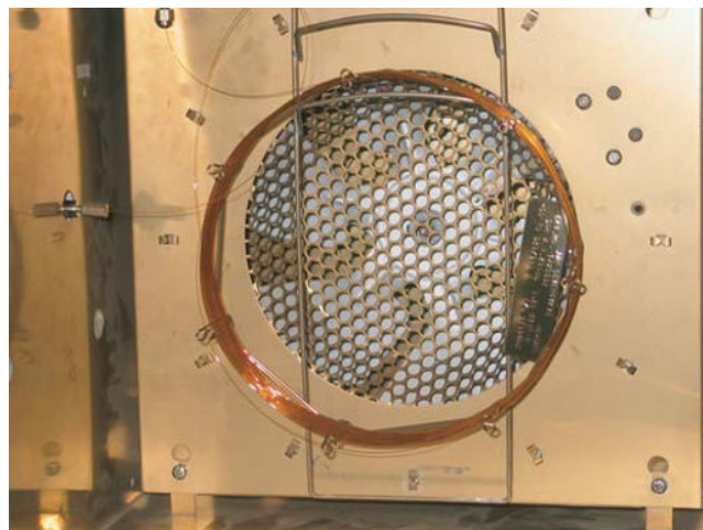
FIGURE 25.23 Close up view of column in GC oven. Notice the two connections of the column including the top left into the injection port, and the middle left where the column is connected to the detector.
