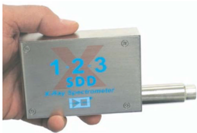
FIGURE 20.4 Example of a Peltier-cooled silicon drift detector (SDD). (Reprinted with permission from Amptek Inc.)
