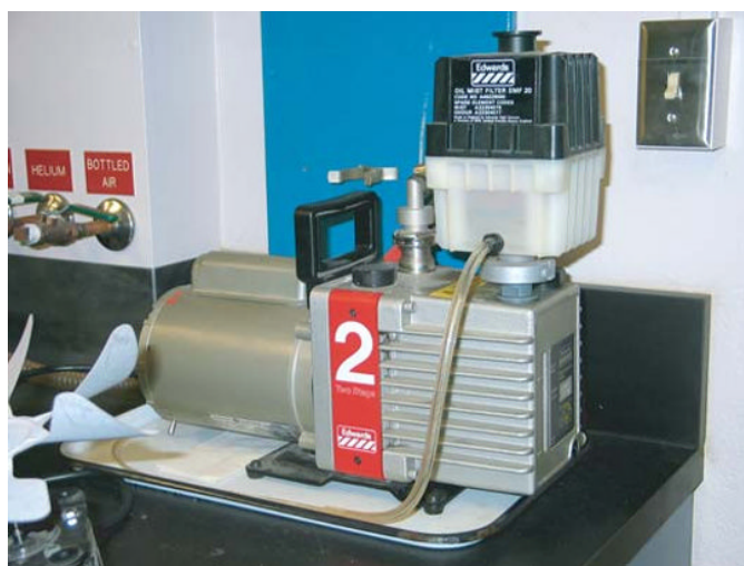
FIGURE 2.27 Examples of laboratory vacuum pumps.
