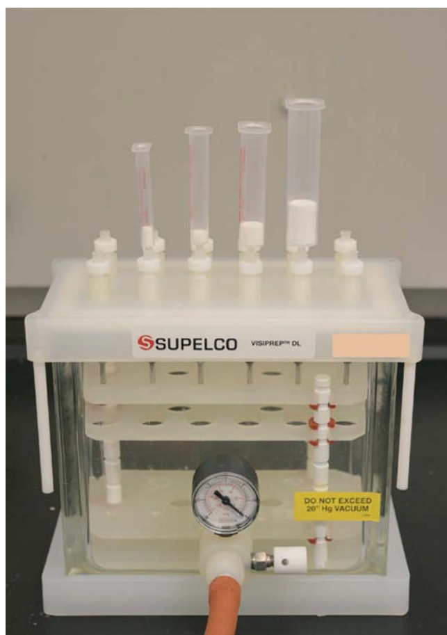
FIGURE 23.2 Solid phase extraction (SPE) vacuum manifold. Six SPE tubes are positioned on the manifold. SPE tube flow controlled by small hand turn valves under the tubes and either the flow-through wash/waste or the eluting compounds are collected in glass test tubes placed inside the manifold and under the SPE tubes. At the bottom right is located an inlet fitting for connection of a vacuum source usually also consisting of a control valve and a pressure gauge.
