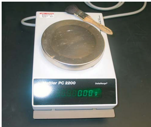
FIGURE 2.22 A top loading balance used for larger amounts of the item to be weighed. Also used when the precision of an analytical balance is not necessary.
