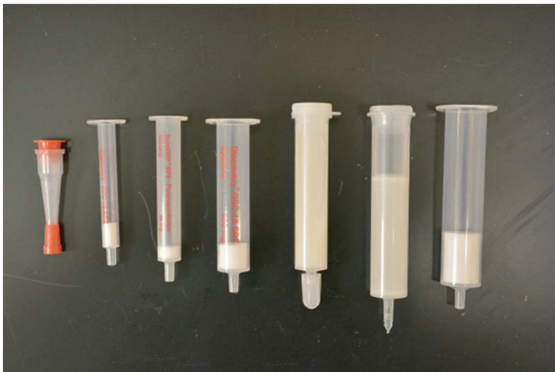
FIGURE 23.1 Examples of solid phase extraction (SPE) cartridges used in the analytical laboratory.
