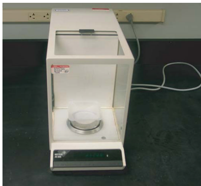
FIGURE 2.21 Examples of analytical balances. Used for precise weighing of amounts up to approximately 220–260 g depending upon the make of the balance.
