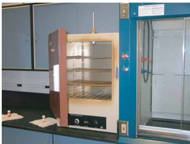
FIGURE 2.20 A drying oven located to the left of the laboratory fume hood. These are lower-temperature ovens with temperatures ranging from 40 to 220 °C.
