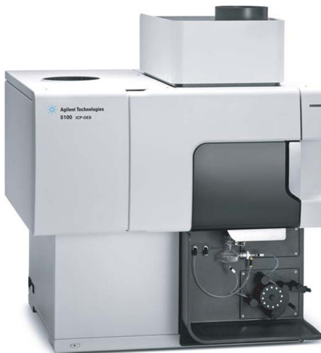
FIGURE 18.8 The Agilent 5100 ICP-OES instrument. (© Agilent Technologies, Inc. 2014, Reproduced with Permission, Courtesy of Agilent Technologies, Inc.)
