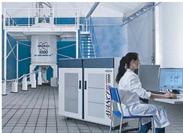
FIGURE 16.5 Bruker AVANCE 1000 MHz (23.3 T) NMR spectrometer. (Reprinted with permission from Bruker BioSpin.)
