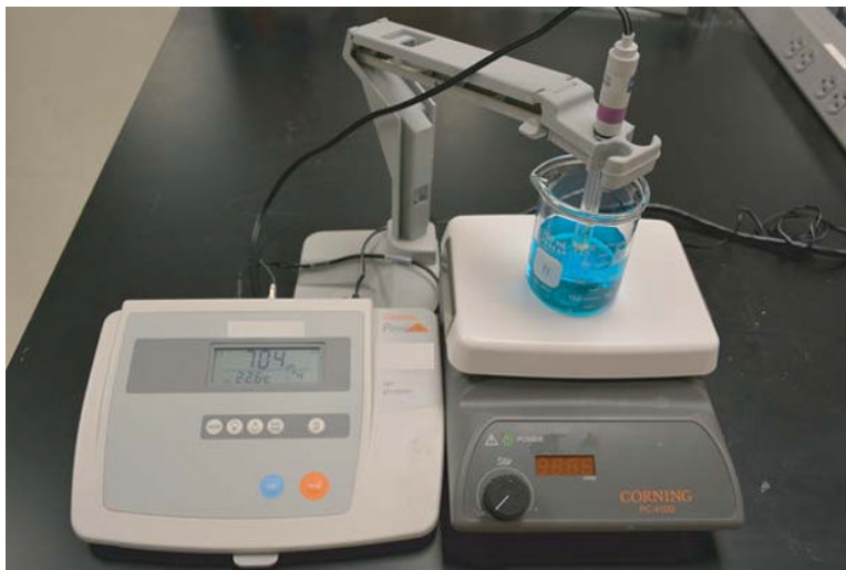
FIGURE 9.5 Example of a bench top pH meter including LCD readout and pH electrode.
