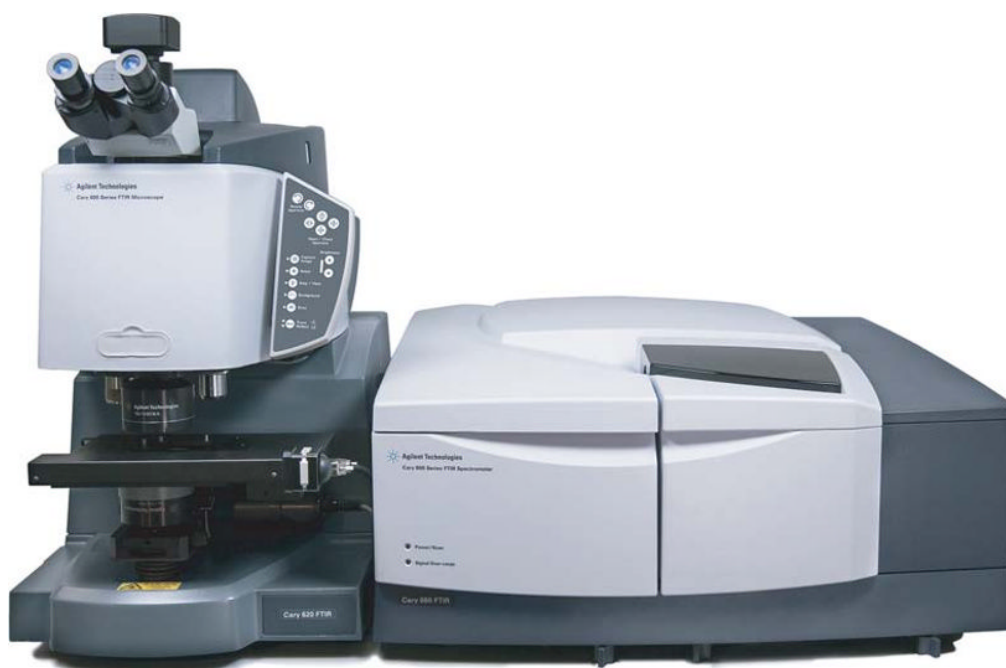
FIGURE 15.6 Agilent Cary 620 spectrochemical imaging system where the FTIR instrument has been coupled to a microscope. (© Agilent Technologies, Inc. 2014, Reproduced with Permission, Courtesy of Agilent Technologies, Inc.)
