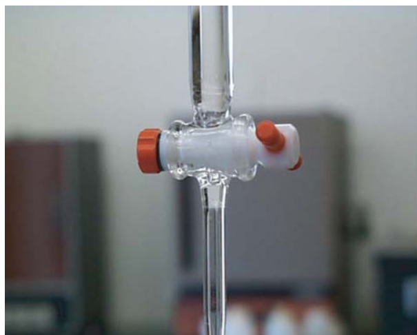
FIGURE 10.12 Titration burette stopcock.
