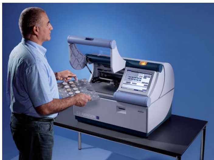
FIGURE 20.8 Bruker S2 Ranger EDXRF spectrometer. (Reprinted with permission from Bruker AXS Inc.)
