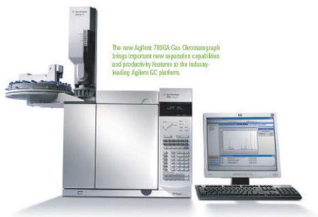
FIGURE 25.8 (a) A Hewlett Packard (HP) 5890 Series GC. (b) The latest generation of this series of GC's called the Agilent (spun-off company from HP) 7890A Series GC.
