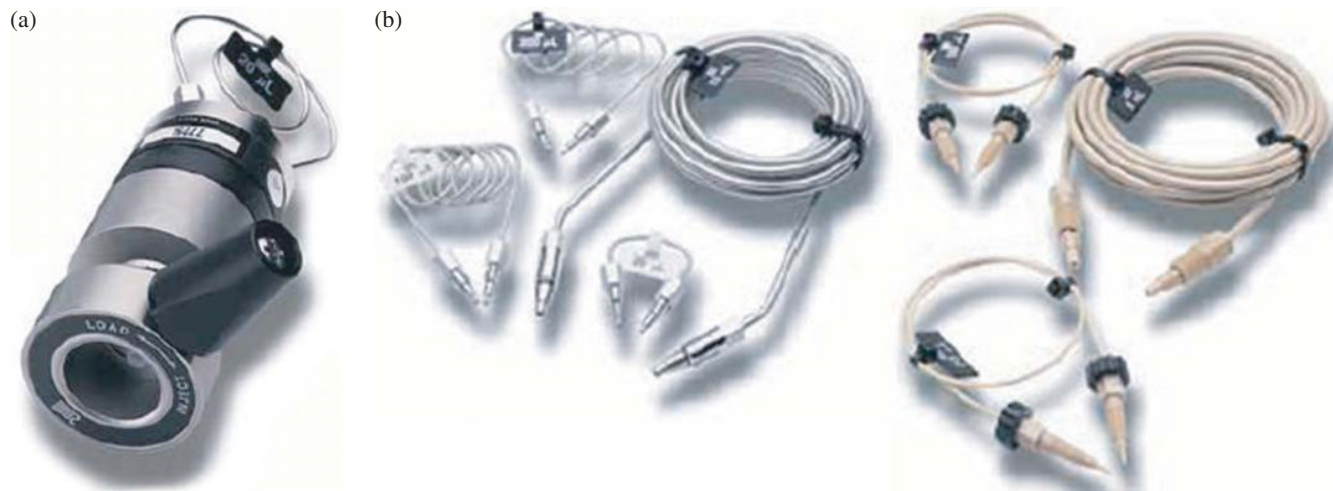
FIGURE 22.5 (a) Close up view of the Rheodyne injection valve. Located in the back of the injection valve is a sample loop. (b) Examples of different volumes of sample injection loops.
