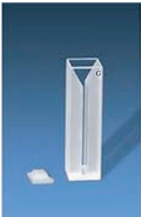
FIGURE 13.20 Micro quartz cuvette cell with 1 cm path length and a volume of 1.4 ml.
