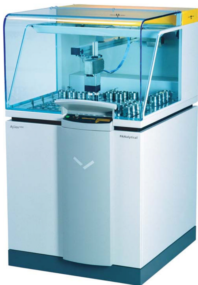
FIGURE 20.16 The PANalytical AXIOS mAX sequential WDXRF spectrometer. (Image courtesy of PANalytical.)
