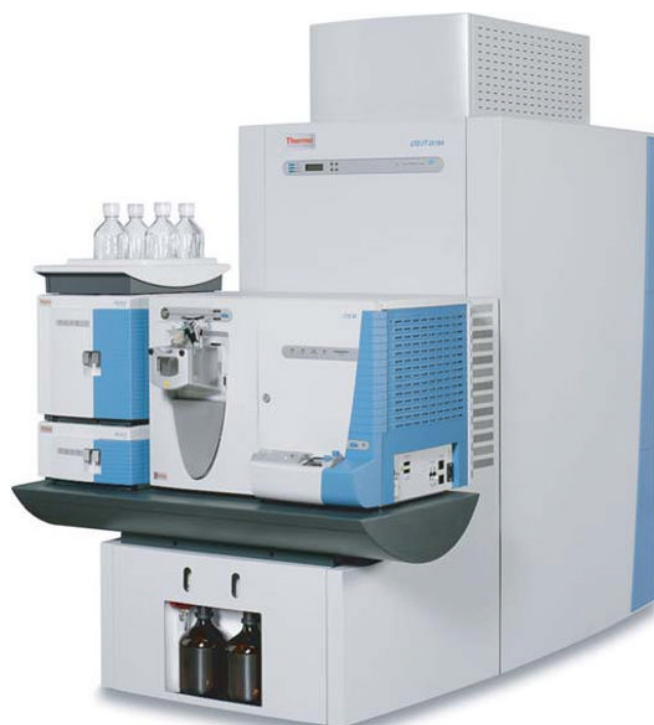
FIGURE 30.40 Picture of the LTQ-FT Ultra TM mass spectrometer. (Reprinted with permission from Ref. [12]. Copyright 2004 American Chemical Society.)
