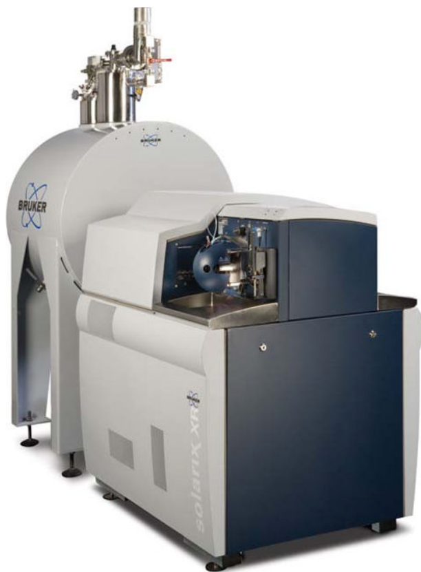
FIGURE 30.26 A Bruker Daltonics solariX XR Fourier transform ion cyclotron resonance mass spectrometer (FTICR/MS). The large circular portion of the mass spectrometer is the shielded magnet, which comes in 7.0, 9.4, 12, or even 15 T magnets that are actively shielded. The ion cyclotron cell is located within the central bore of the magnet. The front, right portion of the mass spectrometer houses an inlet source and a trapping quadrupole for ion accumulation prior to entry into the ICR cell. (Reprinted with permission from Bruker Daltonics.)
