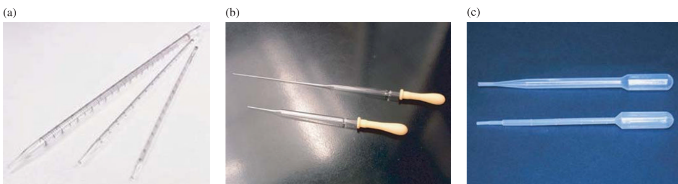
FIGURE 2.9 Examples of common disposable pipettes. (a) Serological pipettes that are “to contain, TC,” (b) glass Pasteur pipettes and their bulbs, and (c) plastic transfer pipettes.
