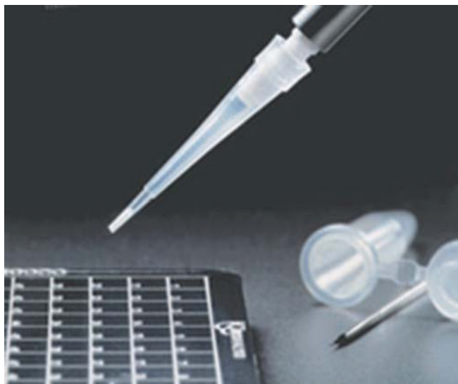
FIGURE 29.22 Spotting of a MALDI target plate. (Courtesy of EMD Millipore Corporation, Billerica, MA.)
