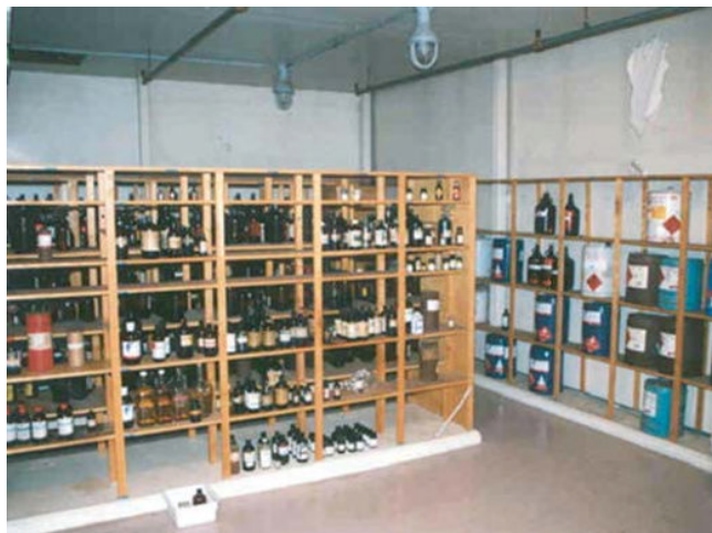
FIGURE 3.14 Storage of chemicals on wooden shelves. Are any chemicals stored here oxidizers? Note the flammable liquid loading on the right. This shelving arrangement would not last should a fire occur even with fire sprinkler activation. (Reprinted from Journal of Chemical Health and Safety , 15(2), Fred Simmons, David Quigley, Helena Whyte, Janeen Robertson, David Freshwater, Lydia Boada-Clista, J.C. Laul, Chemical storage: Myths vs. reality , 23–30, Copyright (2008), with permission from Elsevier.)
