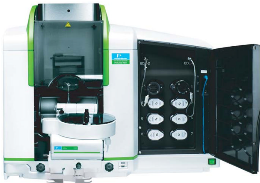
FIGURE 17.13 The PinAAcle™ 900 lamp compartment that holds the hollow cathode lamps for metals analysis. (Reprinted with permission from PerkinElmer).
