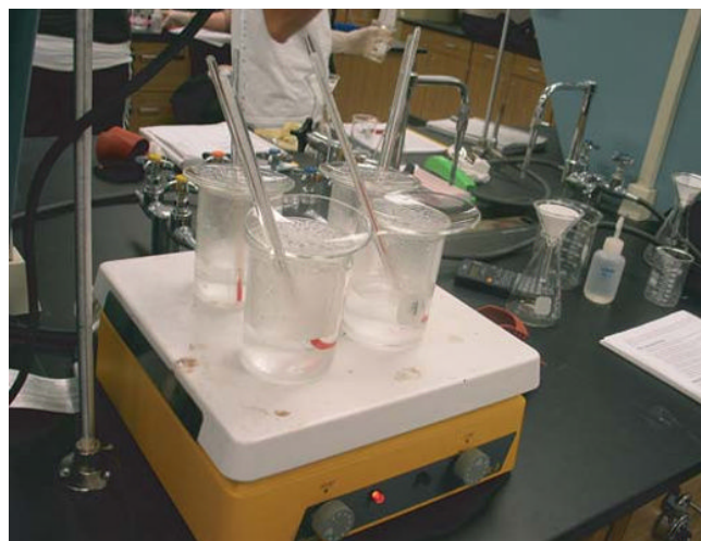
FIGURE 2.12 Example of the use of watch glasses being used to cover beakers being heated on a hot plate.
