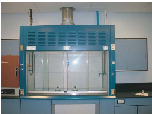
FIGURE 2.19 An example of a common laboratory hood. The compartment is positive vented at the top. A blower is connected to the vent pipe at the top of the hood.
