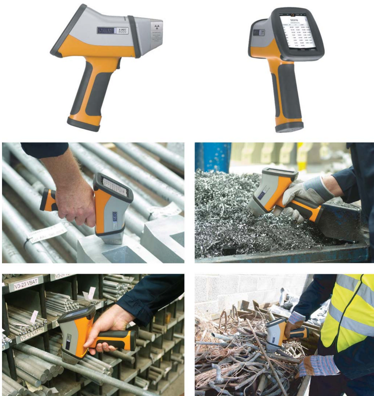
FIGURE 20.10 A hand held X-MET8000 series EDXRF from Oxford Instruments. Examples of field applications using the portable XRF. (Reprinted with permission from Oxford Instruments.)
