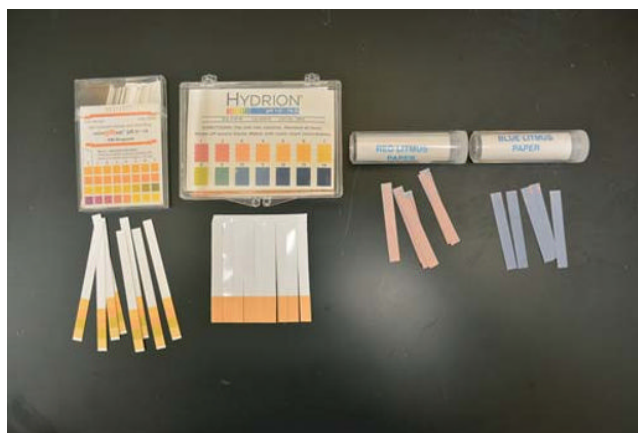
FIGURE 9.2 Examples of commercially available pH test strips and pH indicator papers. Some test strips cover the entire pH range from 1 to 14.
