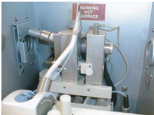
FIGURE 17.10 Graphite furnace sample introduction system. The robotic arm holds a sample introduction tube that is inserted in the middle hole of the graphite tube where the sample is introduced.
