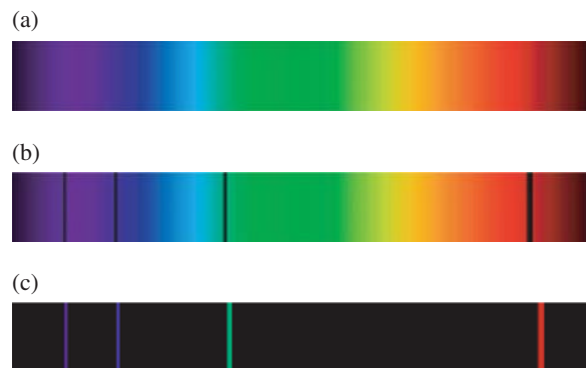
FIGURE 17.2 Spectra representing (a) a continuous spectrum, (b) atomic absorption spectrum, and (c) atomic emission spectrum.
