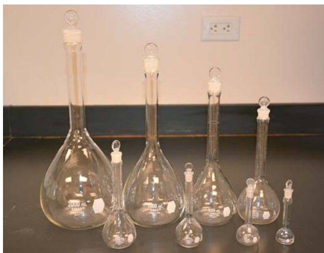
FIGURE 2.2 Examples of volumetric flasks including 100, 250, 500, and 1000 ml sizes.
