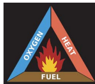
FIGURE 3.8 The fire triangle listing the three elements required for a fire, fuel, oxygen, and temperature.
