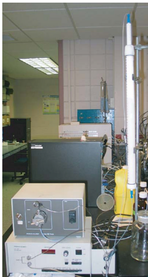
FIGURE 21.4 Column chromatography system example used in the laboratory. The column for the chromatography is the white column located in the right side of the figure. A sample is introduced into the system through an injection valve and sample loop. The injection valve and sample loop are in line with the column through a liquid pump, the top instrument box shown in the figure. The pump flows the injected sample onto the top of the column using the mobile phase. The sample passes through the column where the analytes are separated due to their partitioning coefficients, and are eluted out of the bottom of the column. The bottom of the column has tubing that connects the liquid flow to a UV/Vis detector that is the bottom instrument box in the figure. The separated analytes move through the detector, are measured, and result in a chromatogram such as that illustrated in Figure 21.3.
