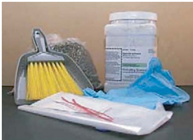
FIGURE 3.12 Example of spill cleanup kit with a scoop and brush used for sweeping up spills that have been treated with a spill agent.
