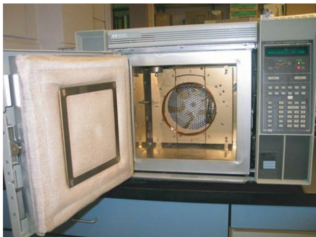
FIGURE 25.22 The gas chromatograph GC oven housing the GC column.
