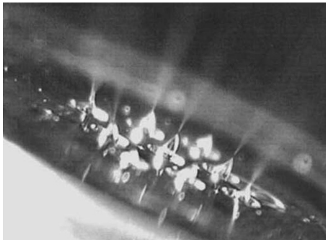
FIGURE 29.13 Photograph of nine stable electrosprays generated from the nine-spray emitter array. (Reprinted with permission from Ref. [29]. Copyright 2001 American Chemical Society.)
