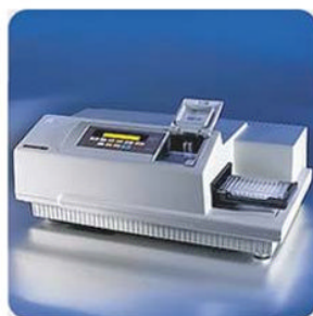
FIGURE 14.13 The SpectraMax M2 microplate reader and 96 well plate. (Reprinted with permission from Molecular Devices, Inc.)
