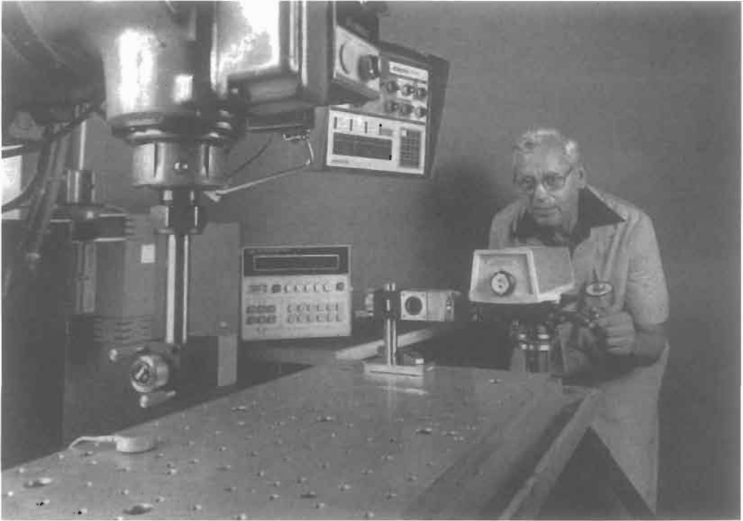
Figure 3.5 Laser interferometer being used to measure length in an industrial application. Courtesy, Agilent, Inc.
