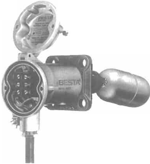
Figure 5.5 Repulsion of like magnetic poles providing non-immersed sensing and toggle action to a float sensor. One commercial form. Courtesy, BESTA Ltd.
