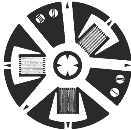
Figure 4.7 Array of gauges for measuring residual stress. Courtesy, Micro-Measurements Division, Measurements Group Inc.
