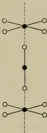
FIG. 9.8. Structure of \text{Cs}_2\text{Au}_2\text{Cl}_6 . \bullet = Au; \circ = Cl.
