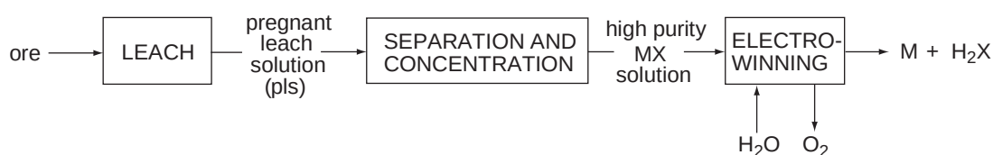
Figure 3 A simplified flowsheet for the hydrometallurgical recovery of base metals using metal complexing agents.
