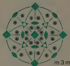
Fig. 15.3 Stereographic projection of the point group m\bar{3}m . Note the triad axes at 55^\circ to the tetrads.
