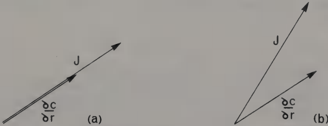
Fig 11.1 The relationship of the resultant flux \mathbf{J} to the applied concentration gradient \partial c/\partial r for diffusion in (a) a polycrystalline solid, (b) an anisotropic single crystal.
