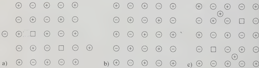
Fig. 13.1 a–c. Schottky defects (a) and Frenkel defects (c) in an ionic crystal ( \square void); (b) the ideal crystal
