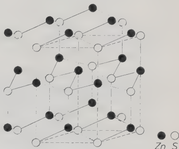
Fig. 11.14. Zn^{[4]}S -structure (wurtzite). Space group P6_3mc Lattice: hexagonal P Basis: S at 0, 0, 0; \frac{2}{3}, \frac{1}{3}, \frac{1}{2} ; Zn at 0, 0, \frac{1}{2} - z; \frac{2}{3}, \frac{1}{3}, z ( z \approx \frac{1}{8} )
