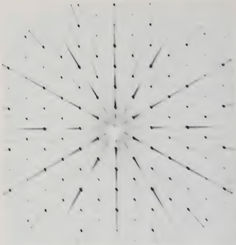
Fig. 12.12. Precession photograph of \beta -eucryptite, \text{LiAlSiO}_4 (space group P6_422 ): a^*b^* -plane (Photograph A. Breit)
