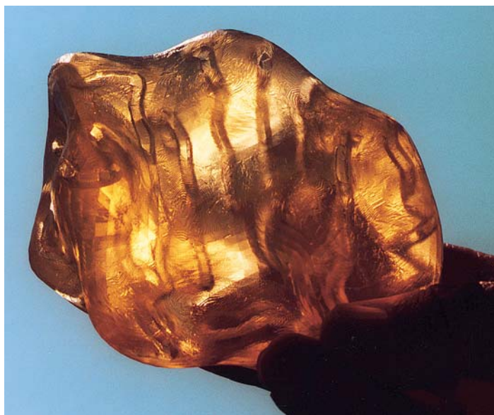
Fig. 17.2.4.2. A stereolithographic model of betalactamase inhibitory protein (BLIP). The model depicts the shape of the molecule as represented by a spherical-harmonic approximation of the solvent-excluded surface. Inside the surface is a hollow tube which follows the \alpha -carbon trace of the protein backbone. The model was designed by Michael Pique and Arthur Olson, and fabricated on a 3D systems SLA 1000 by Beryl Hodgson.
