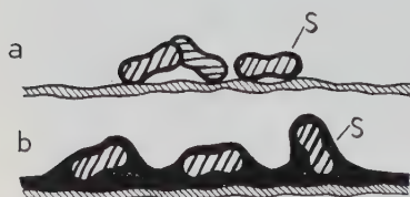
Fig. 4.109a,b. Positive (a) and negative (b) staining of biomolecules on a substrate ( S : stain)
