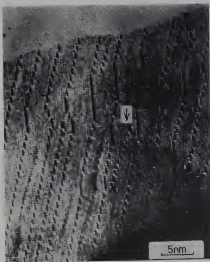
Fig. 1.93. Electron micrograph of a crystal of overall composition \text{Ti}_{0.03}\text{WO}_3 containing mostly [103] CS planes. Short segment of [102] GS plane is arrowed [1.65]
