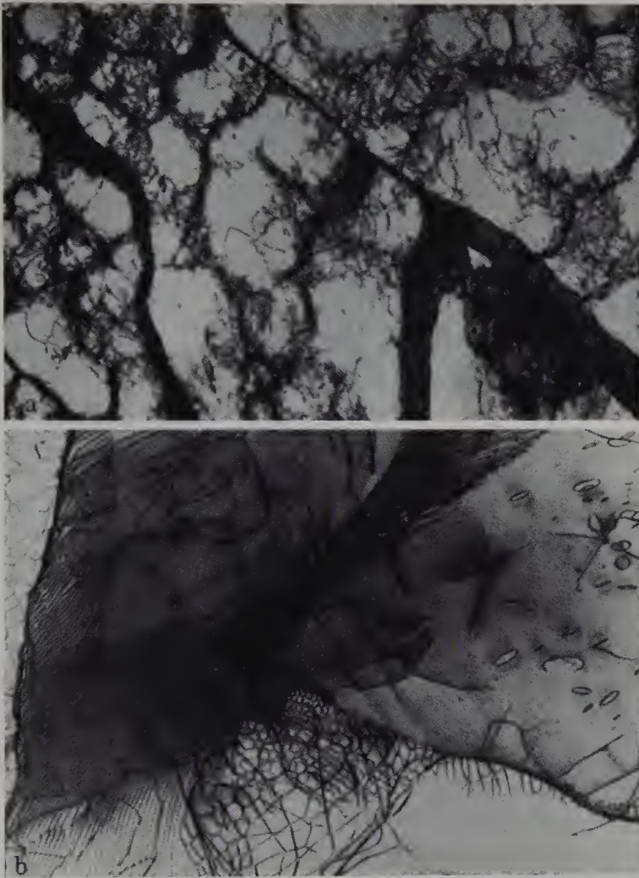
Fig. 5.40a, b. Mosaic structure. (a) X-ray topogram of an MgO crystal, \times 15 (Courtesy of V. F. Miuskov); (b) electron micrograph of a Ge crystal, \times 20,000 (Courtesy of N. D. Zakharov)
