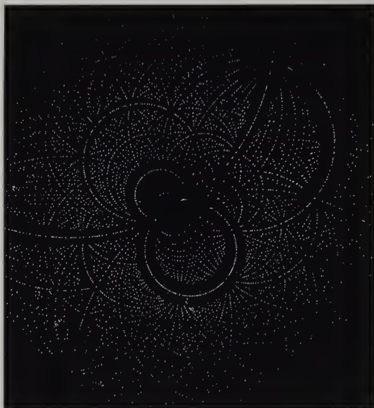
Fig. 6.42. Laue photograph of endonuclease serrata marcescens crystals, wavelengths interval 0.5–2.5 Å. DESY-Doris synchrotron. (Courtesy of H. D. Bartunik)
