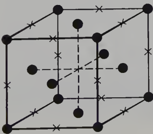
Fig. 1.88. Austenite structure. Crosses represent the positions of the C atoms being incorporated into the \gamma -Fe lattice
