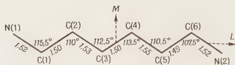
Fig. 65. Configuration of the hexamethylenediamine molecule.
