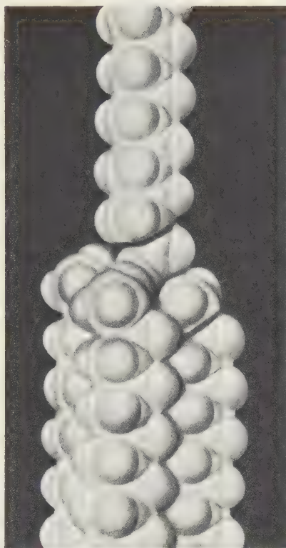
Fig. 52. Packing of molecules in triclinic n -paraffins.
