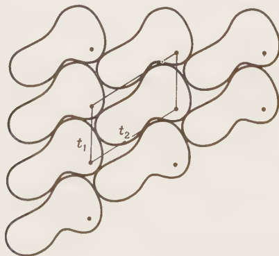
Fig. 19. Dense layer with symmetry p1 .
