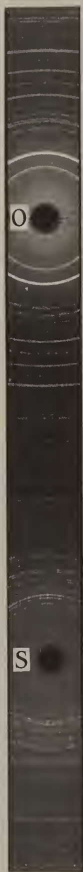
Fig. 10.7. An example of a Debye-Scherrer X-ray film ( \text{CuK}\alpha X-radiation) for \text{SiO}_2 (quartz). S is the 'entrance' hole and O the 'exit' hole. The 'spotty' appearance of the rings arises because of the relatively coarse crystallite size in the specimen. At high 2\theta angles (near the entrance hole) the \text{K}\alpha_1/\text{K}\alpha_2 doublets are resolved but at low 2\theta angles (near the exit hole) they are unresolved. The streaks around the exit hole arise from the presence of residual 'white' X-radiation in the incident beam.
