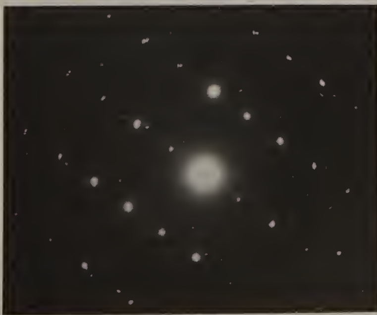
Fig. 9.23. An electron diffraction pattern (ZOLZ) of a particle extracted from a nitrided chromium-containing steel. The camera constant \lambda L (adjusted for print size) is 38 Å mm (see Exercise 9.5).
