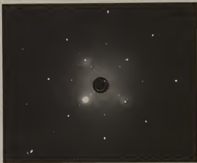
Fig. 9.10. (a) The geometry of the back reflection Laue method for a particular set of hkl planes in a single crystal. The wavelength of the reflected beam is that for which Bragg's law is satisfied for the particular fixed \theta and d_{hkl} value. (b) A back reflection Laue photograph of a single crystal of aluminium oriented with a \langle 100 \rangle direction nearly parallel to the incident X-ray beam showing the reflections S from many (hkl) planes. They lie on a series of intersecting hyperbolae (close to straight lines in this photograph), each hyperbola corresponding to reflections from planes in a single zone, [uvw] . Note the four-fold symmetry of the intersecting zones indicating the \langle 100 \rangle crystal orientation. (Photograph by courtesy of Prof. G. W. Lorimer.)
