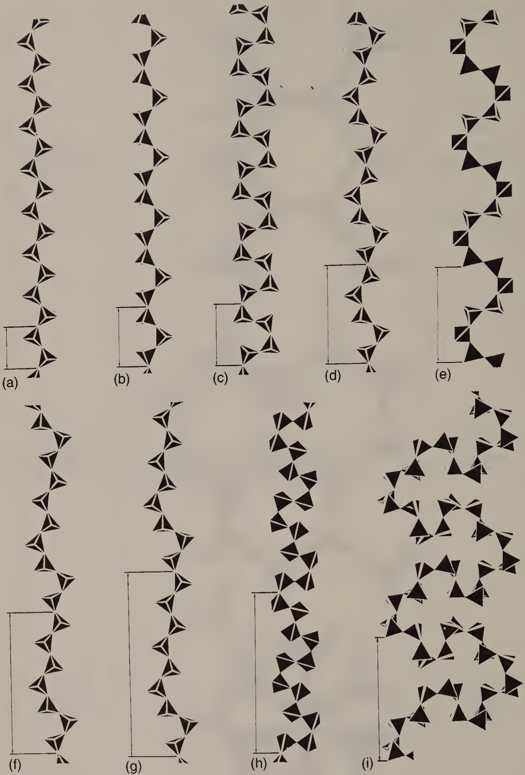
Fig. 1.24. The arrangements of the tetrahedra in the inosilicates. They are described (in German) according to the number of the tetrahedra in the repeat distance: a (zweier); b (dreier); c (vierer); d (fünfer); e (sechser); f (siebener); g (neuner); h (zwölfer); i (24er) (from Structural Chemistry of Silicates by F. Liebau, Springer-Verlag, 1985).
