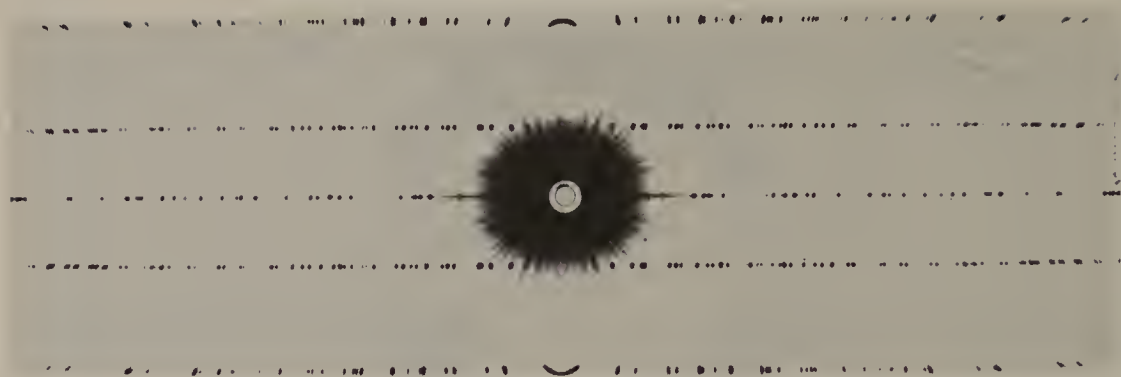
Fig. 9.13. A rotation crystal photograph of topaz \text{Al}_2(\text{SiO}_4)(\text{OH}, \text{F})_2 , orthorhombic. The cylindrical film is shown laid flat with the X-ray beam exit hole at the centre and the rotation axis (in this case the x -axis) vertical. Notice the large number of reflections in each layer line and the vertical and horizontal mirror lines of symmetry which arise because the reflecting sphere sweeps through a much larger region of reciprocal space during the 360^\circ rotation of the crystal than for an oscillation photograph. (Photograph by courtesy of Dr. M. S. Hampar.)
