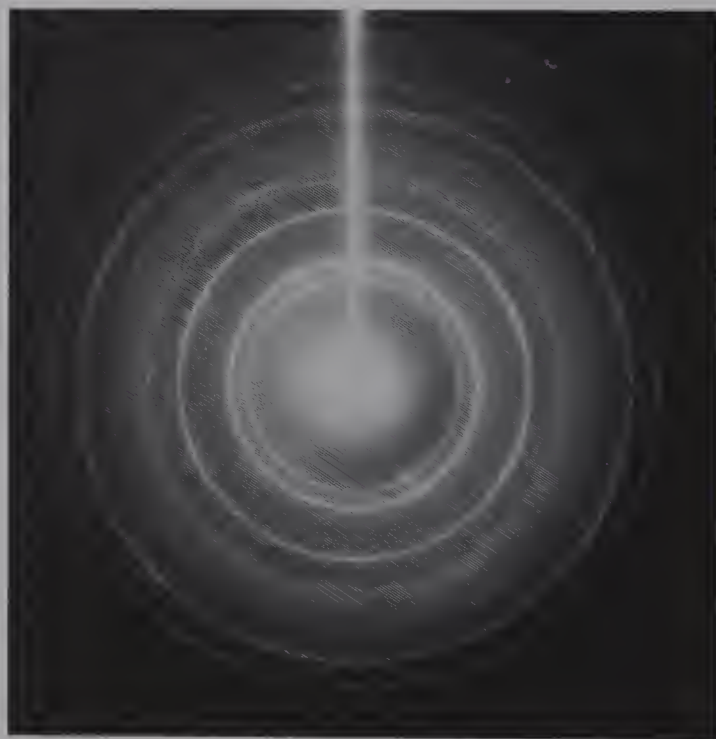
Fig. 11.6. An electron diffraction pattern of polycrystalline aluminium, showing varying intensities of the diffraction rings and the sequence of ring spacings characteristic of the fcc structure.
