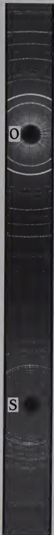
Fig. 10.7. An example of a Debye-Scherrer X-ray film ( \text{CuK}\alpha X-radiation) for \text{SiO}_2 (quartz). S is the 'entrance' hole and O the 'exit' hole. The 'spotty' appearance of the rings arises because of the relatively coarse crystallite size in the specimen. At high 2\theta angles (near the entrance hole) the \text{K}\alpha_1/\text{K}\alpha_2 doublets are resolved but at low 2\theta angles (near the exit hole) they are unresolved. The streaks around the exit hole arise from the presence of residual 'white' X-radiation in the incident beam.
