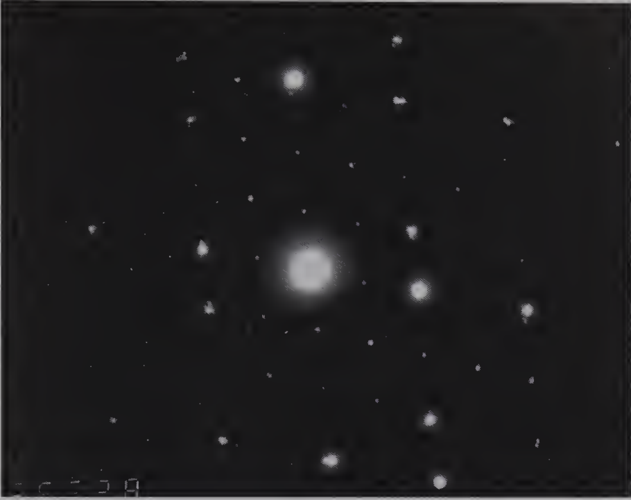
Fig. 11.10. A selected area electron diffraction pattern of a thin foil of a quenched and tempered steel showing reflections from \text{Fe}_3\text{C} precipitates in a single crystallographic orientation (weak spots) and two twin-related orientations of the ferrite ( \alpha\text{-Fe} ) matrix (strong spots). (Photograph by courtesy of Dr. D. H. Jack)
