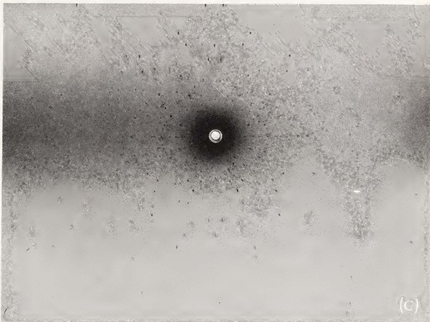
Figure 5.6 Laue photographs (a) Back-reflection photograph taken with a polaroid camera and fluorescent screen. (b) Forward-reflection photograph on a flat plate showing a hexagonal axis parallel to the X-ray beam. (c) Photograph taken using a film in a cylindrical cassette shows mirror planes parallel and perpendicular to the X-ray beam.
