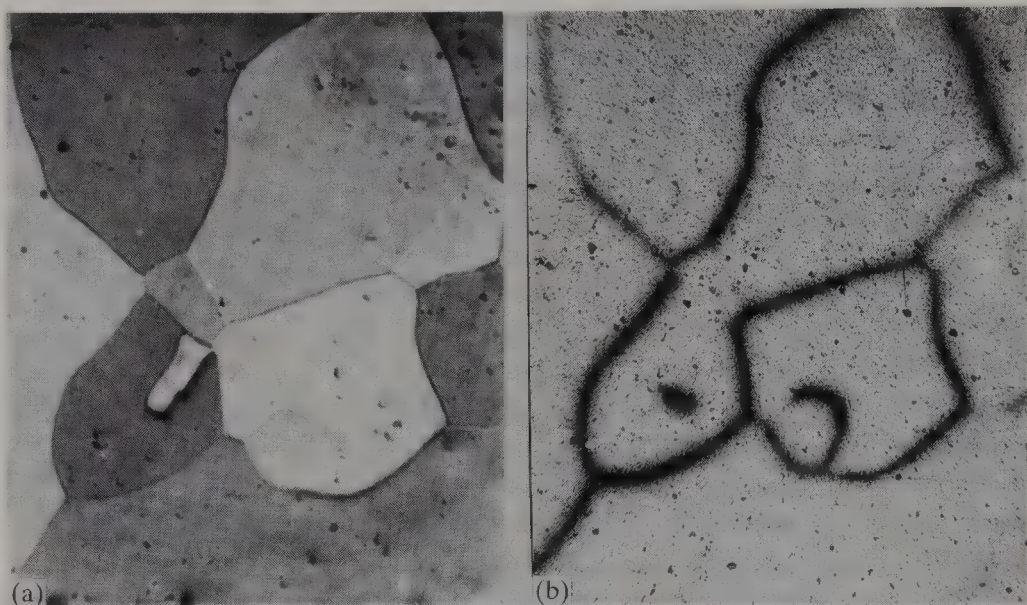
Fig. 5.9. Intergranular diffusion of radioactive Fe in iron: (a) metallographic image; (b) autoradiography. There is no diffusion along the twin boundaries since no disorder occurs there (by kind permission of P. Lacombe).
