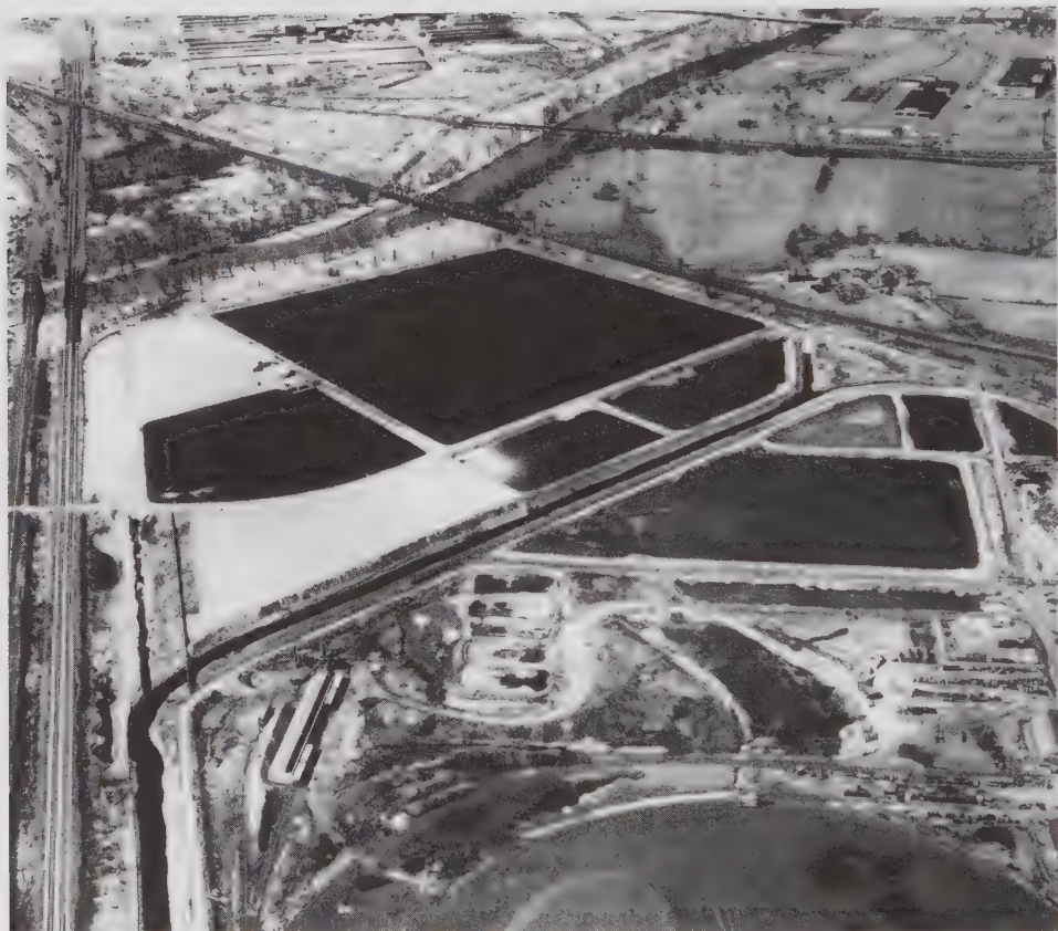
Aerial view of Bound Brook waste-treatment area showing basins, or lagoons, and Cuckold's Brook, looking toward the southwest, around 1950. Equalization basin no. 6 is to the left. To its right is the settling basin, no. 7. The Dorrco neutralization unit is between basins 6 and 7. In the distance, beyond the Raritan River, is the Johns-Manville facility. (Fairchild Aerial Surveys/Edelstein Library.)
