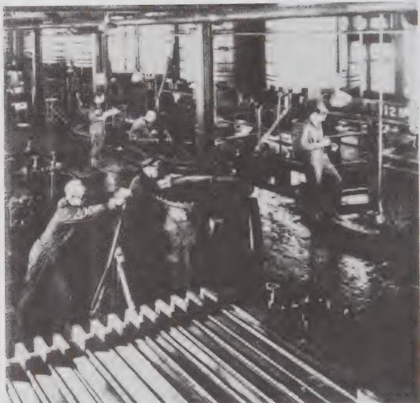
Interior of azo dye manufacturing building at Bound Brook, 1940. Note the raised wooden diazotization tubs, filter press in the foreground, and the protective clothing worn by workers. ( Dyes Made in America, 1915–1940 [Bound Brook: American Cyanamid Company, 1940]/Edelstein Collection.)
