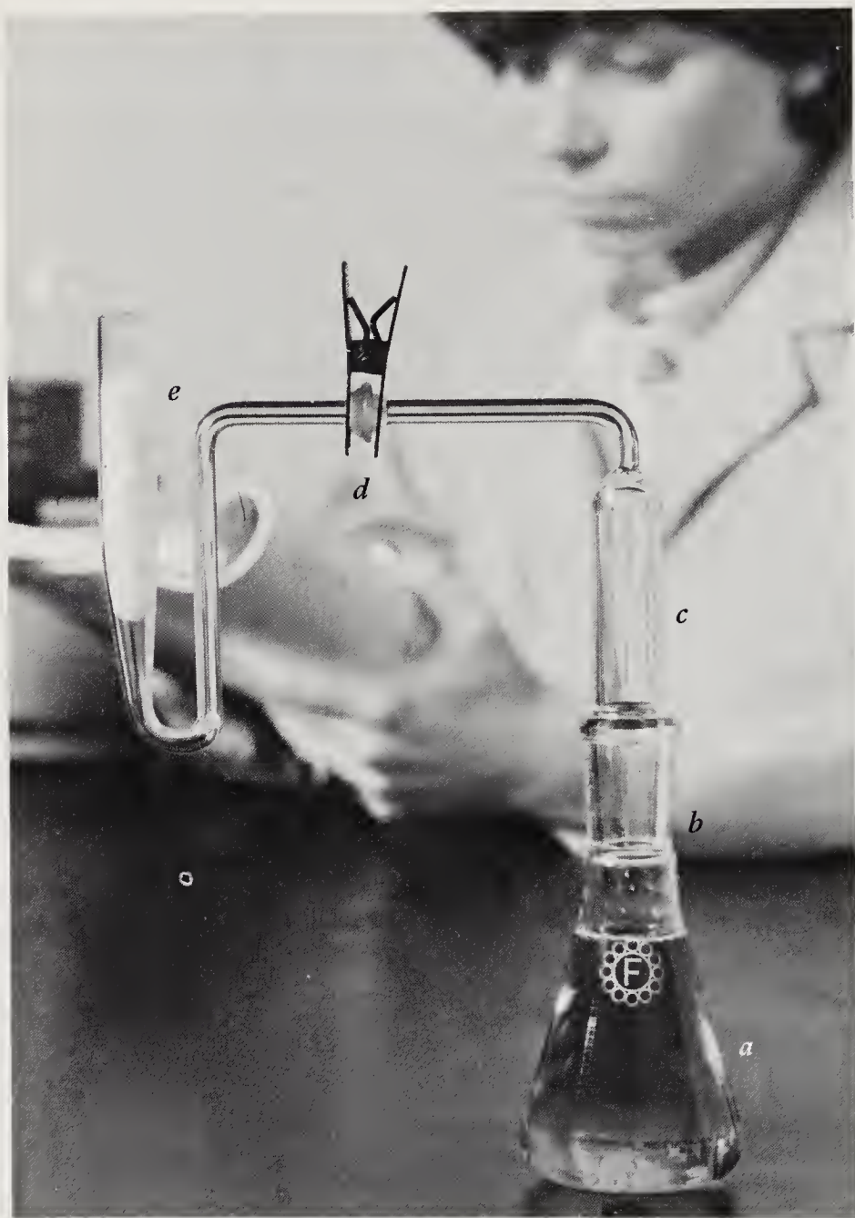
Figure 6 Apparatus for Arsenic Test (Courtesy Fisher Scientific Co.)
