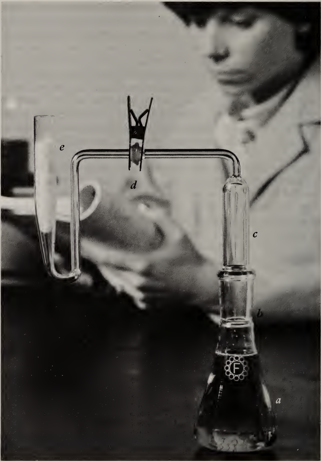
Figure 10.1 Apparatus for arsenic test. (courtesy Fisher Scientific Co)
