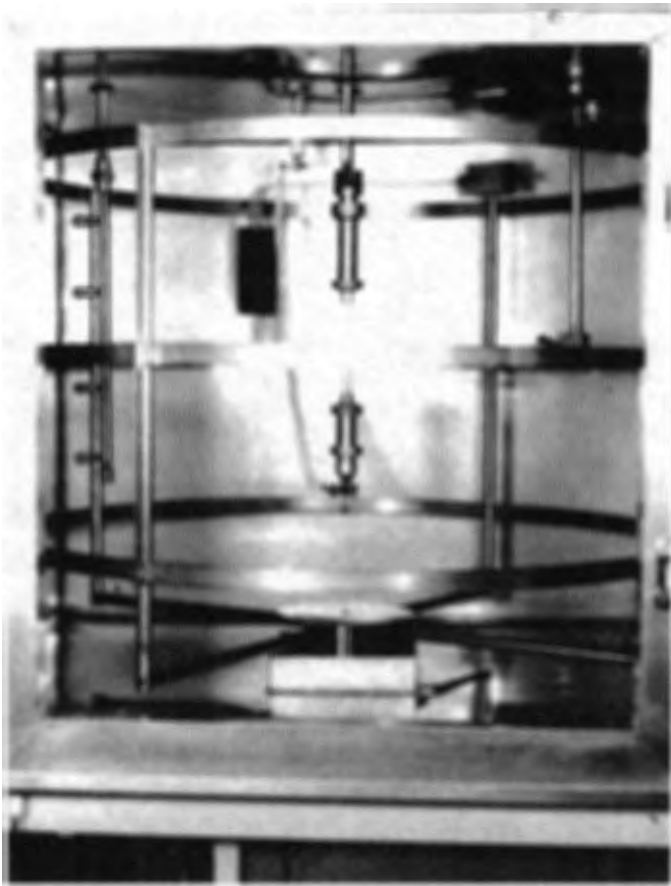
Plate 19.7 — The 6500 watt xenon arc system employed in the Ci65.
