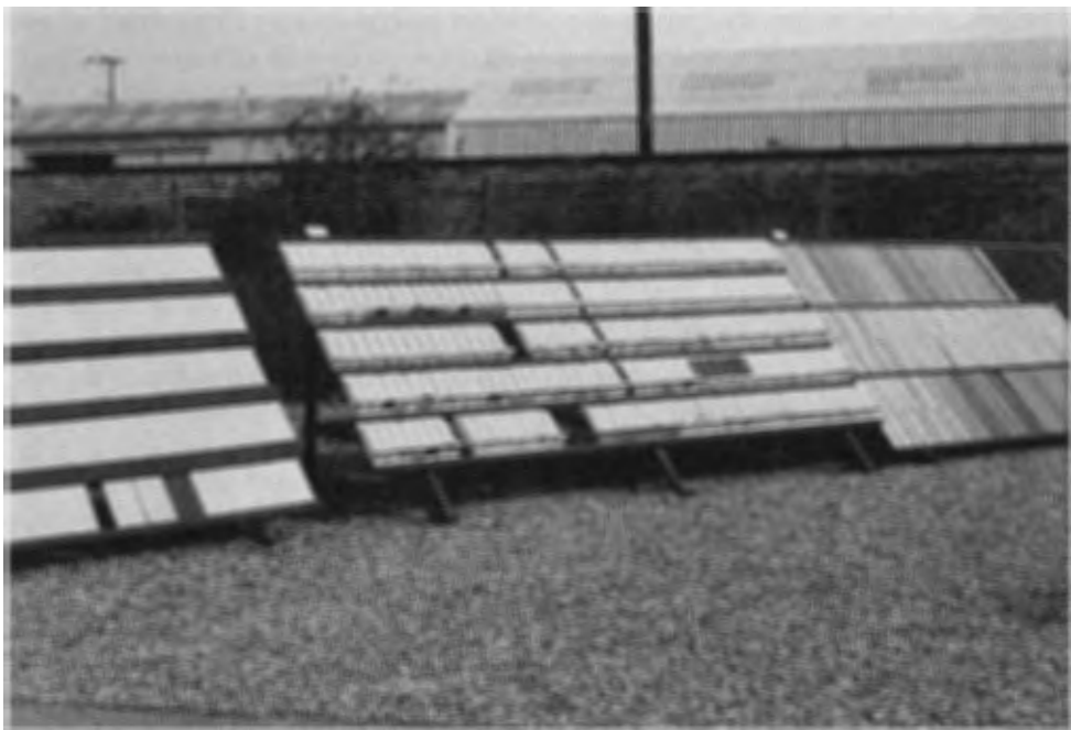
Plate 19.9 — Panel racks for exterior exposure of panels.
