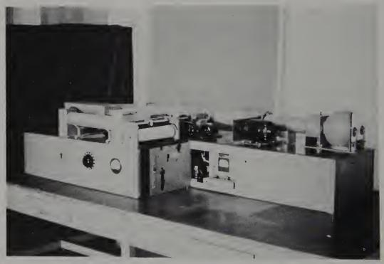
Figure 9.2 The first recording spectrophotometer.
