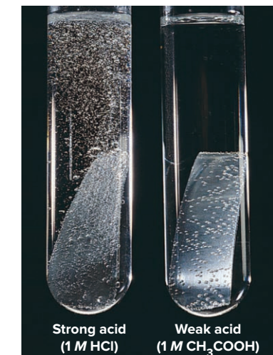
Figure 18.2 Reaction of zinc with a strong acid ( left ) and a weak acid ( right ).
