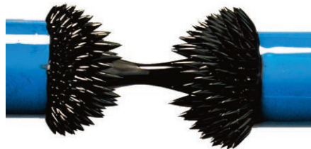
Figure 12.50 The magnetic behavior of a ferrofluid. Nanoparticles of magnetite ( \text{Fe}_3\text{O}_4 ) dispersed in a viscous fluid are suspended between the poles of a magnet.
