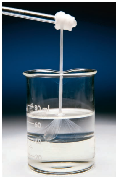
Figure 15.28 The formation of nylon-66 . In the laboratory, the six-C diacid chloride, which is more reactive than the diacid, is used as one monomer; the polyamide forms between the two liquid phases.
