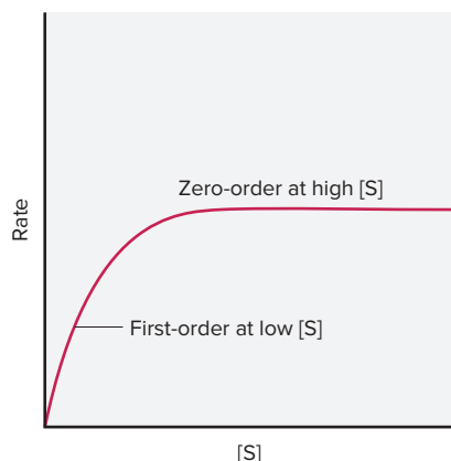
Figure 16.27 Plot of the initial rate of an enzyme-catalyzed reaction versus substrate concentration
