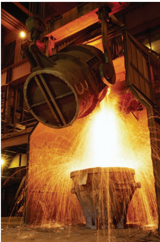
Figure 22.18 The basic-oxygen process for making steel.
