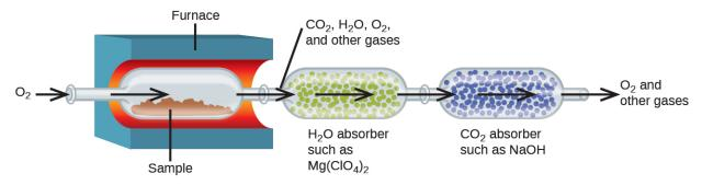
**Figure 4.17** This schematic diagram illustrates the basic components of a combustion analysis device for determining the carbon and hydrogen content of a sample.
