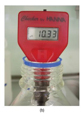
Figure 14.4 (a) A research-grade pH meter used in a laboratory can have a resolution of 0.001 pH units, an accuracy of  $\pm$  0.002 pH units, and may cost in excess of \$1000. (b) A portable pH meter has lower resolution (0.01 pH units), lower accuracy ( $\pm$  0.2 pH units), and a far lower price tag. (credit b: modification of work by Jacopo Werther)
