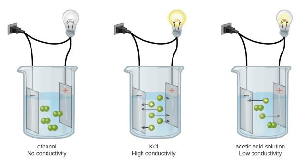
**Figure 11.7** Solutions of nonelectrolytes such as ethanol do not contain dissolved ions and cannot conduct electricity. Solutions of electrolytes contain ions that permit the passage of electricity. The conductivity of an electrolyte solution is related to the strength of the electrolyte.
