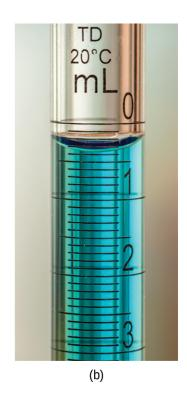
**Figure 4.15** (a) A student fills a buret in preparation for a titration analysis. (b) A typical buret permits volume measurements to the nearest 0.01 mL. (credit a: modification of work by Mark Blaser and Matt Evans; credit b: modification of work by Mark Blaser and Matt Evans)
