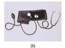
**Figure 9.6** (a) A medical technician prepares to measure a patient's blood pressure with a sphygmomanometer. (b) A typical sphygmomanometer uses a valved rubber bulb to inflate the cuff and a diaphragm gauge to measure pressure. (credit a: modification of work by Master Sqt. Jeffrey Allen)
