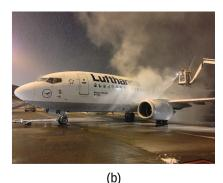
Figure 11.23 Freezing point depression is exploited to remove ice from (a) roadways and (b) the control surfaces of aircraft.
