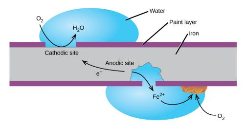
**Figure 17.17** Once the paint is scratched on a painted iron surface, corrosion occurs and rust begins to form. The speed of the spontaneous reaction is increased in the presence of electrolytes, such as the sodium chloride used on roads to melt ice and snow or in salt water.
