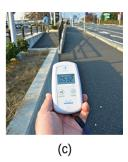
Figure 21.35 Devices such as (a) Geiger counters, (b) scintillators, and (c) dosimeters can be used to measure radiation. (credit c: modification of work by "osaMu"/Wikimedia commons)
