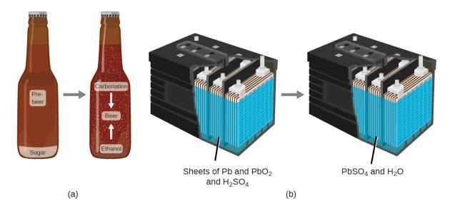
Figure 1.8 (a) The mass of beer precursor materials is the same as the mass of beer produced: Sugar has become alcohol and carbonation. (b) The mass of the lead, lead oxide plates, and sulfuric acid that goes into the production of electricity is exactly equal to the mass of lead sulfate and water that is formed.
