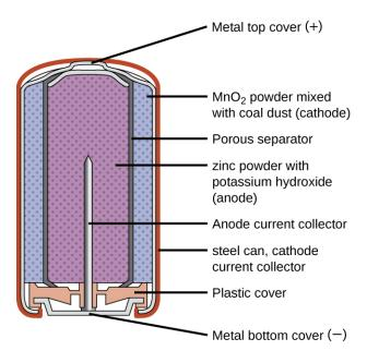
Figure 17.11 Alkaline batteries were designed as direct replacements for zinc-carbon (dry cell) batteries.
