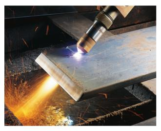
Figure 1.7 A plasma torch can be used to cut metal. (credit: "Hypertherm"/Wikimedia Commons)
