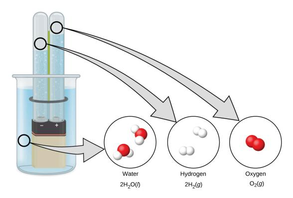
**Figure 18.26** The electrolysis of water produces hydrogen and oxygen. Because there are twice as many hydrogen atoms as oxygen atoms and both elements are diatomic, there is twice the volume of hydrogen produced at the cathode as there is oxygen produced at the anode.
