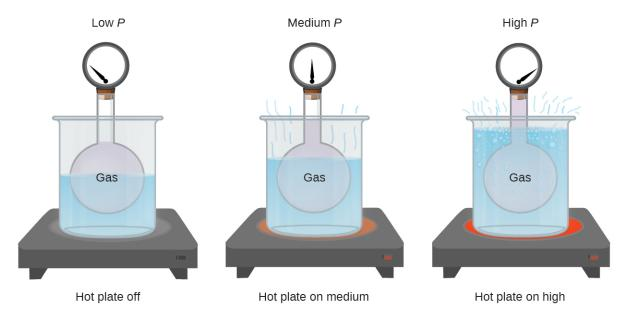
**Figure 9.10** The effect of temperature on gas pressure: When the hot plate is off, the pressure of the gas in the sphere is relatively low. As the gas is heated, the pressure of the gas in the sphere increases.
