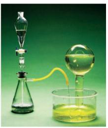
**Figure 12-7** Apparatus for preparing hydrogen from zinc and sulfuric acid.
