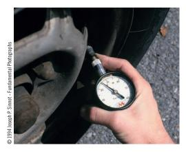
© A tire gauge. This kind of gauge registers "relative" pressure, that is, the *difference* between internal pressure and the external atmospheric pressure. For instance, when the gauge reads 30 psi (pounds per square inch), the total gas pressure in the tire is 30 psi + 1 atm, or about 45 psi. In engineering terminology, this is termed "psig" (g = gauge). For all calculations involving pressure, the total pressure, not gauge pressure, must be used.
