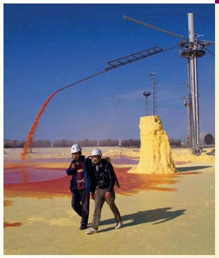
The tower in the background is part of the Frasch process that pumps molten sulfur (dark orange) from underground deposits. After it cools, it forms bright yellow solid sulfur. The workers are wearing respirators to protect them from the small amounts of  $SO_2$  that form when the hot molten sulfur reacts with oxygen in the air.
