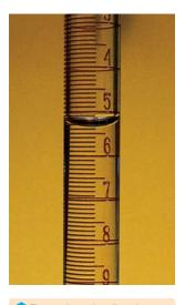
3 The meniscus describes the surface of the liquid in the buret. Aqueous solutions wet glass, so the meniscus of an aqueous solution is always concave. The position of the bottom of the meniscus is read and recorded.
