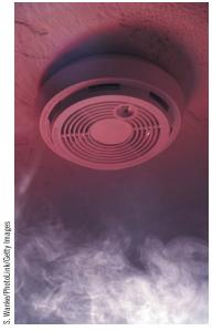
A weakly radioactive source such as americium is used in some smoke detectors. Radiation from the source ionizes the air to produce a weak current. Smoke particles interrupt the current flow by attracting the ions. This decrease in current triggers the alarm.
