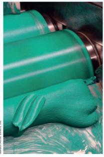
A milling machine mixes pigments with light oils to produce oil paint. Pigments in paints usually do not dissolve, but rather are very finely dispersed into oil or another liquid.
