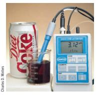
The pH of a Diet Coke is measured with a modern pH meter. Many carbonated soft drinks are acidic due to the dissolved  ${\rm CO_2}$  and phosphoric acid (both weak acids).
