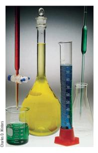
Figure 1-18 Some laboratory apparatus used to measure volumes of liquids: 150-mL beaker (bottom left, green liquid); 25-mL buret (top left, red); 1000-mL volumetric flask (center, yellow); 100-mL graduated cylinder (right front, blue); and 10-mL volumetric pipet (right rear, green).
