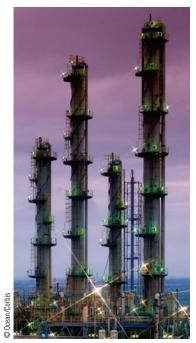
Crude oil is separated by fractional distillation into many components such as gasoline, kerosene, fuel oil, paraffin, and asphalt. The distillation towers in chemical plants are typically four to ten stories tall and can process many tons of liquid mixtures each day.
