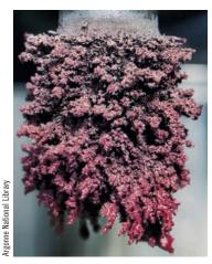
Uranium is deposited on the negative electrode in the electrorefining phase of fuel reprocessing. The crystalline mass is about 97% LiCl and KCl. The remaining 3% uranium chloride is responsible for the amethyst color.
