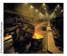
3 Casting molten aluminum. Electrolytic cells used in the Hall—Héroult process appear in the background.
