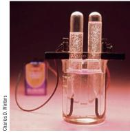
Electrolysis of water to produce  $O_2(g)$  and  $H_2(g)$ .  $Na_2SO_4$  was dissolved in the water to improve the conductivity. Can you identify which tube in this picture is collecting the  $H_2$  gas and the name of the electrode producing it (anode or cathode)?
