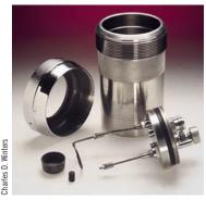
A disassembled bomb calorimeter
