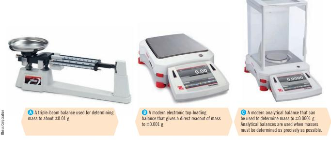
Figure 1-16 Three types of laboratory balances.
