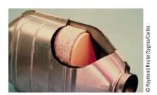
B A cutaway view of a catalytic converter, showing the pellets of catalyst
