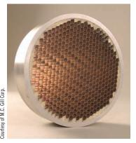
This aluminum honeycomb material is made by bonding aluminum foil sheets to form hexagonal cells. It is used to make sandwich construction panels that have a very high strength-to-weight ratio.
