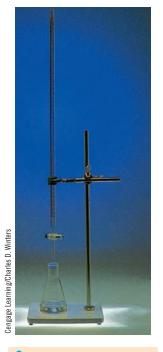
A typical setup for titration in a teaching laboratory. The solution to be titrated is placed in an Erlenmeyer flask, and a few drops of indicator are added. The buret is filled with a standard solution (or the solution to be standardized). The volume of solution in the buret is read carefully.
