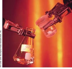
Robotics technology is used to manipulate highly radioactive samples safely.
