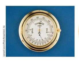
3 Portable barometers. This type is called an aneroid ("not wet") barometer. Some of the air has been removed from the airtight box, which is made of thin, flexible metal. When the pressure of the atmosphere changes, the remaining air in the box expands or contracts (Boyle's Law), moving the flexible box surface and an attached pointer along a scale.
