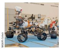
The Curiosity Mars rover is powered by a  $^{238}$ Pu $^{0}$ Pu $^{0}$ thermoelectric battery. The rover requires more power than solar cells could provide.
