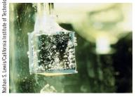
Gaseous H<sub>2</sub> is produced from H<sub>2</sub>O at an illuminated photoelectrode. Light from the sun may soon be used to produce hydrogen, the ultimate clean-burning fuel.
