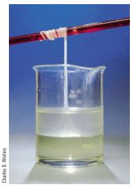
Nylon is formed at the interface where hexamethylenediamine (in the lower water layer) and adipoyl chloride (a derivative of adipic acid, in the upper hexane layer) react. The nylon can be drawn out and wound on a stirring rod. In industry, adipic acid is used in place of adipyl chloride.
