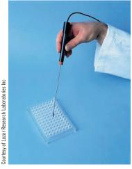
Microelectrodes have been developed to measure concentrations in very small volumes of solution.
