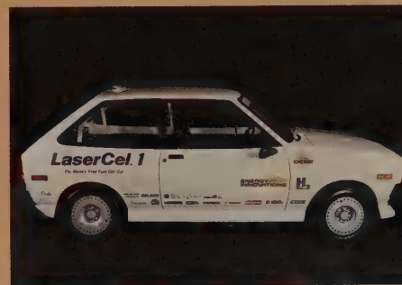
The LaserCel 1, unveiled in 1991, is more economical to operate on hydrogen than on gasoline. This is accomplished by replacing the internal combustion engine with a hydrogen fuel cell.
