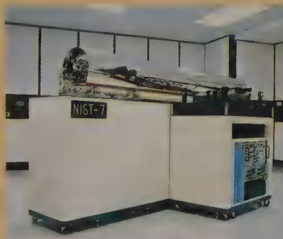
The atomic clock at the National Institute of Standards and Technology in Boulder, CO, loses only 1 second in a million years.
