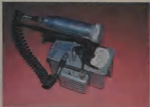
FIGURE 18.5 Left: Geiger-Müller survey meter. Right: Worker wearing film badge (above I.D. tag) to measure radioactivity.
