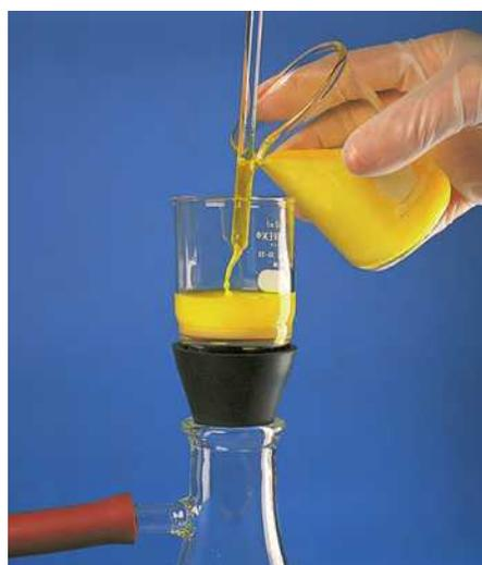
**b** The solution is filtered by pouring it into a crucible containing a porous glass partition. Afterward, the crucible is heated to dry the barium chromate. By weighing the crucible before and afterward, you can determine the mass of precipitate.
