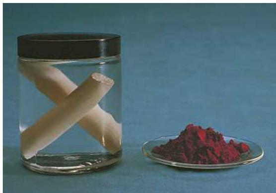
White phosphorus is a major industrial chemical and is prepared by heating phosphate rock with coke (C) and quartz sand (SiO<sub>2</sub>) in an electric furnace. The overall reaction is
