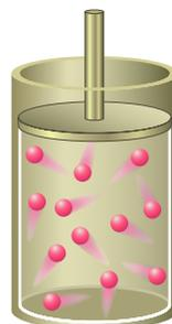
**c** Container after the molecules are allowed to move the piston and increase the volume. The concentration of gas molecules and frequency of collisions with the container walls have decreased, and the pressure of the gas molecules inside the container is again equal to atmospheric pressure ( $P_{\text{inside}} = P_{\text{atm}}$ ).
