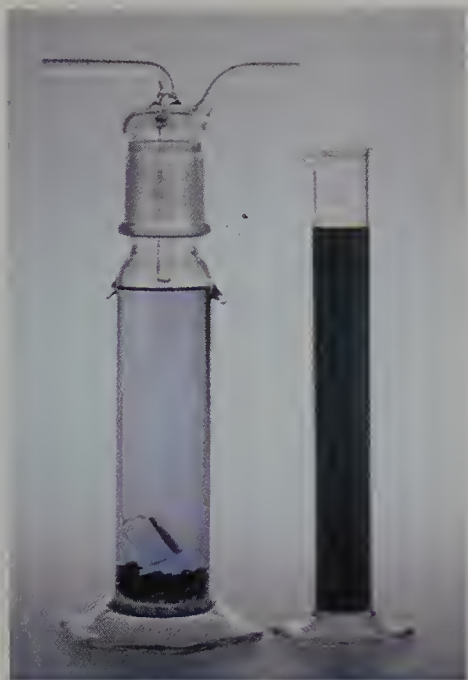
Figure 20-11 A chromous bubbler, which is used to remove traces of oxygen from inert gases such as nitrogen or argon. The apparatus on the left is the chromous bubbler. The blue color of the solution is due to \text{Cr}^{2+}(\text{aq}) . The solid at the bottom of the tube is zinc amalgam ( \text{Zn} + \text{Hg} ). The green solution in the graduated cylinder is \text{Cr}_2(\text{SO}_4)_3(\text{aq}) , which is used to prepare the chromous bubbler. The green \text{Cr}(\text{III}) is reduced to the blue \text{Cr}(\text{II}) by the zinc amalgam. The gas to be deoxygenated enters the bubbler at the left inlet tube, bubbles up through the solution of \text{Cr}(\text{II}) , and exits from the right tube. A glass frit at the bottom of the inlet tube breaks up the entering gas stream into small bubbles.
