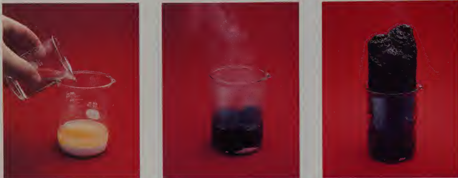
Figure L-10 Concentrated (98%) sulfuric acid is a powerful dehydrating agent capable of converting sucrose to carbon.
