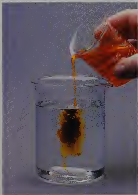
Figure 18-1 Addition of a 0.10M solution of the oxidizing agent potassium dichromate, \text{K}_2\text{Cr}_2\text{O}_7 (aq) (orange solution), to a solution 0.10M in iron(II) sulfate, \text{FeSO}_4 (aq) (light green), and 0.10M in \text{H}_2\text{SO}_4 (aq) . The iron is oxidized from Fe(II) to Fe(III) and the chromium is reduced from Cr(VI) to Cr(III).
