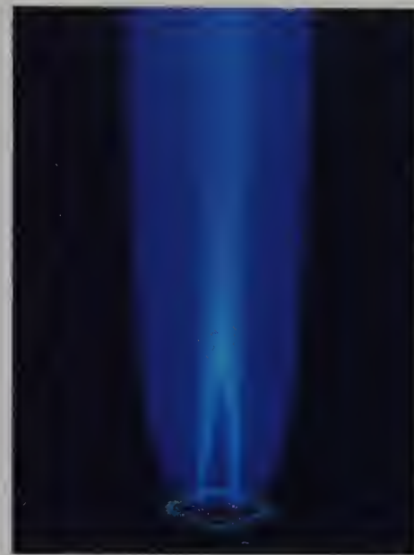
Figure D-1 An oxy-hydrogen torch. The flame temperature is about 2500^\circ\text{C} .
