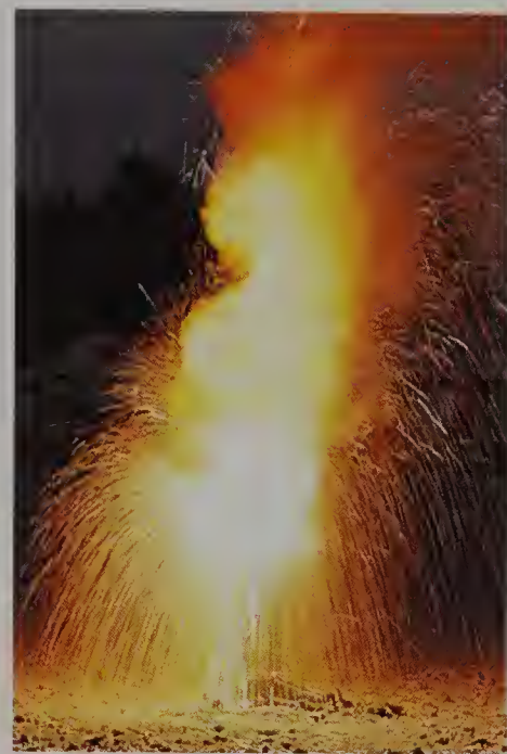
Figure 3-4 A thermite reaction. A spectacular example of a single-replacement reaction is the reaction between powdered aluminum metal and iron(III) oxide
