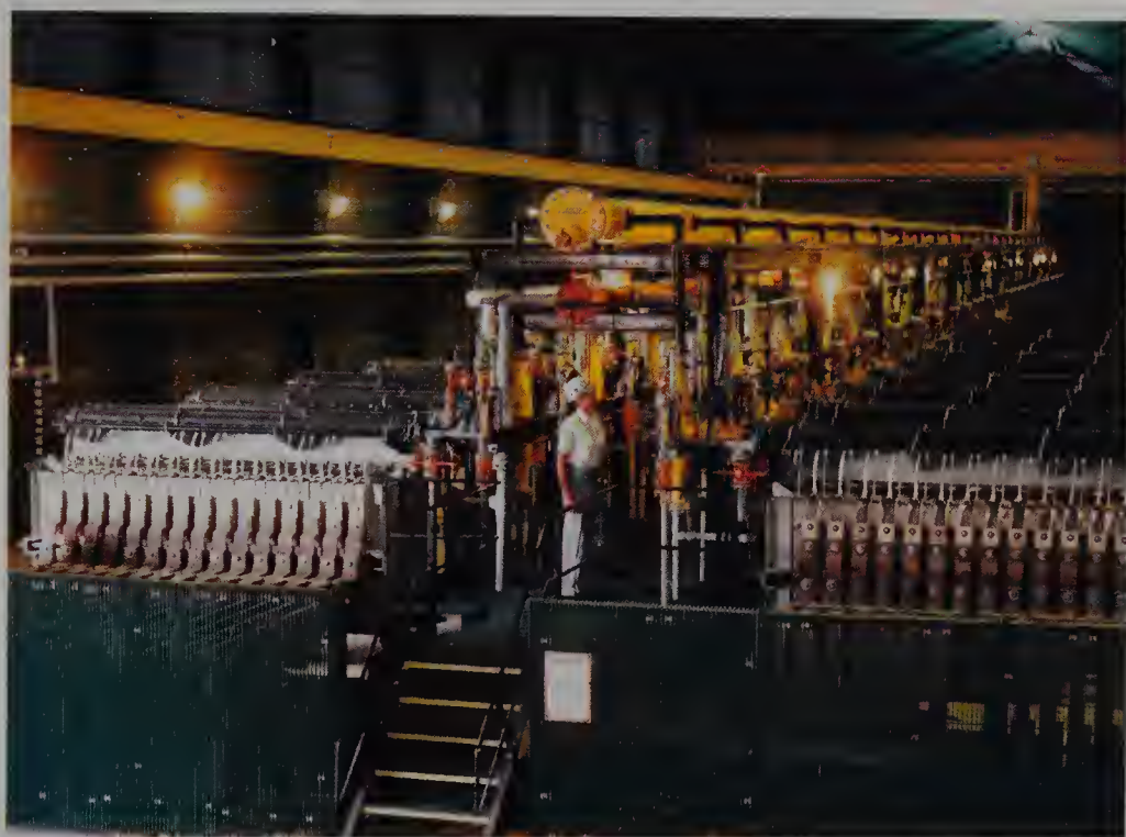
A chlor-alkali plant, in which chlorine and sodium hydroxide are obtained from sodium chloride by electrolysis.
