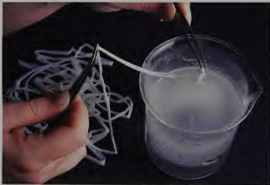
Figure 24-1 The formation of nylon by a condensation polymerization reaction at the interface of two immiscible solvents, one of which (water) contains the diamine monomer \text{H}_2\text{N}(\text{CH}_2)_6\text{NH}_2 plus \text{NaOH}(\text{aq}) and the other of which (hexane) contains the compound \text{ClC}(\text{CH}_2)_4\text{CCl} . The small molecule
