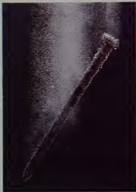
Figure 2-21 The reaction between iron metal and a dilute aqueous solution of sulfuric acid. The bubbles generated at the surface of the iron nail are hydrogen gas. The iron replaces the hydrogen in \text{H}_2\text{SO}_4 and thereby enters the solution as \text{FeSO}_4(aq) .
