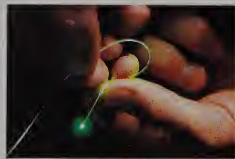
Figure H-9 Fiber optics. Light is transmitted through thin strands of silica glass that form an optical-waveguide fiber bundle.
