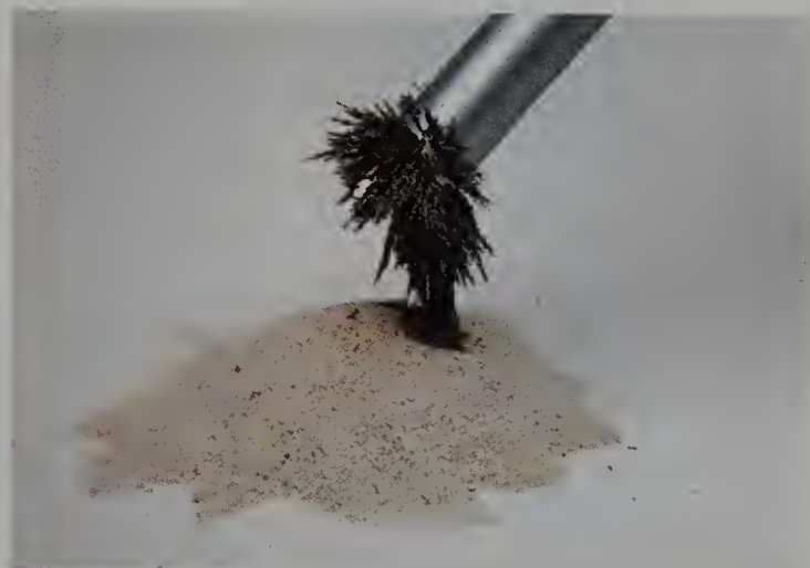
(d) A magnet can be used to separate iron filings from the mixture. The iron filings are attracted by the magnet, but the other three components are not.
