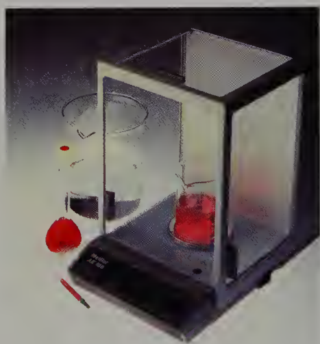
Figure 1-11 A modern analytical balance, used to determine mass. The mass determination is made by turning a dial to find the known mass (using a set of standard masses enclosed within the balance) that balances the unknown mass. When the two masses just balance, they are equal within the accuracy of the balance.
