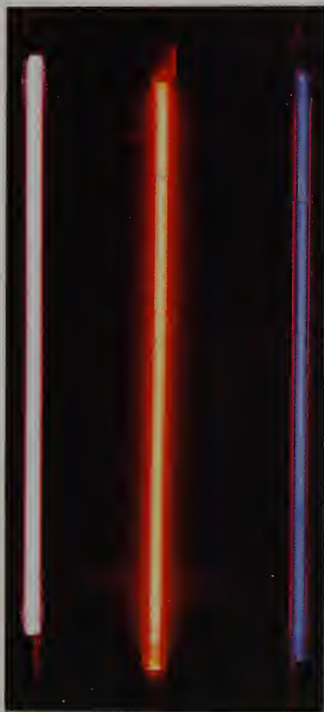
Figure 2-6 When an electric discharge is passed through a noble gas, light of a characteristic color is emitted. The tubes in the photo contain helium ( left ), neon ( center ), and argon ( right ).
