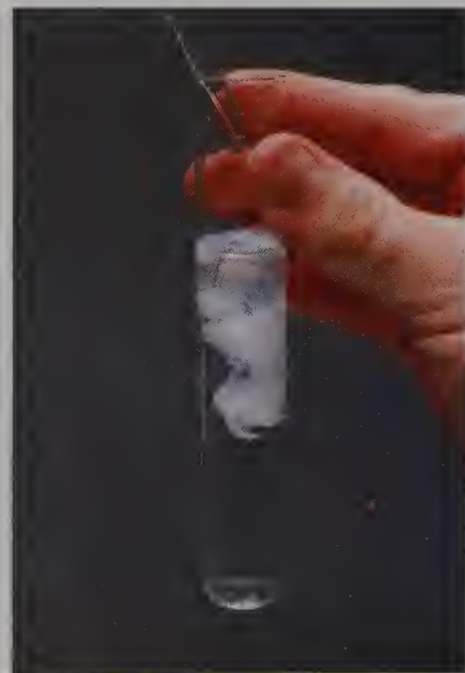
Figure 2-24 The reaction of \text{NaCl}(aq) with \text{AgNO}_3(aq) yields the white precipitate \text{AgCl}(s) .
