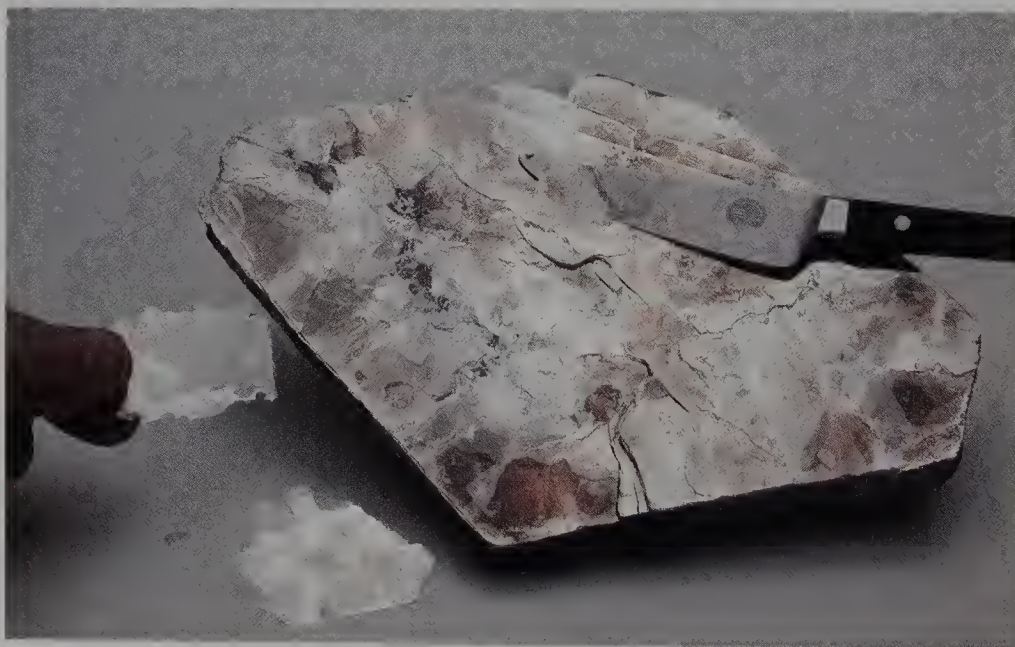
Figure H-7 The ease with which the mineral mica can be separated into thin sheets is a direct consequence of the existence of polymeric silicate sheets with the composition (\text{Si}_2\text{O}_5^{2-})_n .
