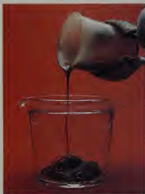
Figure L-8 If liquid sulfur at about 200°C is cooled quickly by pouring it into cold water, a rubbery substance called plastic sulfur is obtained.
