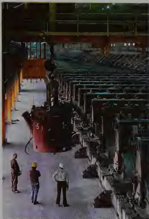
Figure 20-5 The Hall process on an industrial scale. Shown here is an Alcoa potline (198 pots) at the Massena, New York, plant.
