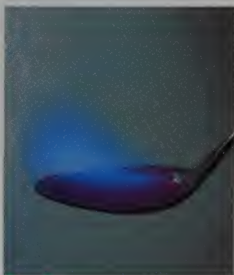
Figure 2-16 Sulfur burns in oxygen with a blue flame. The production of \text{SO}_2 by burning sulfur is a key reaction in the manufacture of sulfuric acid. Sulfur dioxide is also produced when sulfur-containing coal or petroleum is burned.
