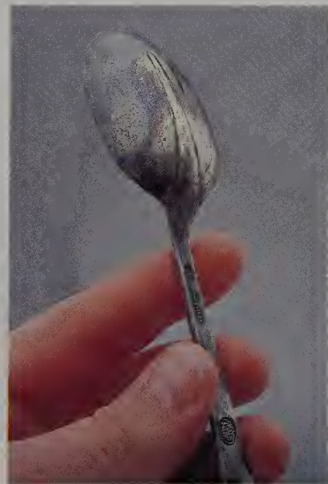
Figure L-11 Silver sulfide is a black, insoluble solid that appears as a dark tarnish on the surface of silver.
