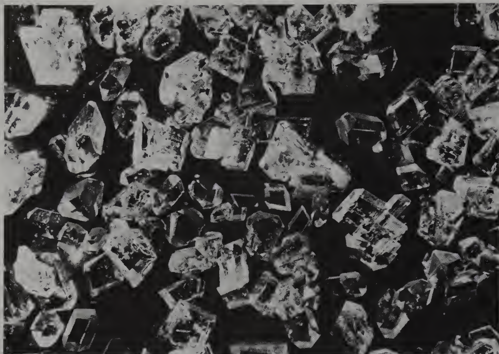
Figure M-2 Xenon tetrafluoride crystals. Xenon tetrafluoride was first prepared in 1962 by the direct combination of \text{Xe}(g) and \text{F}_2(g) in a nickel reaction chamber at 6 atm and 400^\circ\text{C} .
