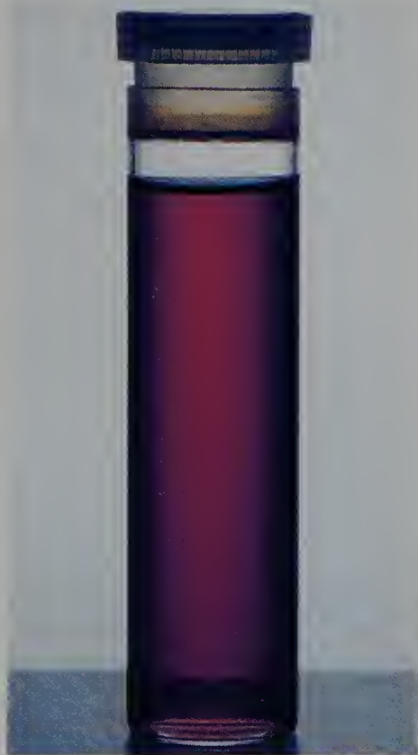
Figure 22-12 An aqueous solution of titanium(III) chloride. The d^1 ion [\text{Ti}(\text{H}_2\text{O})_6]^{3+} has a red-purple color.
