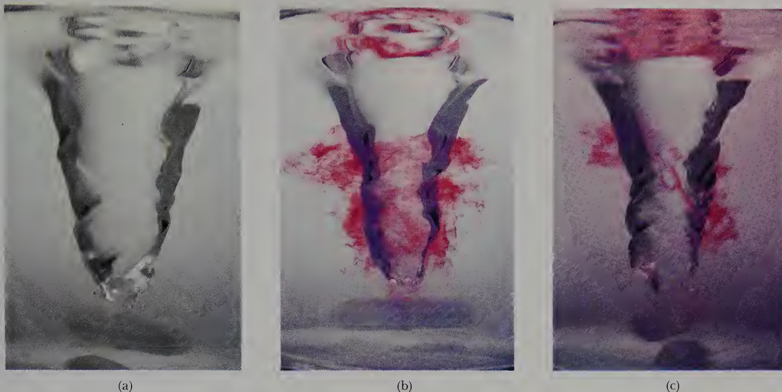
Figure 16-4 Experimental setup for the titration of \text{HCl}(aq) with \text{NaOH}(aq) . A 50.0-mL sample of \text{HCl}(aq) is placed in the reaction flask together with a magnetic bar for stirring the reaction mixture during the titration. (a) Two or three drops of the acid-base indicator phenolphthalein is added to the \text{HCl}(aq) , and then (b) \text{NaOH}(aq) is added from a buret. As the equivalence point is approached, the base is added dropwise until (c) a single drop turns the entire reaction mixture a pink color that does not revert to colorless with stirring.
