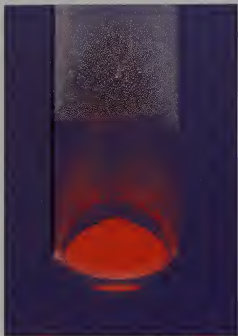
Figure 2-19 When mercury(II) oxide is heated, it decomposes into elemental mercury and oxygen gas. The red compound shown here is mercury(II) oxide. The elemental liquid mercury has condensed on the walls of the test tube.
