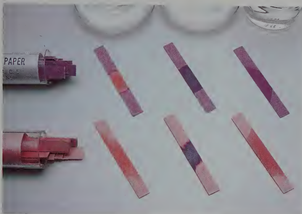
Figure 2-25 Litmus paper is used as a simple test for acidity or basicity. Blue litmus paper turns red when placed in an acidic solution. Red litmus paper turns blue when placed in a basic solution. In the upper row of strips, blue litmus paper is treated first with acid, then with base, and then with pure water. In the lower row of strips, red litmus paper is treated first with acid, then with base, and then with pure water.
