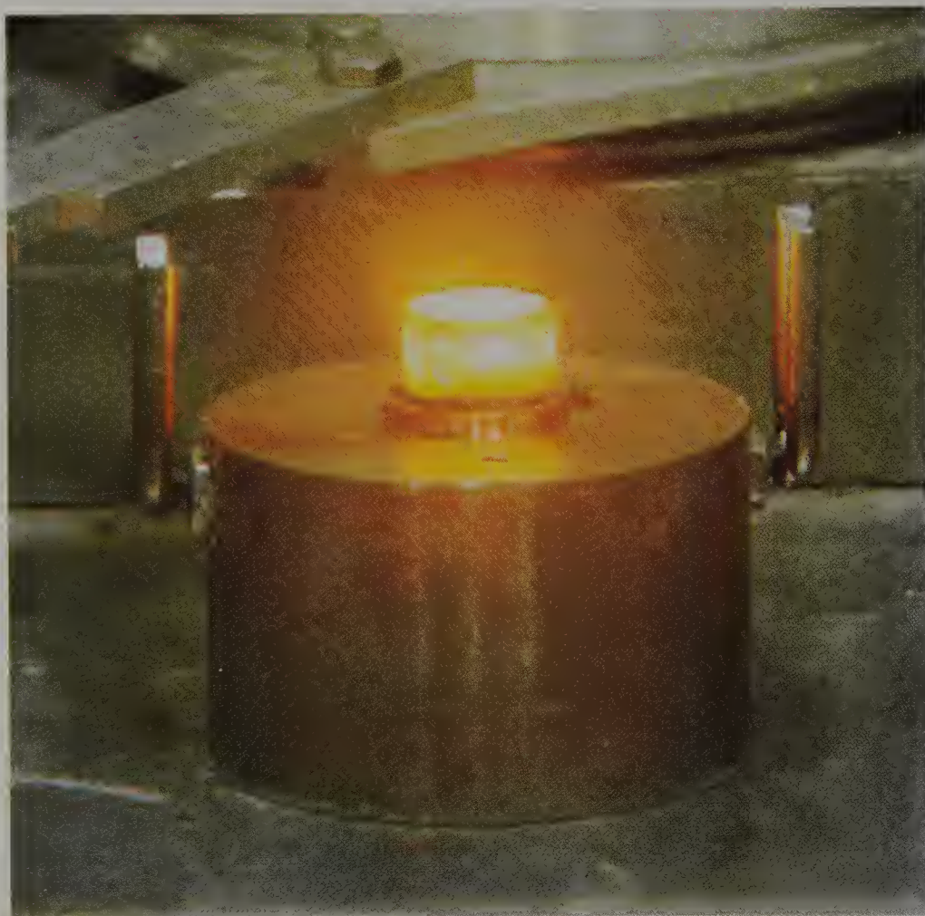
A sample of the radioactive substance, curium oxide, glowing from the heat released during radioactive decay.
