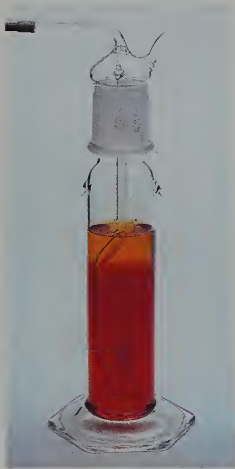
Figure 2-23 When \text{Cl}_2(g) is bubbled into an aqueous NaBr solution, the chlorine replaces the bromine in NaBr, forming \text{NaCl}(aq) and reddish \text{Br}_2(aq) .
