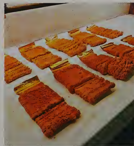
Figure 20-6 Gold is purified by electroplating. The spongy gold deposits shown here were electroplated onto gold strips. The top of the original gold cathode is visible in the photo.
