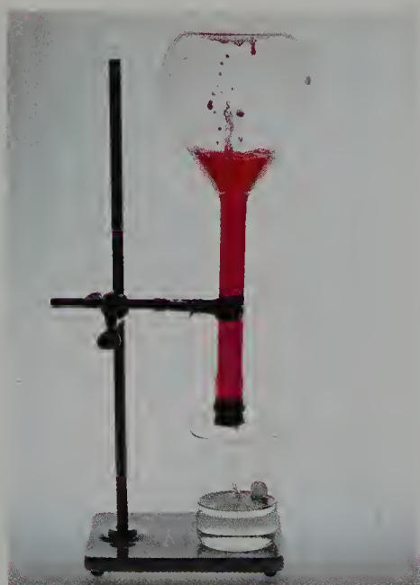
Figure I-2 An ammonia fountain. The inverted flask is filled initially with ammonia gas. The beaker contains water and the acid-base indicator phenolphthalein, which is colorless in acidic or neutral solution and red in basic solution. When a small amount of water is squirted into the flask, the dissolution of ammonia gas in water creates a pressure drop in the inverted flask, and the aqueous solution is driven up into the flask by the atmospheric pressure. The solution changes to a red color because ammonia is a base and phenolphthalein is red in basic solution. The high solubility of ammonia in water leads to a large pressure drop, which in turn produces a strong upsurge of solution, thus creating a fountain.
