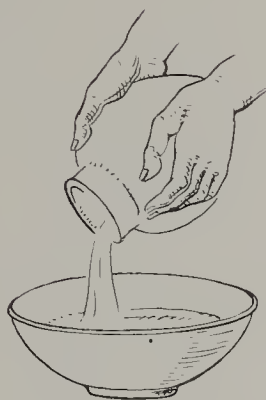
Fig. 64. Glazing the inside of a pot by swilling.
