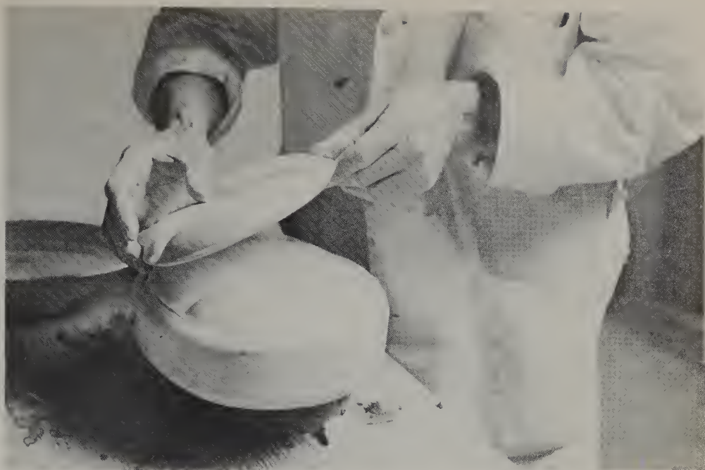
IX. Making a presed divided dish: Lifting the finished and dried dish off the mould
