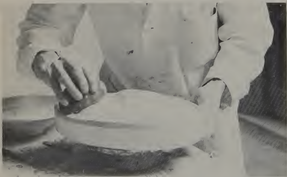
VIII. Making a pressed divided dish: Trimming and smoothing the back of the dish with a potter's kidney-shaped rubber
