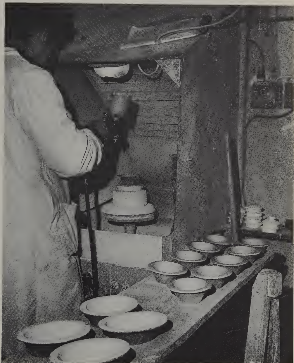
XXXVI. Glaze and colour spraying. Honiton Pottery
