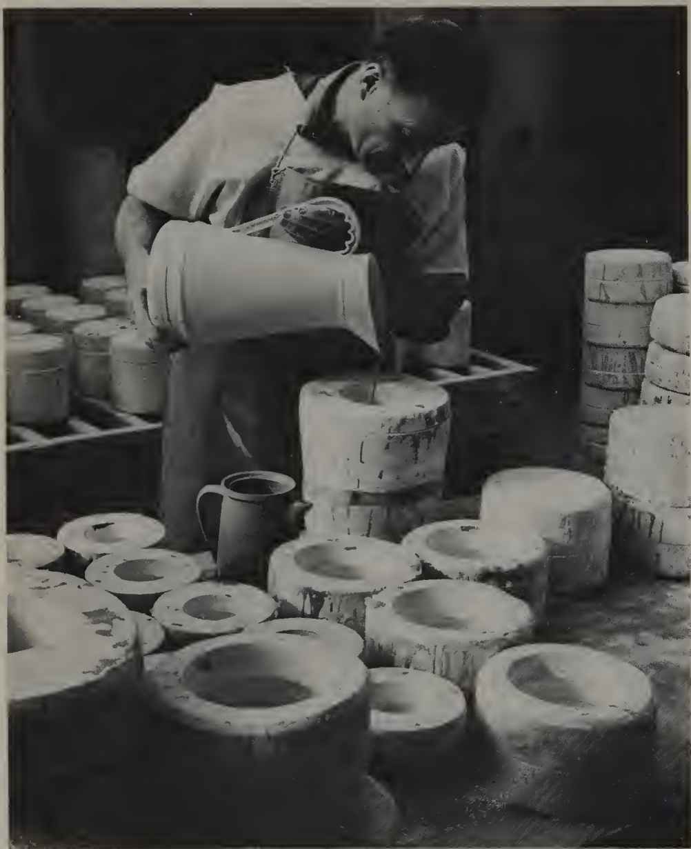
XXVIII. Casting: pouring slip (liquid clay) into a plaster mould. Honiton Pottery
