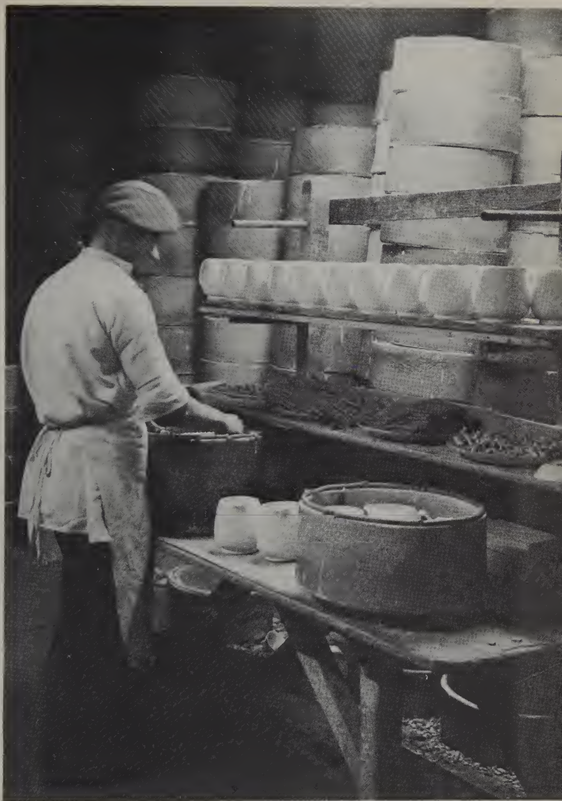
XXXIV. Placing glazed wares into saggars preparatory to firing
