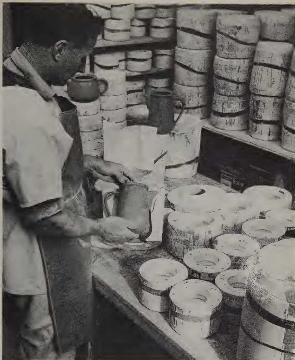
XXIX. Casting: after the cast has set and been drained, it is removed from the mould. Honiton Pottery
