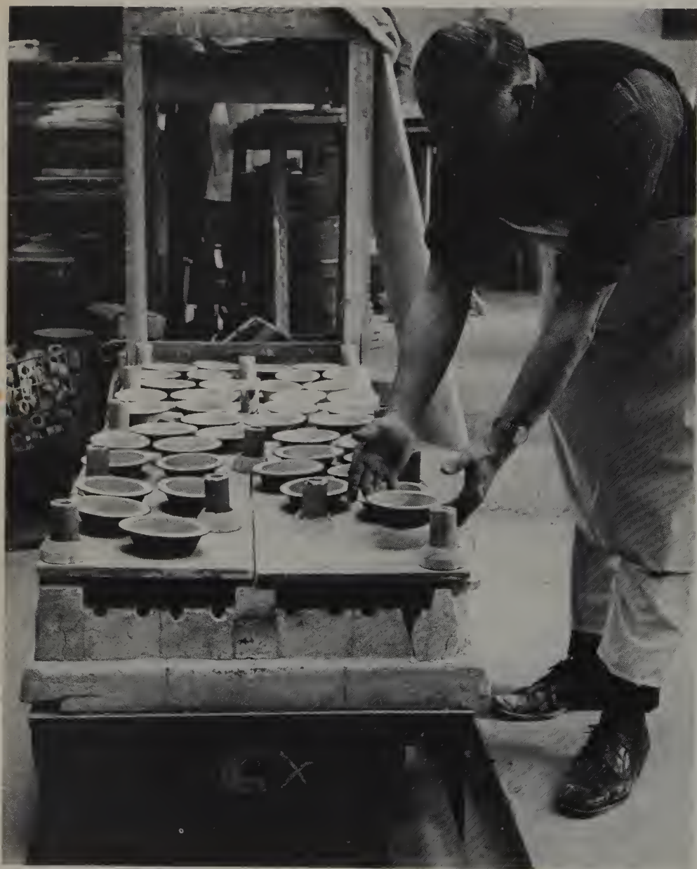
XXXI. Placing wares on a truck for a truck-loaded kiln. Honiton Pottery
