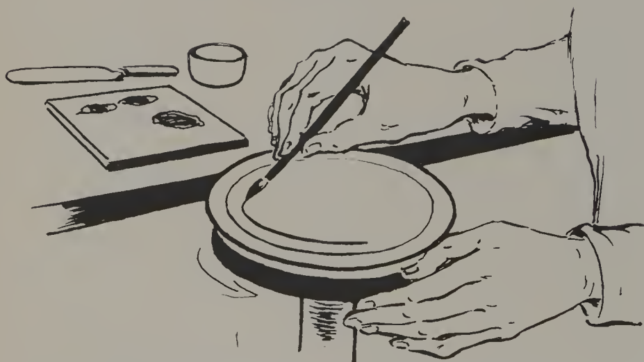
Fig. 61. Running bands and lines on a plate with the aid of the lining wheel.
