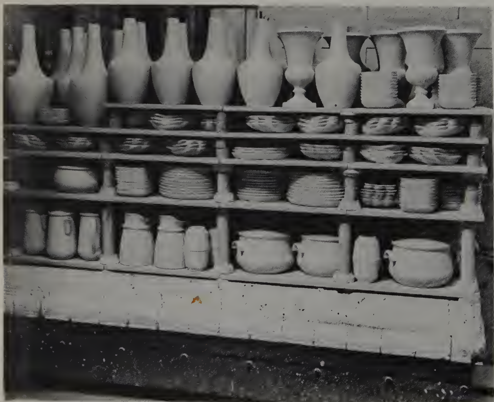
XXXIII. A truck inside the kiln ready to be fired. Honiton Pottery
