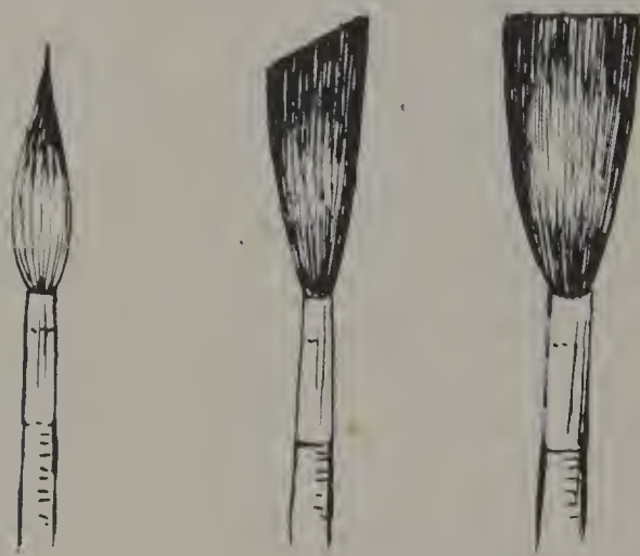
Fig. 60. A pottery painter's brushes. (a) Tracer (b) Liner (c) Bander
