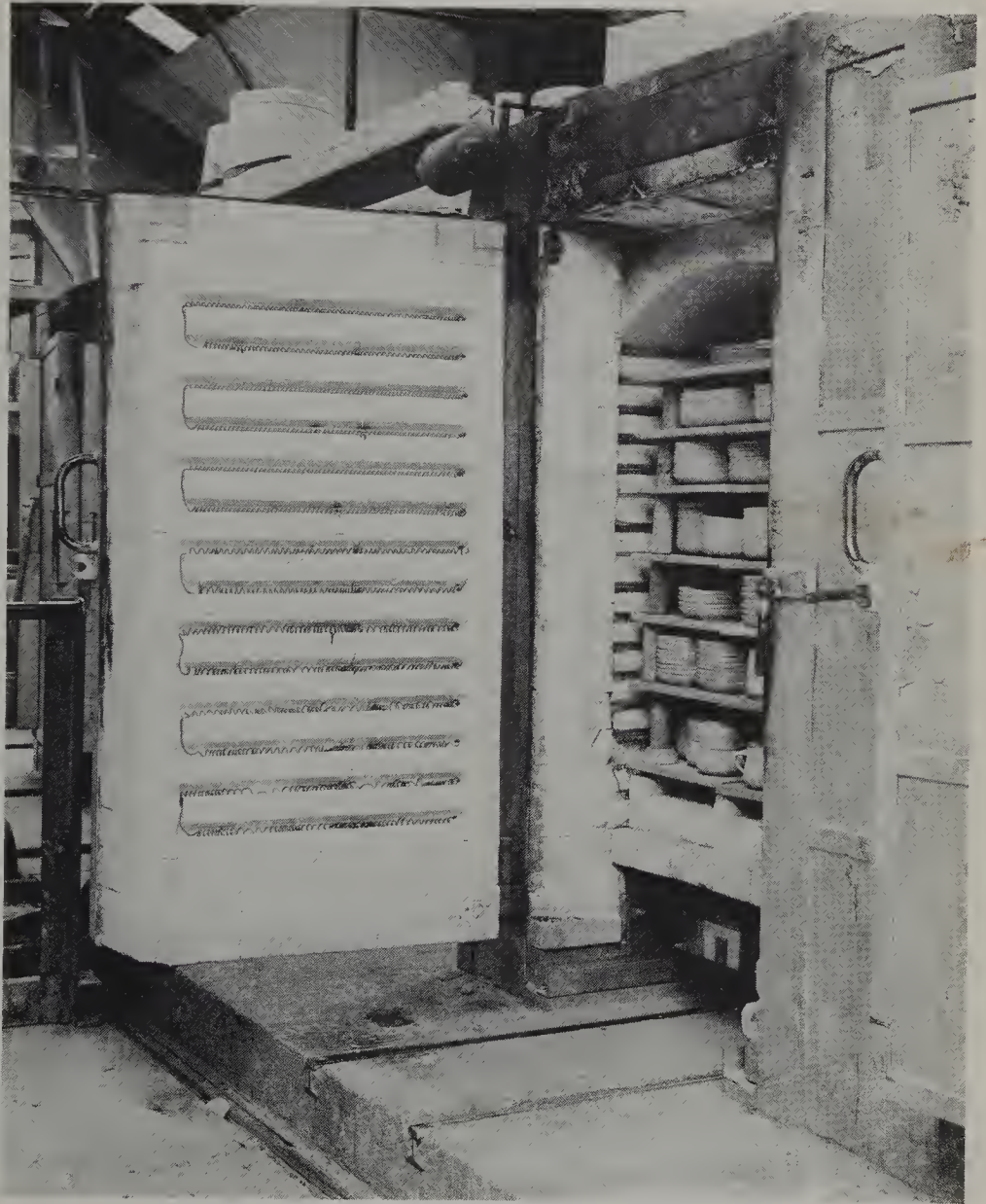
XXXII. A fully-loaded truck ready for firing. Honiton Pottery
