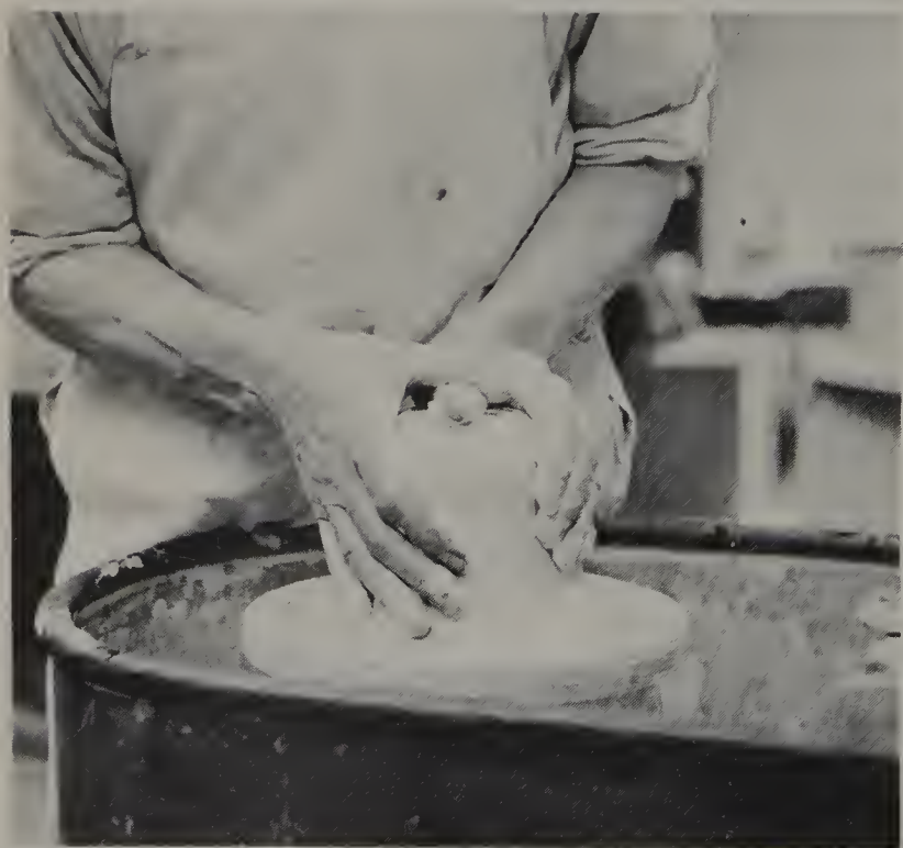
Depressing the clay cone into a cylindrical shape X-XI. Throwing
