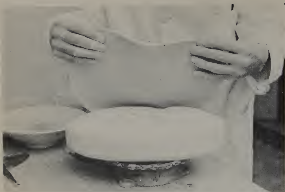
VII. Making a pressed divided dish: Putting the pancake of clay on to the mould
