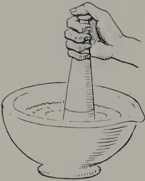
Fig. 69. Mixing and grinding glaze with a pestle and mortar.
