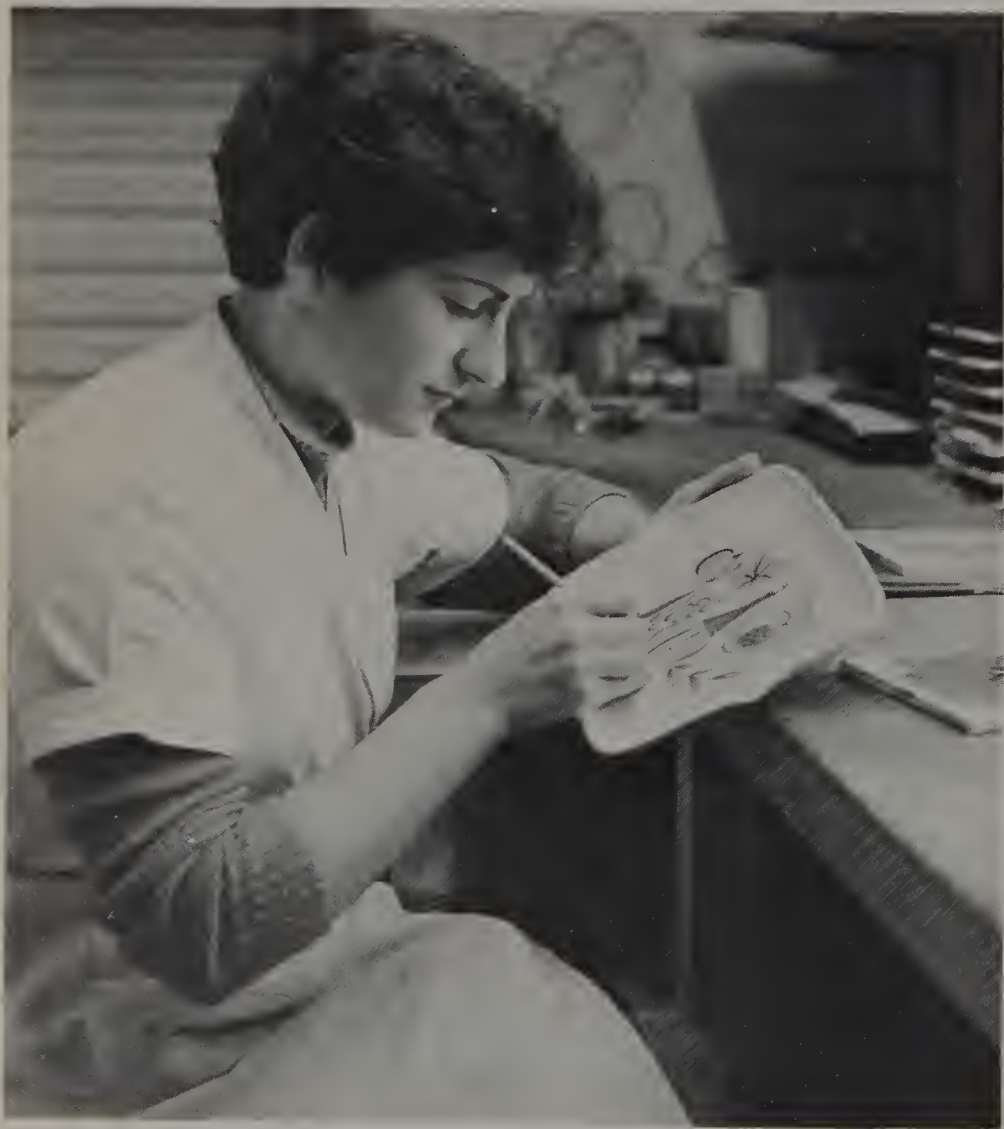
XXXVII. Hand painting on the biscuit ware in underglaze colours. Sandgate Pottery
