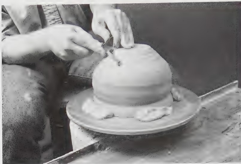
7-32 Trimming pottery on the wheel. The clay is shaved away a little at a time using a loop tool. Hold the tool firmly at about a 45-degree angle to the clay surface so that the tool peels off a continuous strip of clay as the pot turns. Start trimming using a small diameter loop tool or the small corner of a large trimming tool, taking little cuts until the surface is leveled. Then use the broader edge of the tool if a smooth surface is desired. Hold the pot down on the wheel head with the left hand. Brace yourself for stability just as when throwing.
