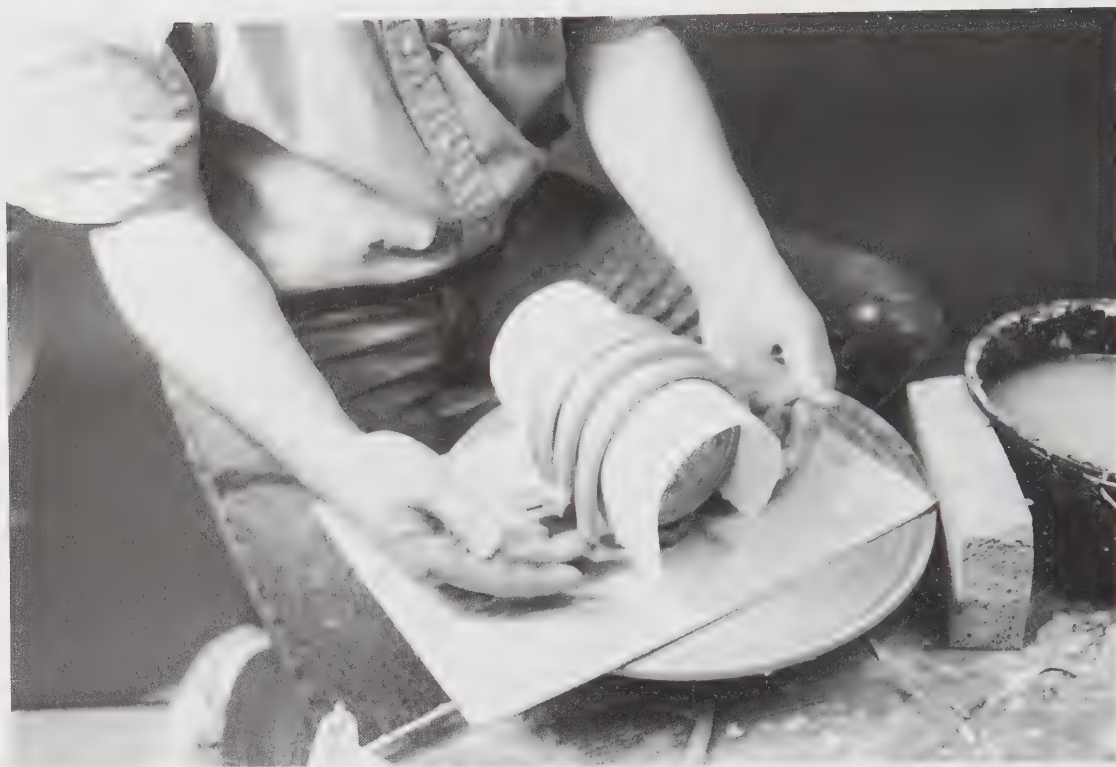
7-45 Shaping teapot handles Teapot handles can be shaped over a can or piece of pottery to get a uniform round curve. Note the piece of paper between the handles and the coffee can to keep them from sticking.
