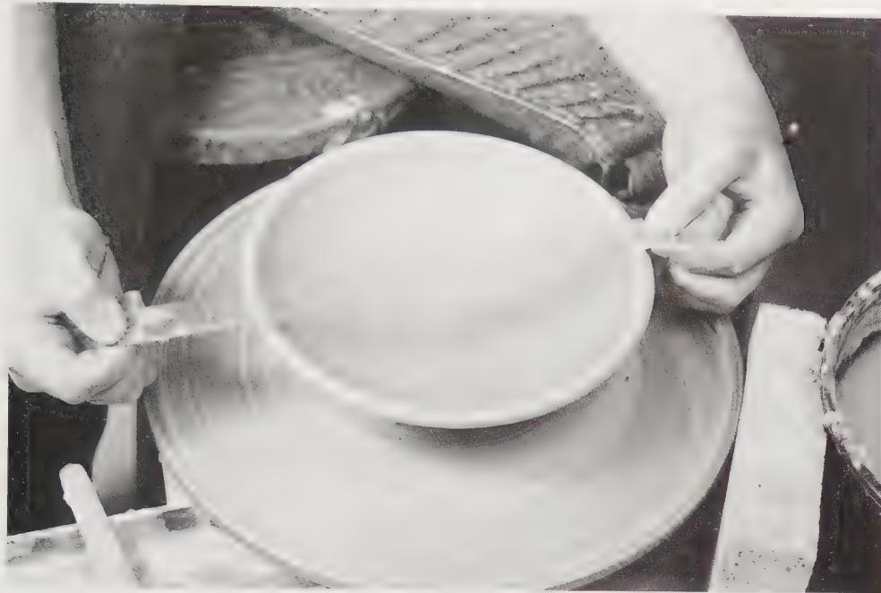
7-56 Making pots with lids Here the lid for the pot is being measured with a ruler. A simple bowl shape is made, which will be turned upside down and trimmed when it is leather hard. A knob or handle will be added after trimming to allow lifting the lid.
