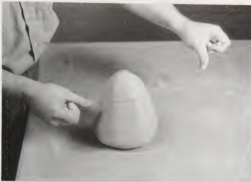
5-13 Wedging —spiral technique. The clay can be cut apart with a tightly stretched wire to check for air pockets or inconsistencies in the texture.
