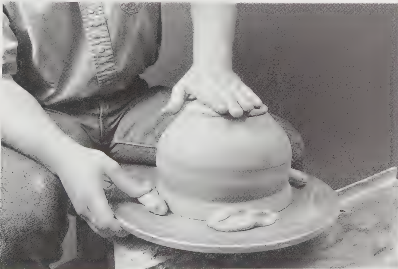
7-31 Trimming pottery on the wheel. Once the pot is centered on the wheel head, it must be firmly held in place during trimming. Thick coils of soft plastic clay are added as chunks to hold the bowl. Hold the pot down against the wheel to keep it on center, place a coil of clay against the rim, and then press the coil down against the wheel head to stick it. Don't press the plastic clay hard against the rim or it may distort the rim.
