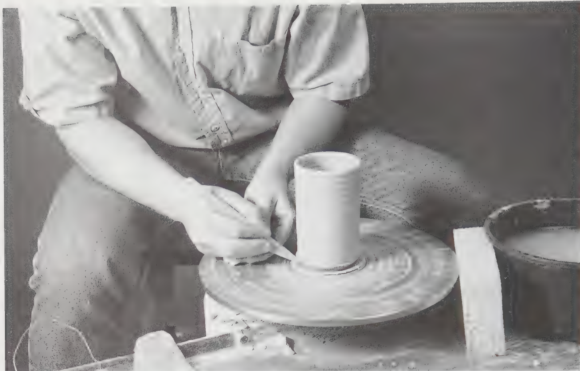
7-10 Basic throwing techniques—finishing. When the clay is evenly thinned to about 1/8- to 1/4-inch thickness and the cylinder is complete, trim off the extra clay at the base using a wooden potter's knife. Place the point against the clay about 1/4 inch above the wheel head, then slowly press the point downward at about a 45-degree angle until it hits the wheel head.
