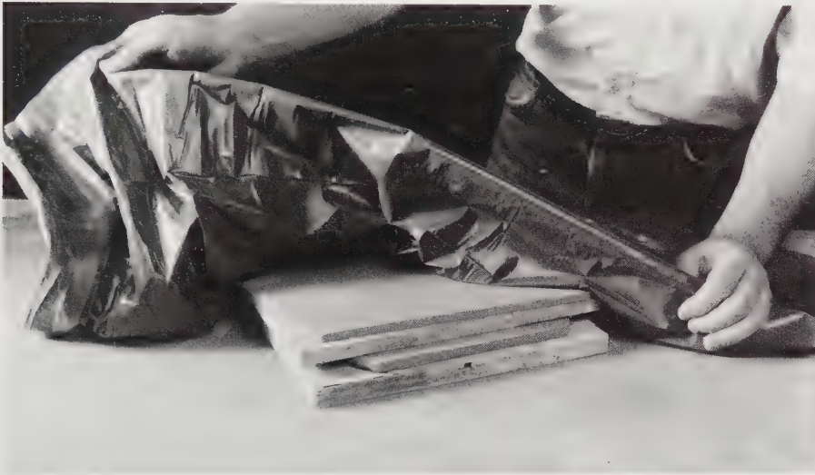
6-57 Stiff slab construction Slabs of clay are rolled out to a uniform thickness and left slightly larger than needed. They can be dried evenly by placing them on flat boards, which are stacked up like a board-on-clay sandwich, and covered with plastic for a day or so.
