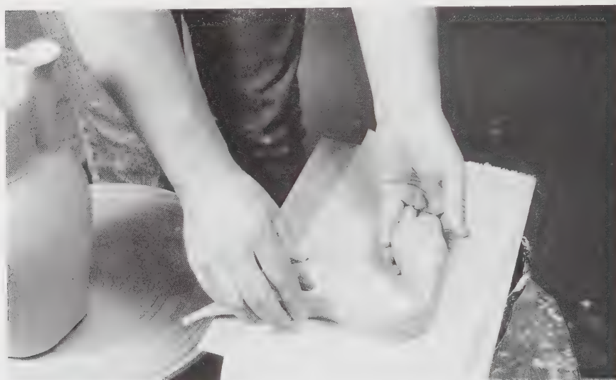
7-40 Pulling a handle After the handle is pulled it may be useful to let it dry slightly. You can lay the handle on its side on a clean piece of paper, shaping it fairly closely to the needed shape. After the clay stiffens a bit it may be impossible to make the sharp bends needed in the handle without it cracking. Cut off the large chunk of clay from which the handle was pulled, but leave some extra clay on both ends of the handle so that it can be cut and fitted to the pot.
