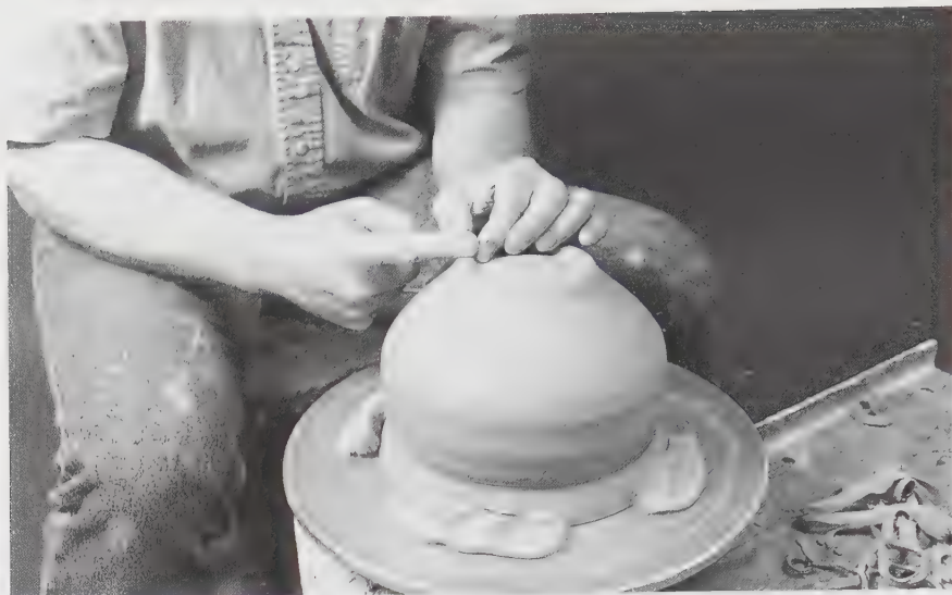
7-36 Trimming pottery on the wheel. The foot of the pot can be rounded and smoothed after trimming by pressing the side of the finger firmly against the clay. Use a very small amount of water if needed to help smooth the foot. A rib can be used if the clay is too dry or too groggy.
