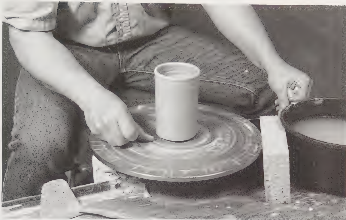
7-12 Basic throwing techniques—cutting off. The cut-off wire is stretched tightly between the hands and held against the wheel head with the right thumb. Pull the wire under the pot as it turns slowly, taking care that the wire stays tightly against the wheel head. You can squeeze a little water from your sponge onto the wheel head and into the groove at the base of the pot before cutting. This helps to easily slide the pot off the wheel.
