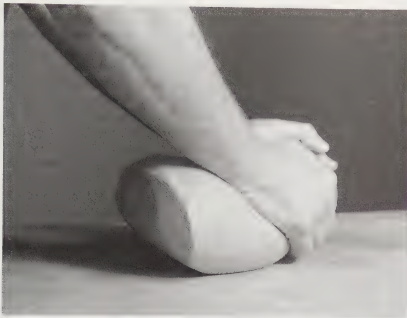
5-9 Wedging —spiral technique. As the clay is pressed down, allow it to roll forward on the table so that the bottom part of the clay (at left) rocks up slightly.
