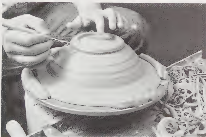
7-35 Trimming pottery on the wheel. Judging the thickness of the bottom when trimming takes some practice. Some potters tap on the bottom to hear the change in sound as the bottom gets thinner and more drum-like. Taking a careful look at the shape of the inside of the pot before trimming is equally important!
