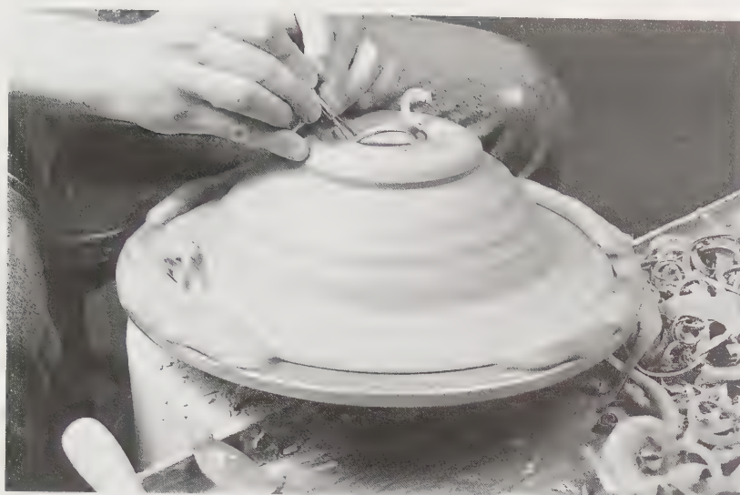
7-34 Trimming pottery on the wheel. Make the foot robust enough to hold the weight of the pot. A well-designed foot can elevate and accentuate the pot, or be a subtle underpinning to the form.
