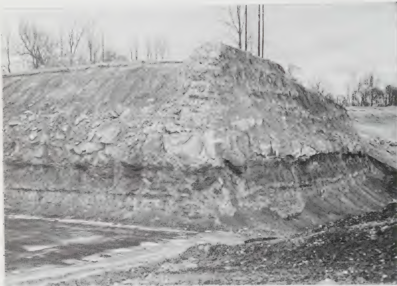
1-5 Clay mining in Oak Hill, Ohio. Clay is mined here at Cedar Heights Clays using heavy industrial equipment. Stoneware clays in the midwestern U.S. often are found in thick layers like this. Before the clay can be used it must be ground and processed.
