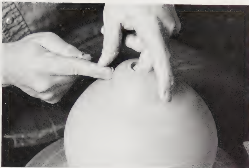
7-23 Throwing closed forms More clay is brought up toward the top as the clay is pushed down and in, supported carefully inside throughout the process. Note how the thumb of the left hand helps to steady the forefinger of the right hand which is doing most of the work.
