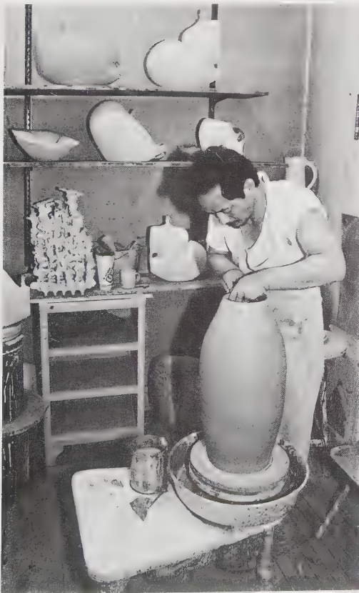
7-21 Yoshiro Ikeda, USA. The top of a larger bottle form is closed slowly, as the potter demonstrates here. Ikeda keeps the main surface of the pot fairly dry when throwing this large form. Water is applied only to the upper section where he is working. This helps to keep the clay from becoming overly soft and prevents the collapse of the large pot.
