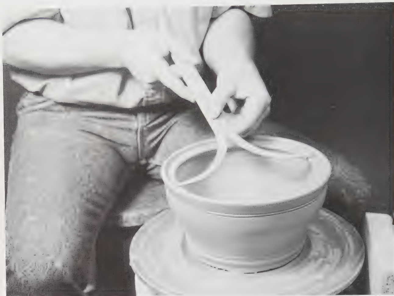
7-55 Making pots with lids Calipers are useful for accurately measuring the widest part of the lid opening. A ruler could also be used if care is taken to measure accurately right after throwing the form.
