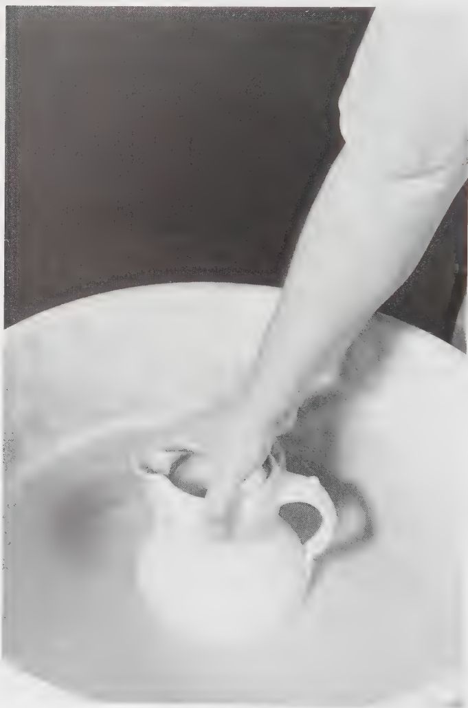
8-23 Glazing by dipping Dipping pots into a glaze is a quick way to apply glaze evenly.
