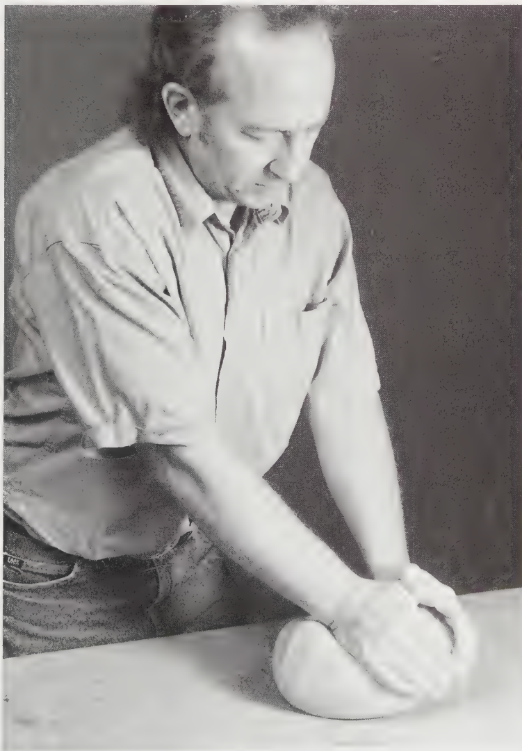
5-6 Wedging and wedging table. The wedging process involves repeated kneading of the clay to remove lumps and air pockets. The wedging table should be low enough to use the full weight of the upper body to help move the clay.
