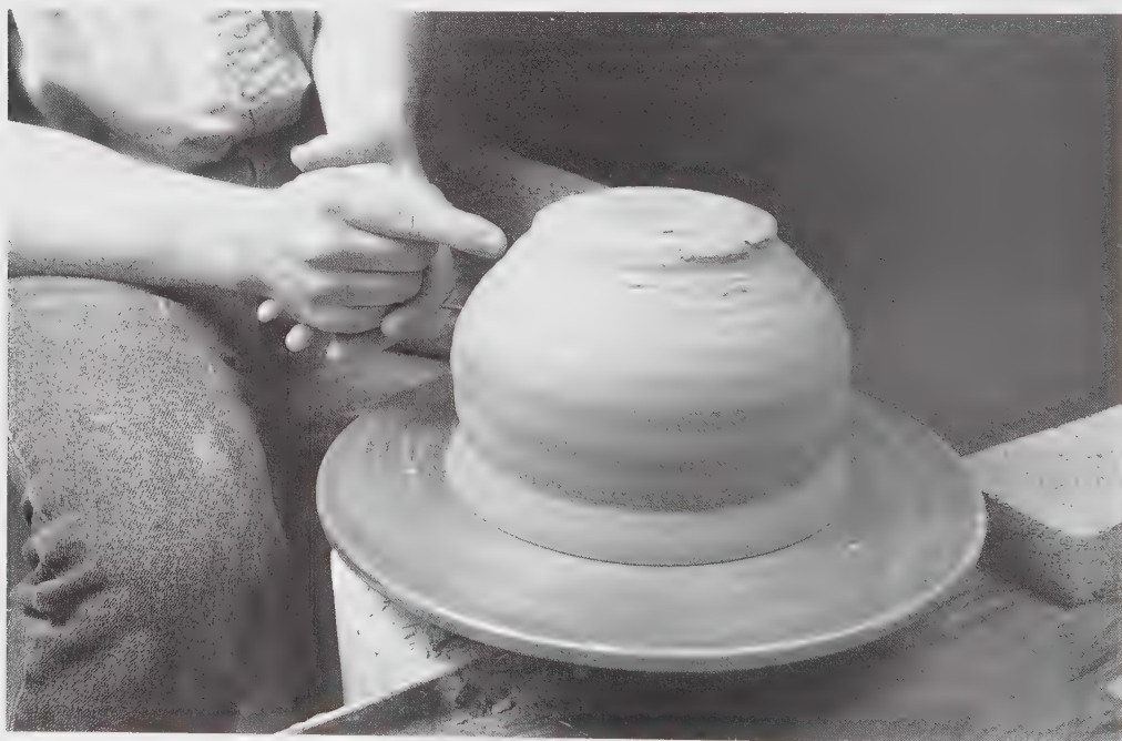
7-29 Trimming pottery on the wheel. Trimming or tooling first requires that the potter re-center the upside-down leather-hard pot on the wheel. This can be done by starting the wheel, holding a finger or tool steady to see where the pot is most off center, and stopping the wheel to move the pot sideways slightly in the direction indicated.
