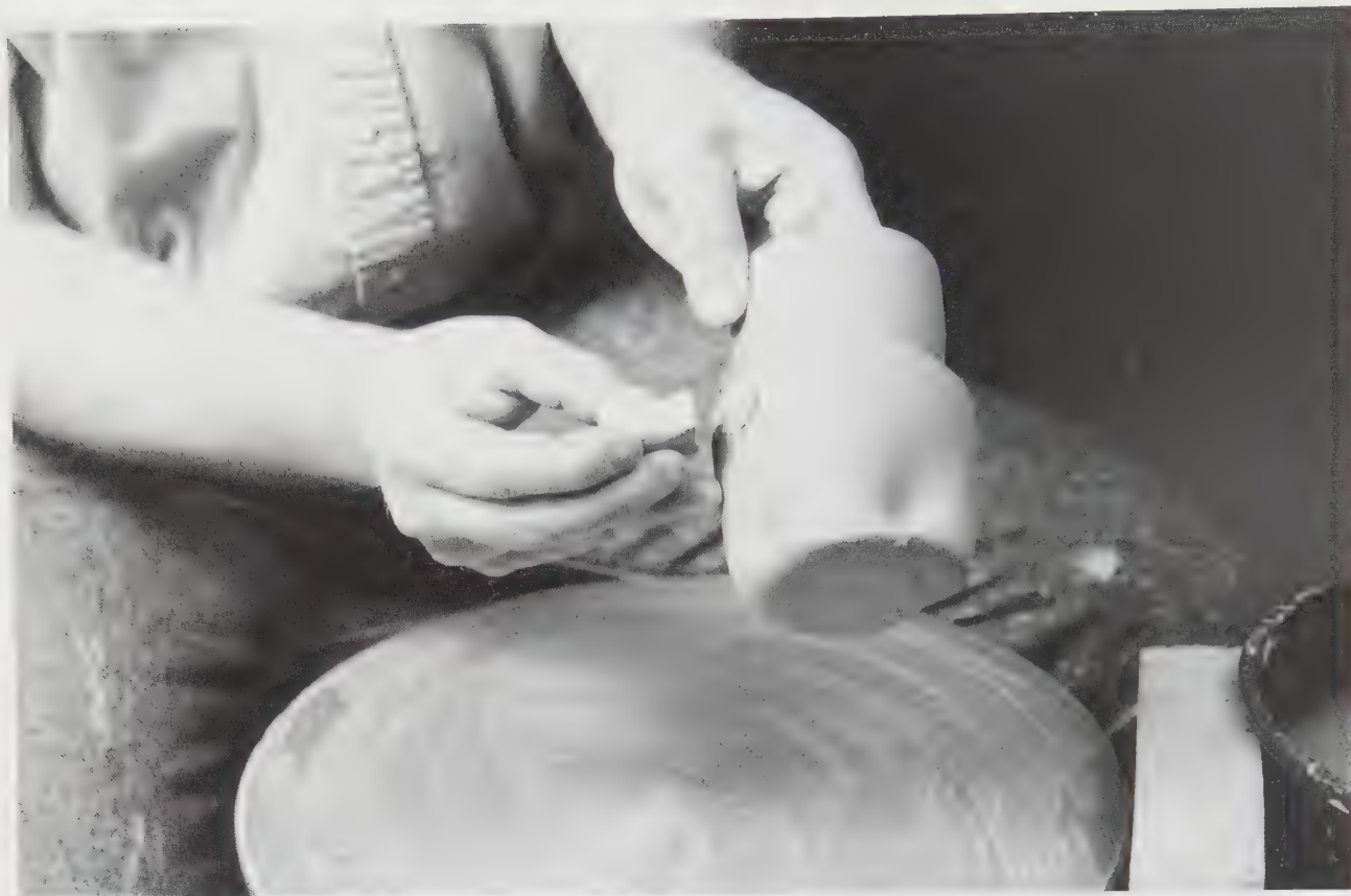
8-6 Sprigging A sprigged design is added to this cup. A small amount of plastic clay is first pressed into the design which has been carved into the end of a bisque clay stamp. This is then pressed onto the surface of the damp clay pot, transferring the design as a raised image.
