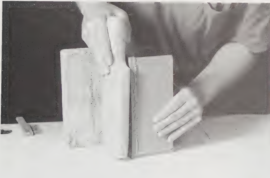
6-62 Use a wooden paddle to put even pressure on the joint and still keep it flat.
