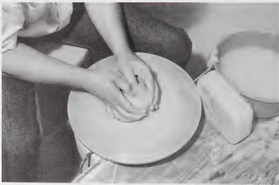
7-4 Basic throwing techniques—centering. When the clay is centered, use the thumbs together to find the exact center of the clay. Keep the hands loosely around the sides of the clay to help steady yourself. Note that the arms are still in the triangular shape, well braced against the body. The thumbs can continue pressing down together, with lots of water for lubrication, stopping about 3/8 inch from the wheel head. It's important to keep the thumbs together, gradually turning them nail to nail, so that they can follow the path of least resistance down the center of the spinning clay.
