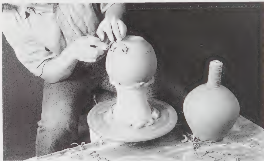
7-37 Trimming using a chuck A bisque-fired clay chuck (the cooling tower shape under this long-necked round bottle being trimmed) is useful for trimming shapes that otherwise would be impossible to turn upside down on the wheel for trimming. A number of variations in shapes and sizes of chucks can be quickly thrown on the wheel. Make the chucks thick and sturdy enough to withstand repeated use. Clay chucks like this can be used as leather-hard clay or even when dry, but are stronger when bisque fired.
