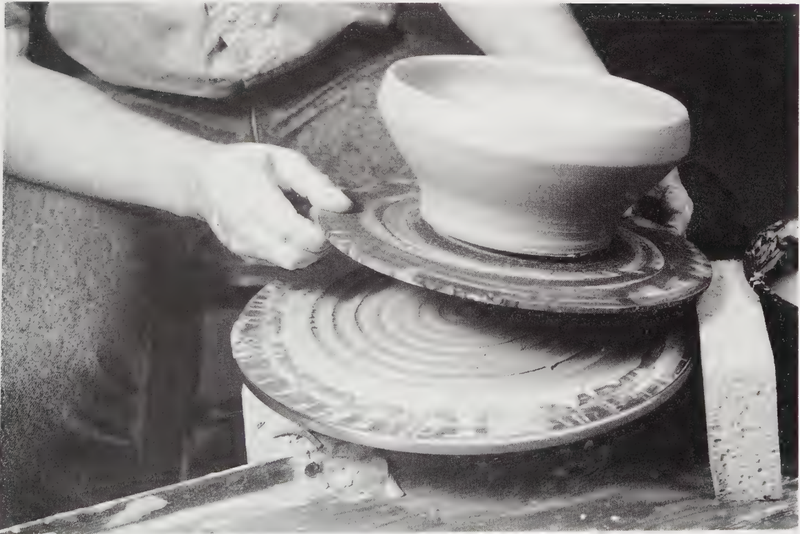
7-19 Using a bat on the wheel makes it easy to remove shapes like bowls, which distort easily if lifted with only the hands.
