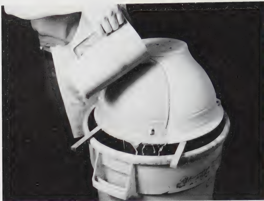
8-25 Glazing a large pot Pouring is a good way to glaze the interior of pots and the exterior of large and awkward shapes. Care and a large container are needed so as not to waste glaze. For the most even coating of glaze, use a large enough pouring container of glaze to cover the whole form in one continuous pour. Note the large bowl being supported by two wood slats while glazing. These will leave very small unglazed spots on the rim which are easily touched up with a brush.
